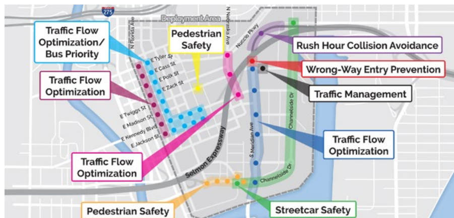
Figure 3.4 Connected Vehicle Pilot Deployment—Downtown Tampa
