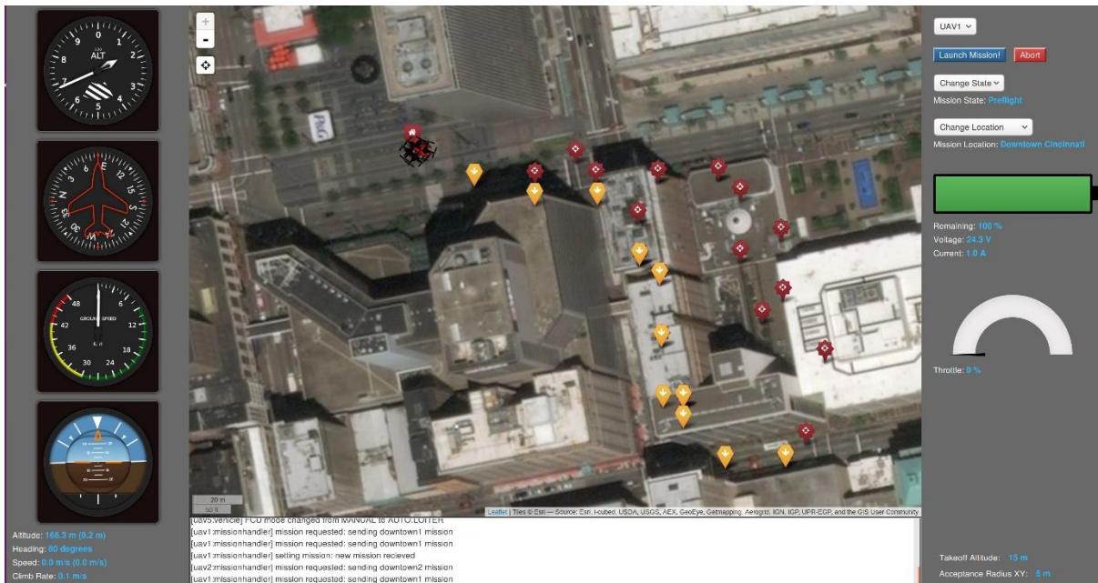
Figure 6: UC's Flymaster Ground Control Program with auto-generated waypoints
