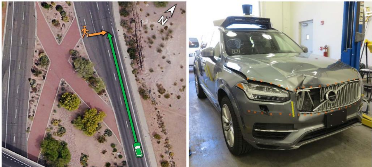
Figure 4-5 (Left) Location of the crash, showing the paths of the pedestrian and of the Uber test vehicle. (Right) Post-crash view of the Uber test vehicle, showing damage to the right front side (NTSB, 2018)
