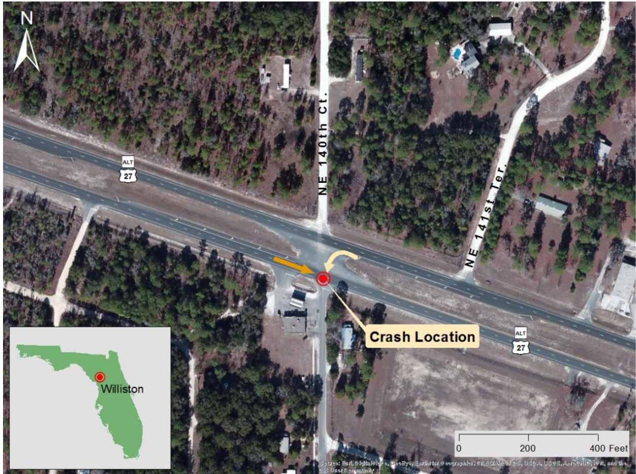
Figure 4-1 Overhead view of the crash intersection, showing the route of the eastbound car toward the crash location with a straight arrow, and the route of the left-turning truck, with a curved arrow (NTSB, 2017)
