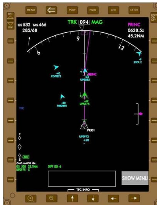
Figure 11. MITRE CDTI on an EFB incorporating the “picnic table” symbology for temporal spacing maintenance (from RTCA 2010, p. 209).
