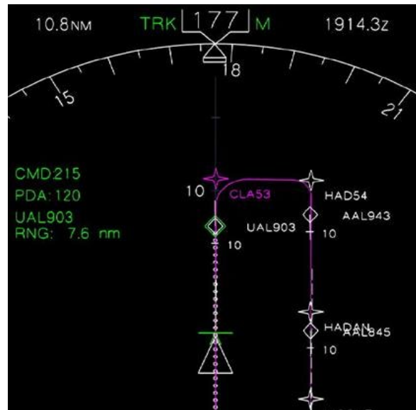
Figure 10. AMSTAR incorporating the “picnic table” symbology for temporal spacing maintenance (from Oseguera-Lohr et al., 2002, pgs. 4, 5).
