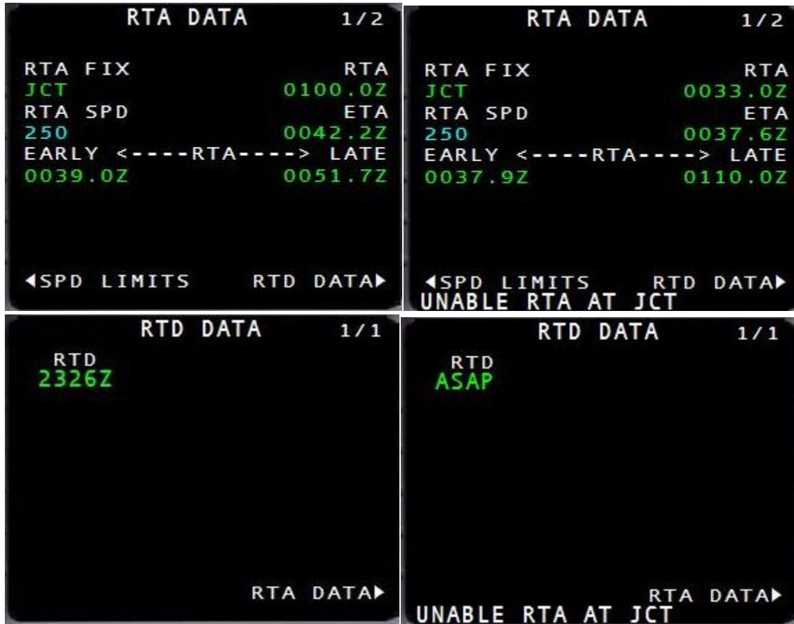
Figure 19. MCDU RTA pages – clockwise from top left: can make RTA, unable to make RTA, unable to make RTA – RTD ASAP, can make RTA with RTD.
