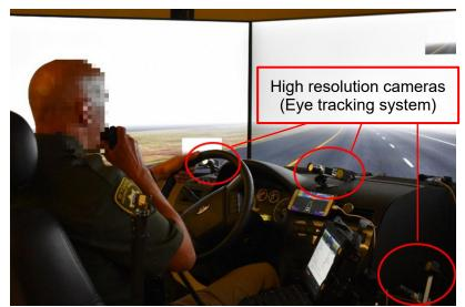
**Figure 50. Smart Eye Cameras Mounting Locations - HP.** *Source: WYDOT &* (23)
