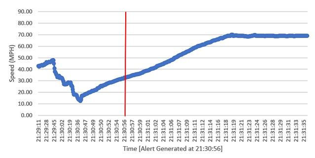
Figure 69. Case B.4 -- Speed (MPH) v. Time. Action: Vehicle Reduced Speed. Source: WYDOT
