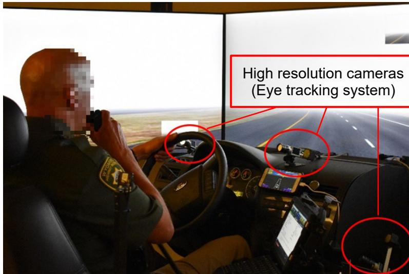
**Figure 50. Smart Eye Cameras Mounting Locations - HP.**
