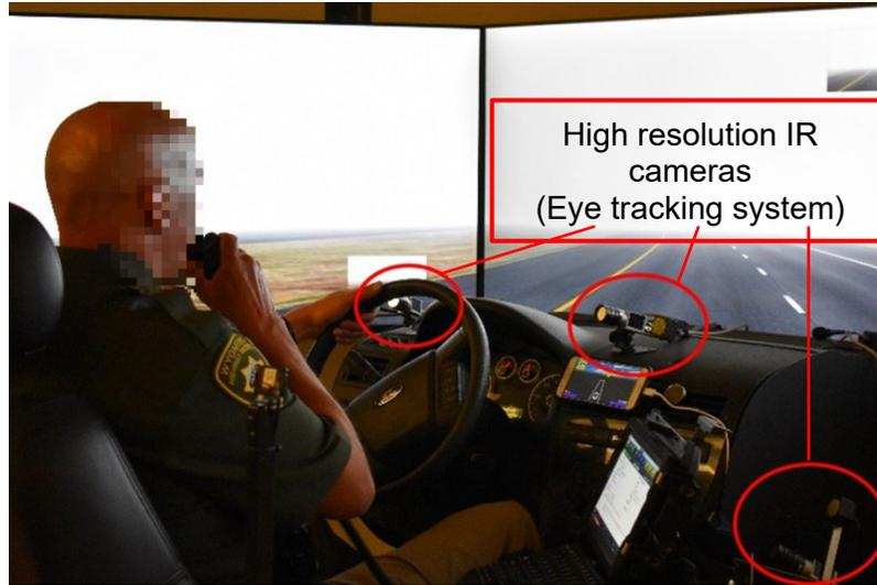
**Figure 157. Smart Eye Cameras Mounting Locations.**
