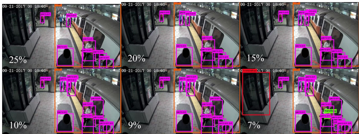
Figure 2.8: Passenger counts at various thresholds using YOLO
