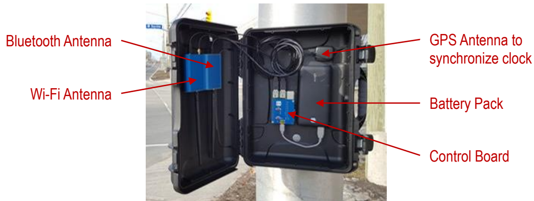
Figure 2.10: Components of the SMATS TrafficBox wireless device detector
