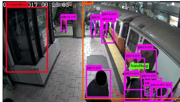
Figure 3.13: Example camera frame showing identified passengers at North Station
