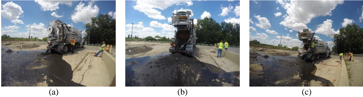
Figure B.41: BUCHER RECYcler 315 Operations on July 18, 2018 at Columbus Decanting Station (a) Draining tank of liquid waste, (b) Rear open dumping the solid waste, (c) Rinsing of all excess waste.
