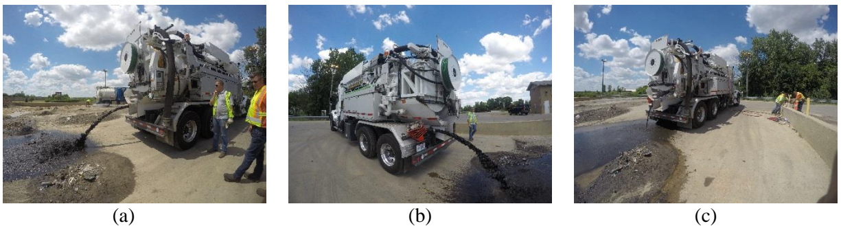
Figure B.40: BUCHER RECYcler 315 Operations on July 18, 2018 at Columbus Decanting Station (a, b) Disposing all the liquid waste, (c) Preparing fresh water hydrant for cleaning.
