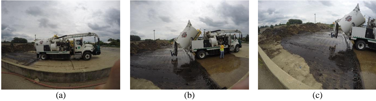
Figure B.9: VJT Operations Using Vac-Con 9CY on June 26, 2018 in Madison County (a) Truck prior to decant, (b) Decanting at Columbus WWTP, (c) Post Decanting.
