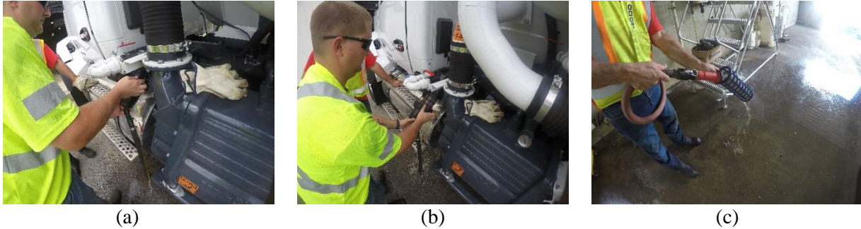
Figure B.33: BUCHER RECycler 315 Maintenance on July 16, 2018 at ODOT Westerville Outpost (a) Draining the tube filter, (b) Releasing the filter from the enclosure, (c) Cleaning filter.
