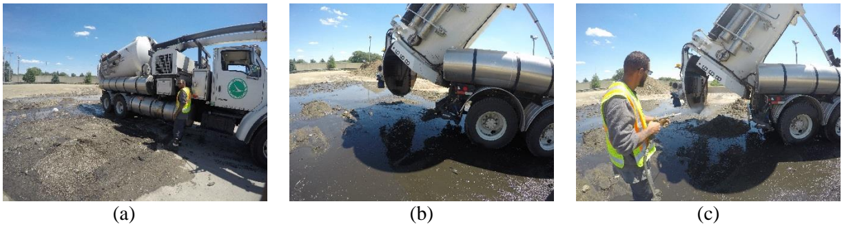
Figure B.38: VJT Operations Using Vector 2100 on July 17, 2018 at Columbus Decanting Station (a) Preparing to dispose of waste, (b) Tank raised disposing waste, (c) Hosing to clear of excess waste.
