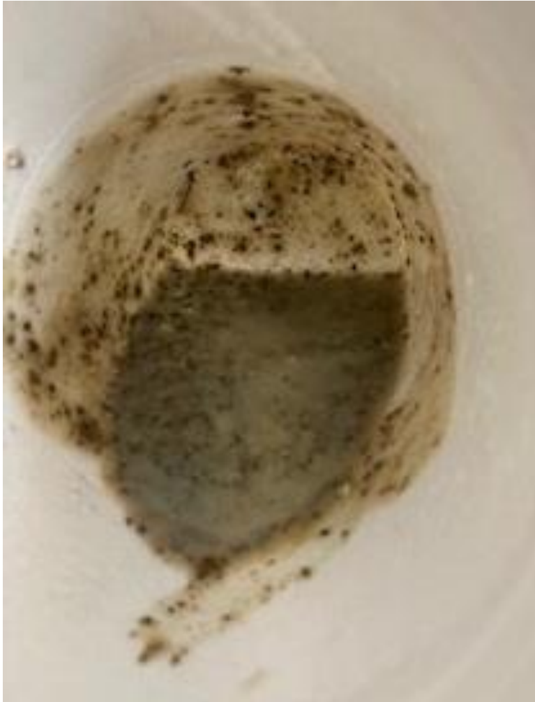
Figure 5. Photograph of “thick chunky material” that formed during application. D. Walker, CDOT
