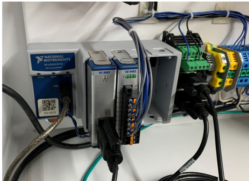
Figure 14. CUI chassis and modules
