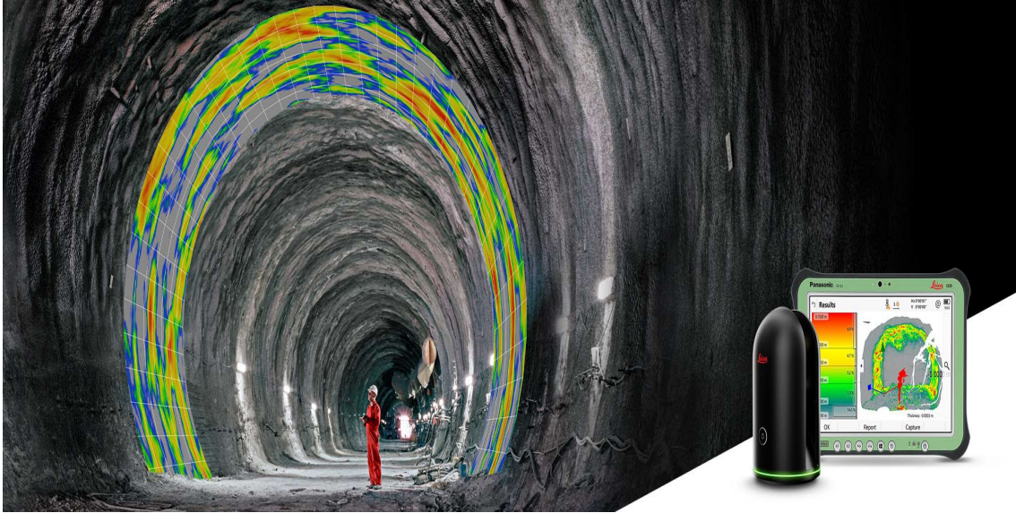
Figure 2.3 3D modeling of constructed structures
