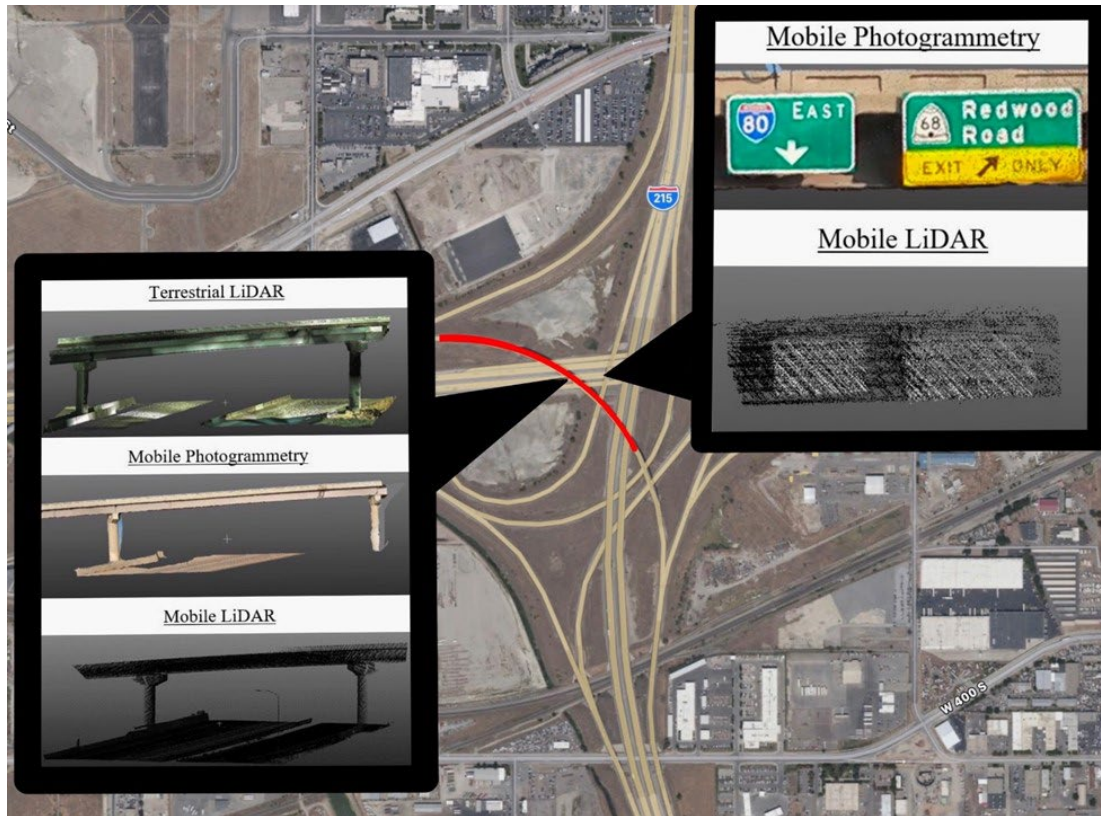
Figure 5.10 Map of reconstructed highway sections (showing the bridge model and a traffic sign model). Images are from both LiDAR-based highway models and image-based highway models.
