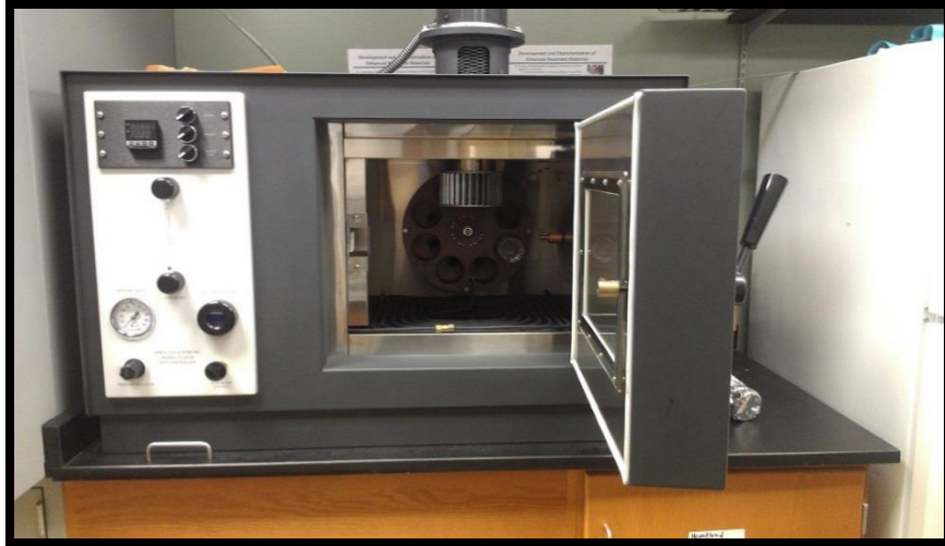
Figure 15. A Rolling Thin-Film Oven (RTFO) from James Cox and Sons
