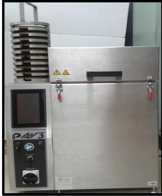
Figure 16. A Pressure Aging Vessel (PAV) from ATS
