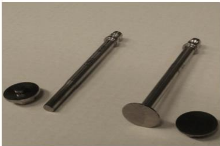
Figure 18. A DSR Machine with Bottom and Upper Plate.
