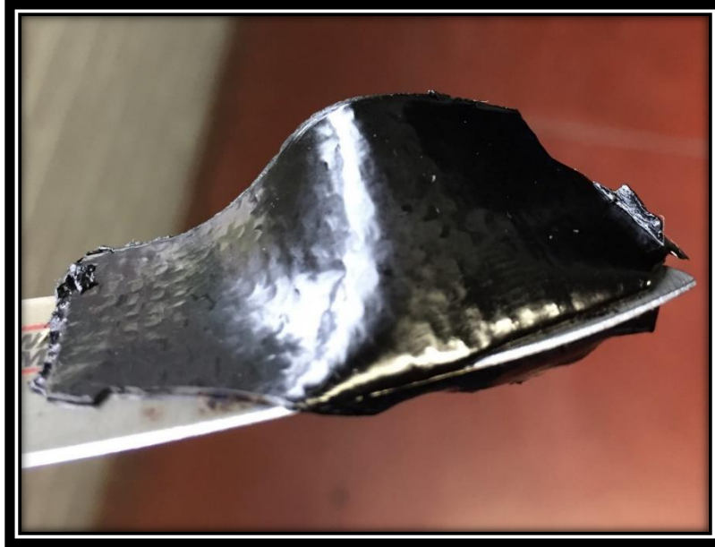
Figure 134. Sticking to the metal edge due to a short cooling period
