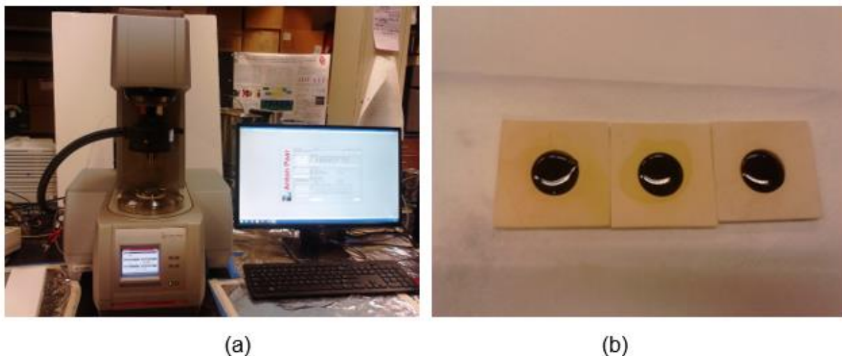
Figure 63. Test setup for DSR test on asphalt binder samples: (a) DSR apparatus; (b) asphalt binder samples for DSR test
