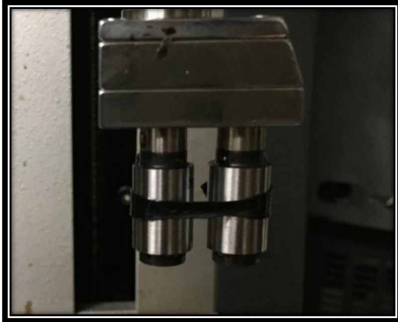
Figure 148. Sample during the extensional deformation test
