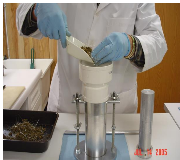
Figure 43. Preparation for Compaction of Direct Shear Specimen (Gregory 2006)
