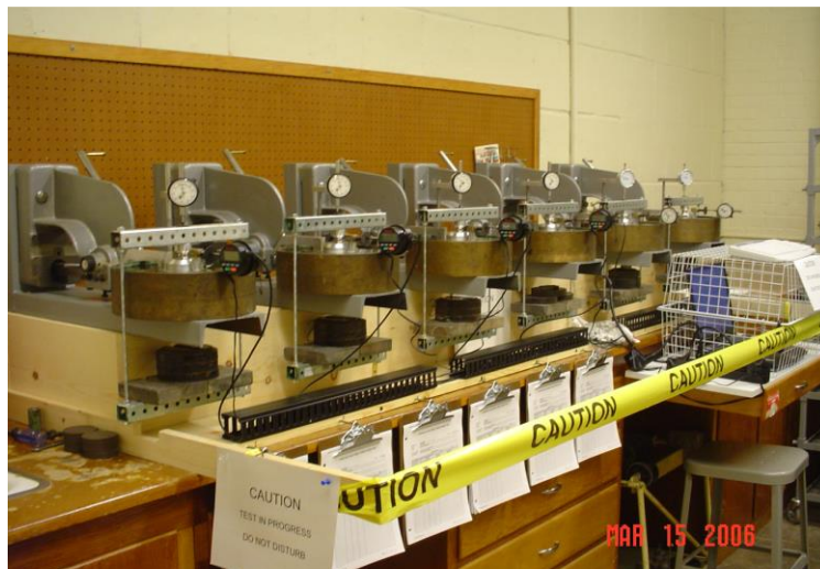
Figure 61. Direct Shear Creep Devices (Gregory 2006)
