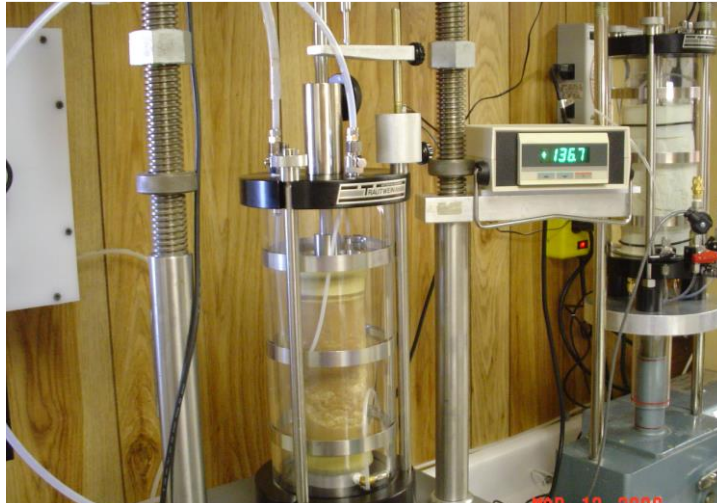
Figure 64. Triaxial Test on Sand Specimen (Gregory 2006)
