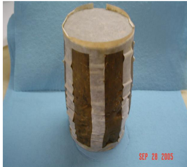
Figure 55. Clay Triaxial Specimen Following Test (Gregory 2006)
