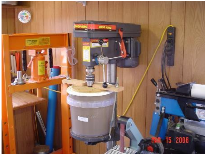
Figure 21. Mixer for Processing Fiber-Soil Specimen into Slurry (Gregory 2006)
