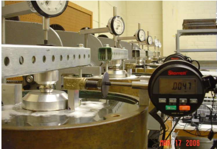
Figure 63. Fully Mounted Creep Specimens with Water in Reservoir (Gregory 2006)
