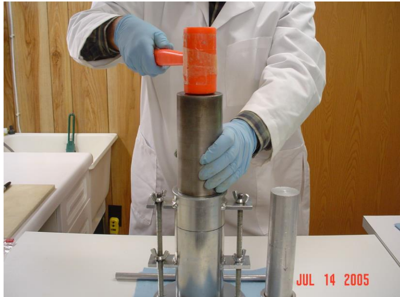
Figure 42. Finishing Compaction with Piston and Guide Ring (Gregory 2006)
