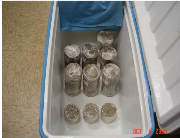
Figure 45. Clay Specimen Storage Cooler (Gregory 2006)
