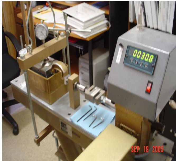
Figure 59. Computer Controlled Direct Shear Test Machine (Gregory 2006)
