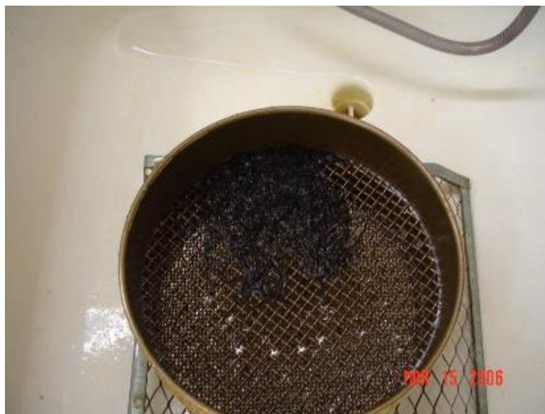
Figure 22. Sieving of Slurry to Extract Fibers (Gregory 2006)
