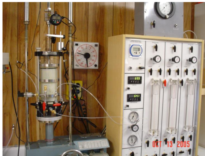
Figure 54. Shear Stage of Triaxial Test on Clay Specimen (Gregory 2006)
