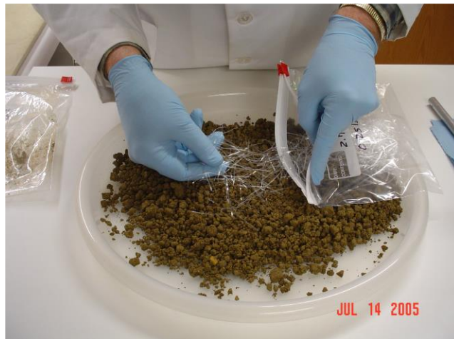
Figure 35. Spreading Fibers Over Hydrated Clay Soil Specimen (Gregory 2006)
