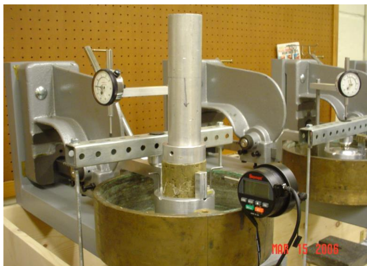
Figure 62. Mounting Clay Specimen in Creep Device (Gregory 2006)
