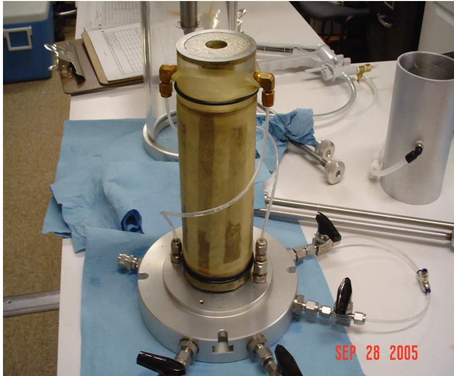
Figure 51. Specimen with Membrane and Top Cap in Place (Gregory 2006)
