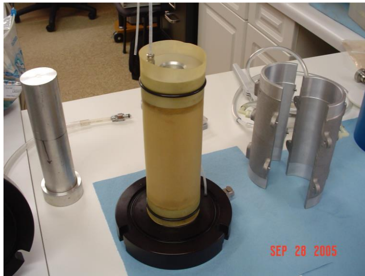
Figure 48. Compacted Sand Specimen after Removal of Split Mold (Gregory 2006)
