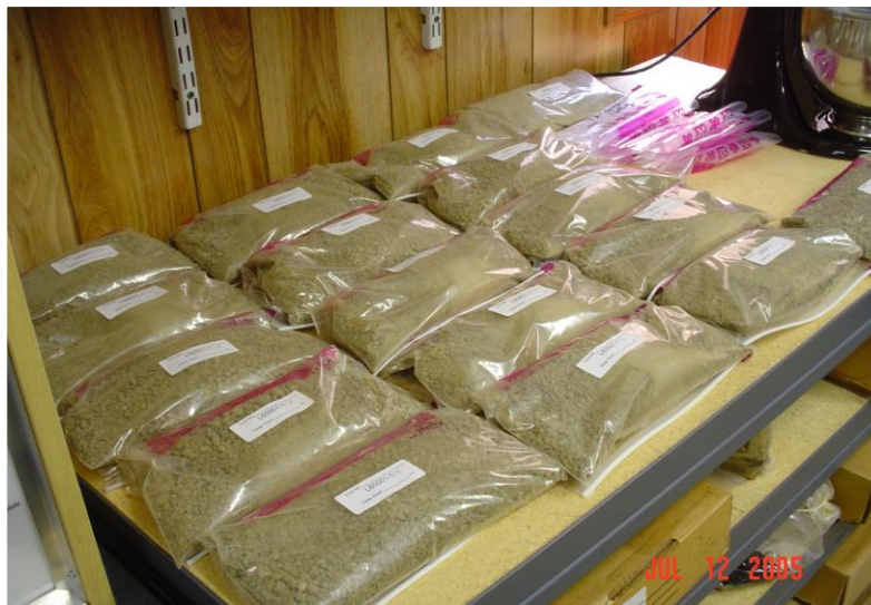
Figure 34. Clay Specimens Prior to Hydration (Gregory 2006)
