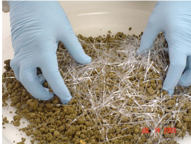
Figure 36. Initial Hand Mixing of FRS Specimen (Gregory 2006)
