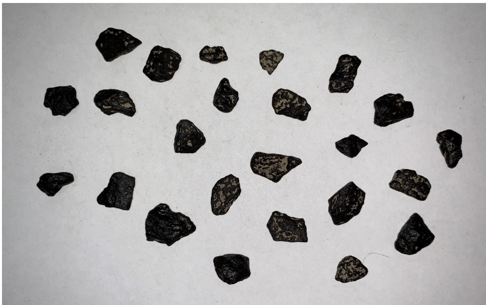
Figure 4.16. Sandstone aggregate at 85.3% precoat (0.6% binder by weight)
