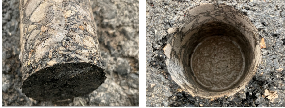
Figure 6.28. Waco SB widening- no treatment- no diamond grinding- hot applied trackless tack- 1st spot
