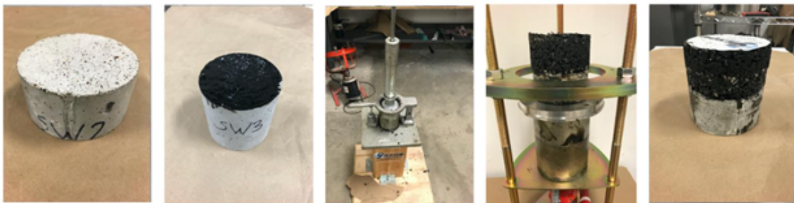
Figure 3.2. Specimen fabrication using the Marshall compactor
