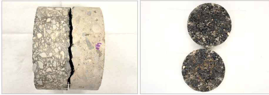
Figure 6.21. Side and top view from SAT I410 core after shear test
