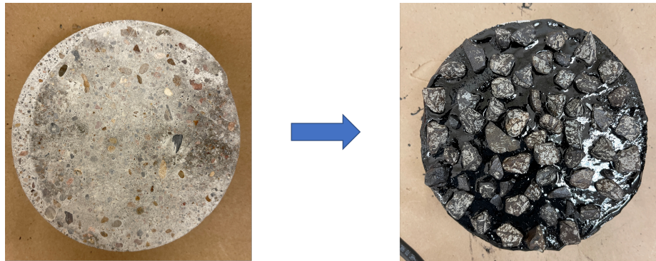
Figure 5.2. A PCC sample with AR binder as chip seal
