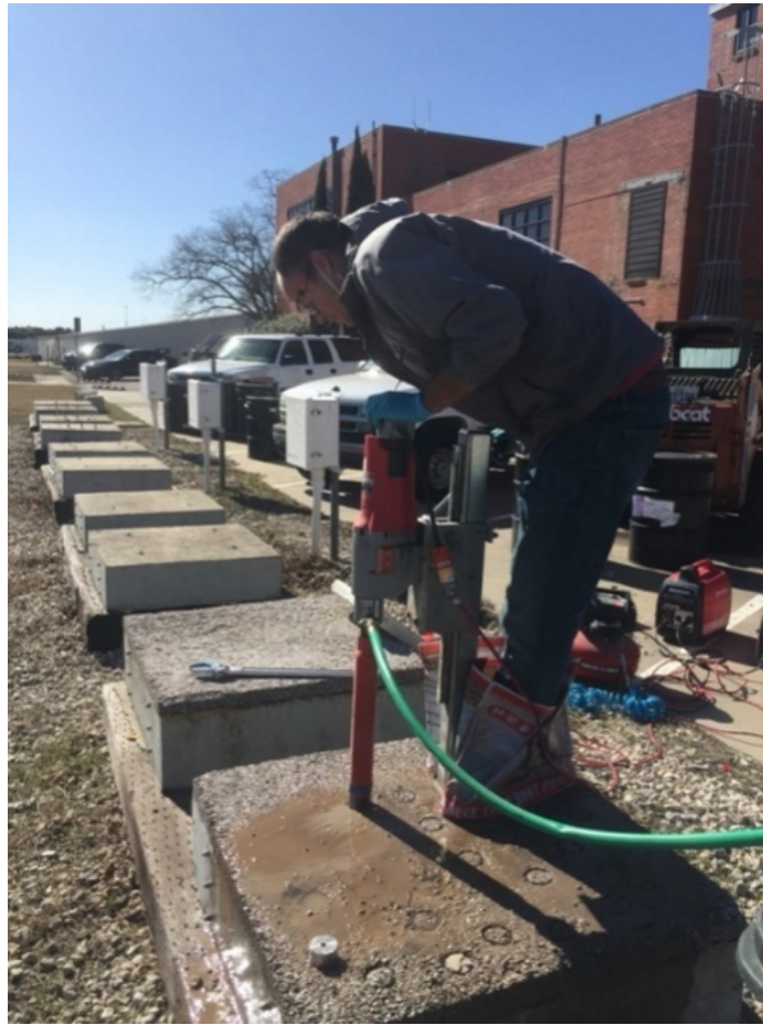
Figure 3.11. Coring of the asphalt overlay and concrete sub-surface by approximately 1/4"
