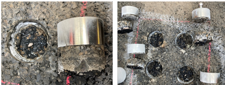
Figure 6.24. Pull-off test on IH69 using AR Type III as tack coat
