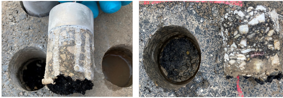
Figure 6.26. Waco NB widening section- diamond ground- No Treatment-Hot applied trackless tack
