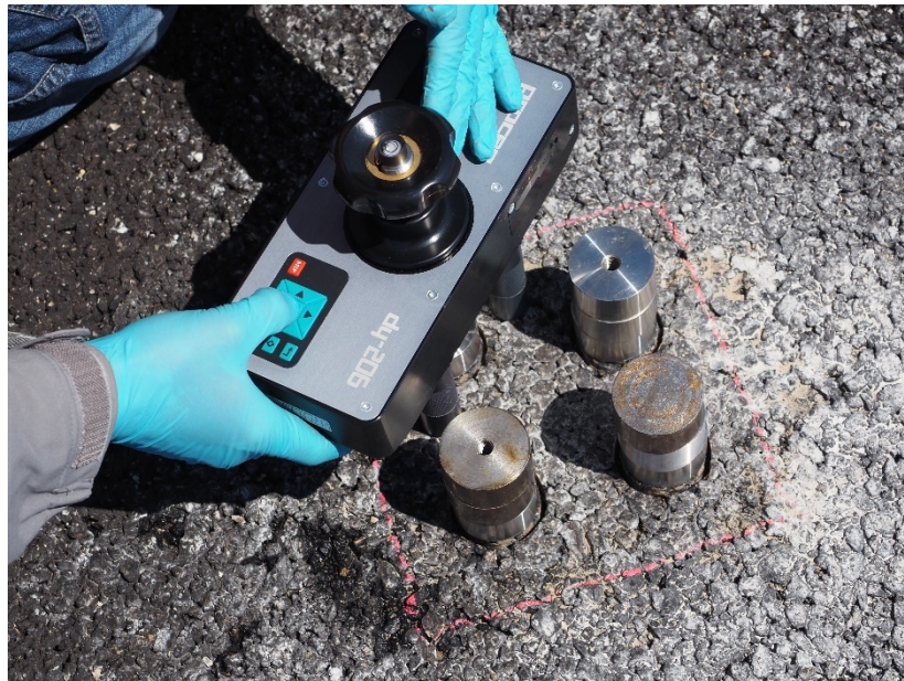
Figure 7. Conducting Pull-Off test.
