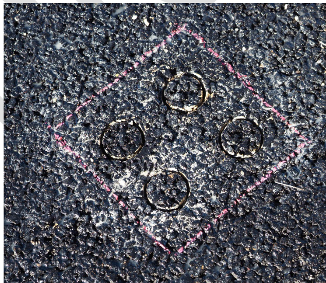
Figure 5. Cores in box outline
