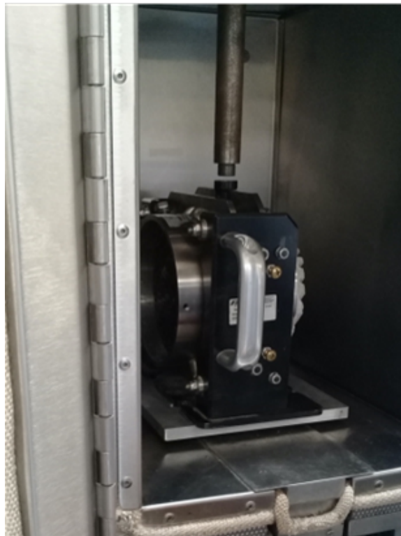
Figure 3.3. Interfacial layer shear strength device
