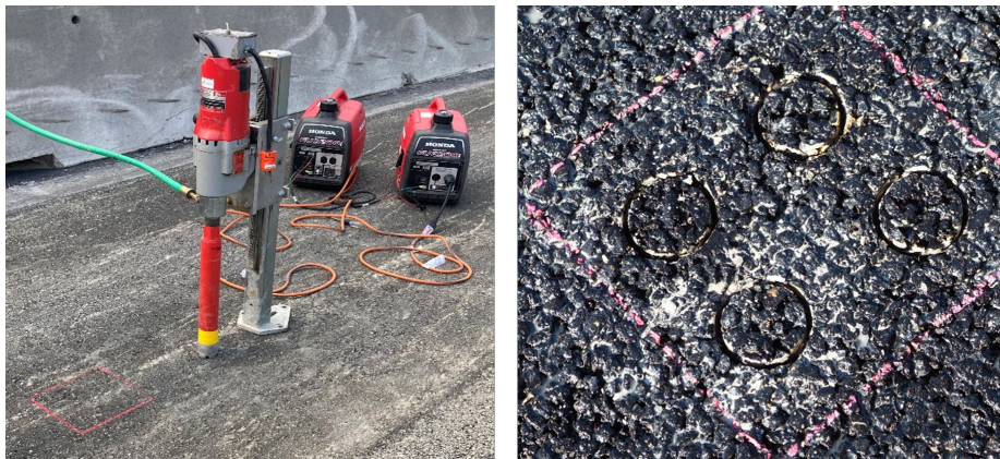
Figure 6.5. Procedure for obtaining 2-inch pull-off samples for in-situ field test
