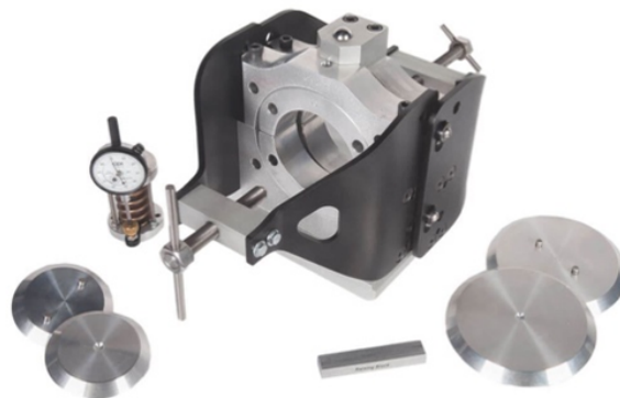
Figure 3.4. Tack coat shear strength tester (Gilson Inc.)
