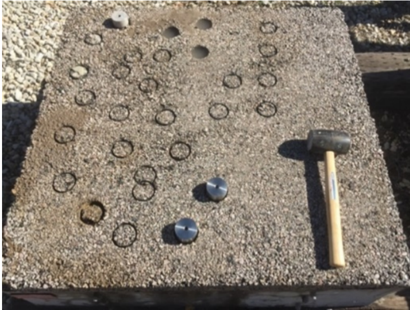
Figure 3.12. Metal caps on two specimens for pull-off test
