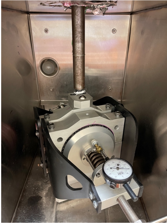
Figure 3—Loading Frame with Shear Strength Device
