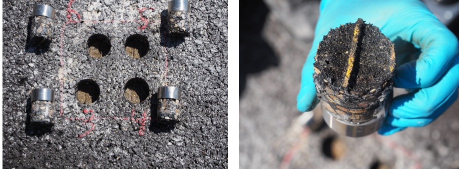
Figure 6.23. Pull-off test on SH130 using AR Type II as tack coat
