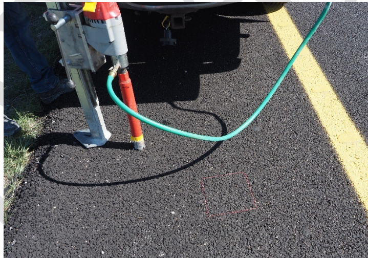
Figure 3. Core Drill Apparatus.
