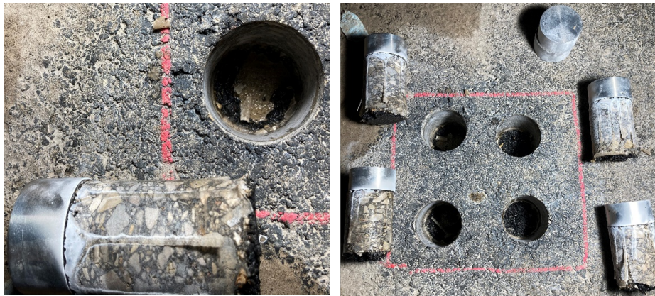
Figure 6.29. Waco SB widening- no treatment- no diamond grinding- hot applied trackless tack- 2nd spot
