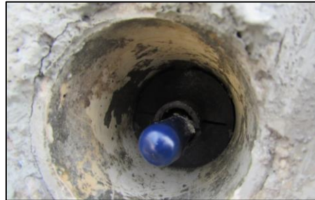
Figure 3-2: Outer End of Test Coupon with Protective Sleeve
