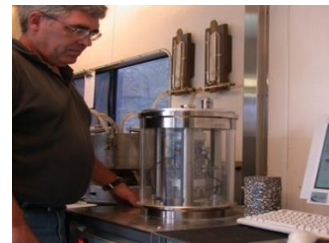
f) Testing in temperature-controlled chamber
