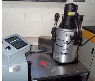
b) Compacting using the Gyratory Compactor
