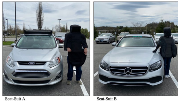
Figure 3. Seat-suit used for each L4/5 AV.
