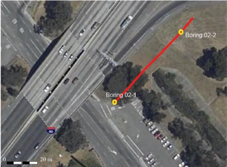
Figure 22. Plan view of location of refraction tomography measurements used to fill in between two boreholes at project site (courtesy of Caltrans) [3]
