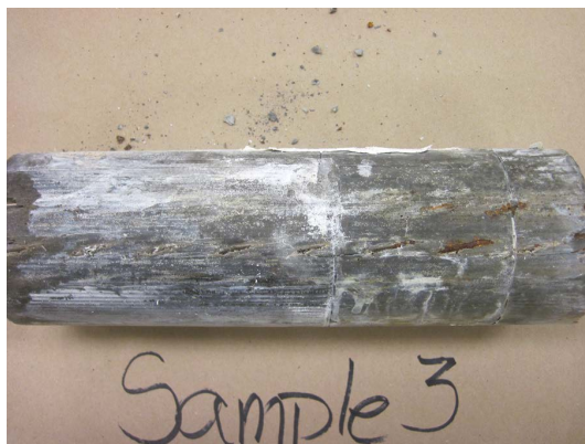
Figure 92. Photos. Treated specimen exposed to salt fog chamber. (112)
