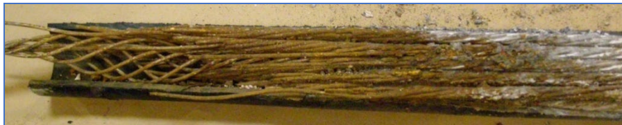
A. Closeup of the other end of the ruptured tendon.
