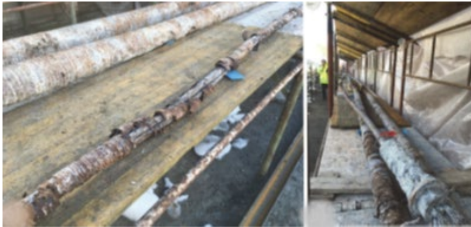
Figure 53. Photos. Severely damaged tendons extracted from collapsed La Reale Viaduct ramp. (81)
