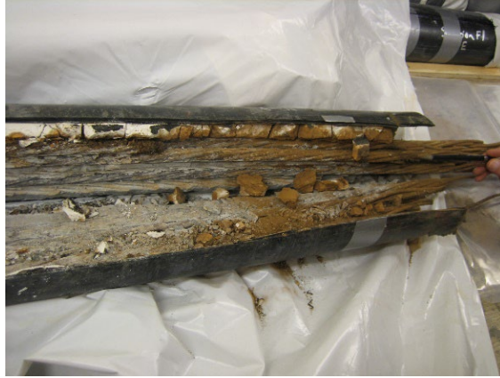
Figure 14. Photo. Interior condition of a failed tendon section.
