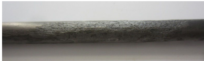
Figure 114. Photo. Uniform corrosion damage on an outer wire. (84)
