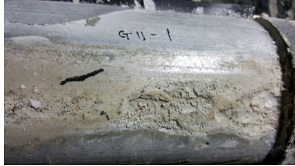
A. Localized soft/wet grout.
