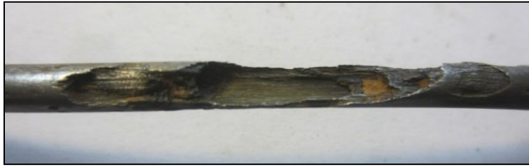
B. Elongated pitting damage.
