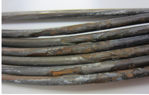
Figure 96. Photo. Close-up of corroded wires from a strand segment that came into contact with the porous grout layer. (72)
