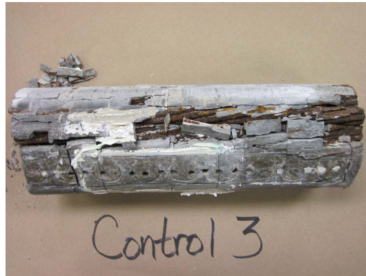
Figure 90. Photos. Control specimen exposed to salt fog chamber. (112)
