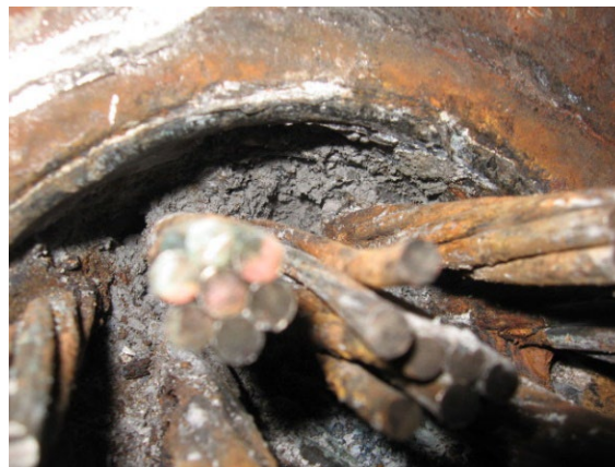
Figure 20. Photo. Interior of low-point anchorage of the second failed tendon.
