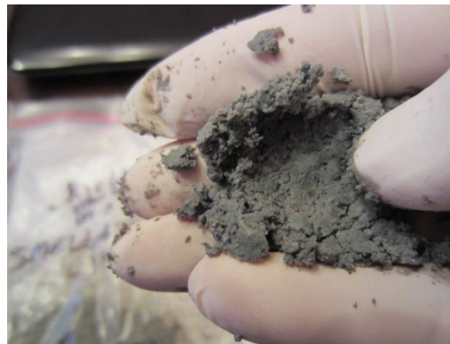
Figure 23. Photo. Claylike texture of a soft/wet grout sample.
