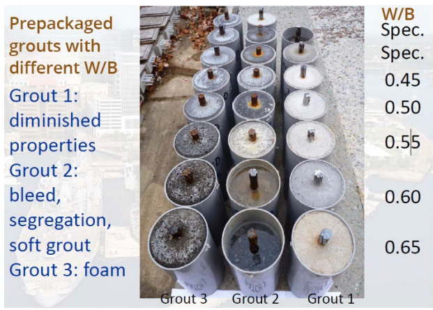
© 2015 M. Sprinkel. Modified by FHWA. W/B = water-grout powder ratio.
