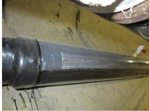
Figure 12. Photo. Condition monitoring section covered with a clear plastic tube.
