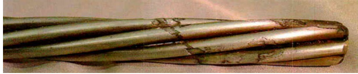
A. Corroded strand before removing gypsum grout.
