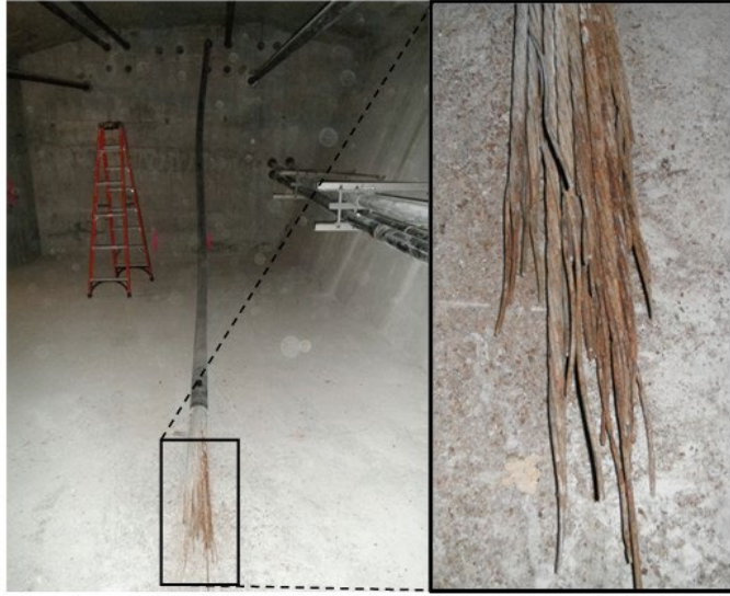
Figure 15. Photos. Ringling Causeway Bridge’s first failed tendon: Ruptured tendon and ruptured section. (35)
