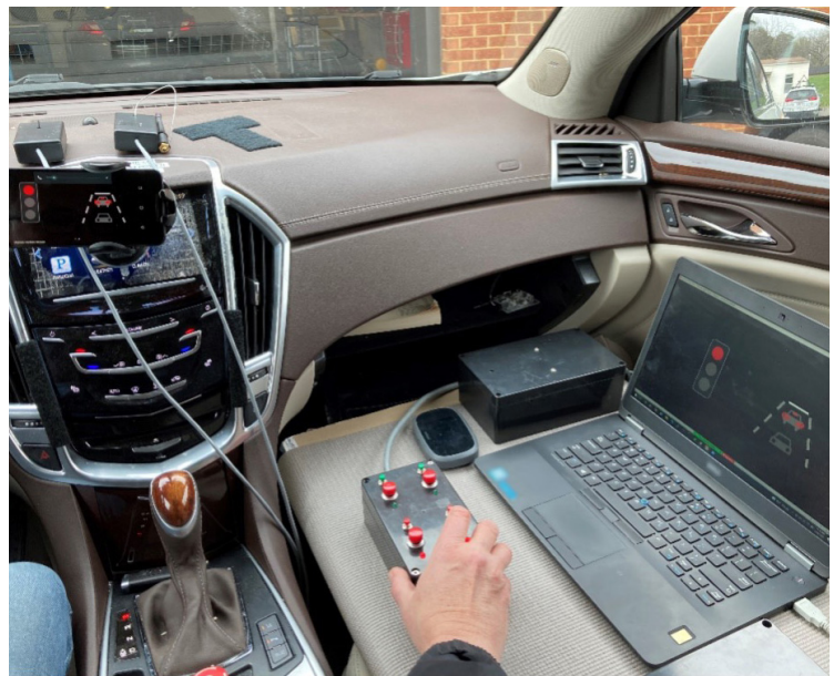
Figure 2. Photograph. In-vehicle signal and display control system for Exploring the Effects of Vehicle Automation and Cooperative Messaging on Mixed Fleets Eco-Drive project.
