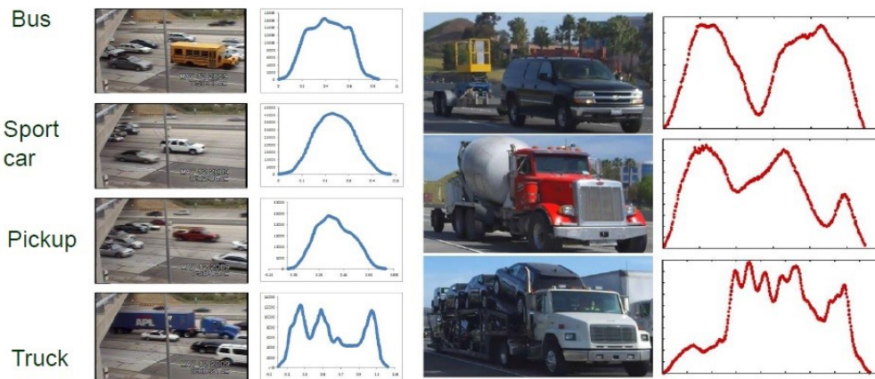
Figure 3.1 Loop Signatures for Different Type of Vehicles (Image from CLR Analytics Inc.).
