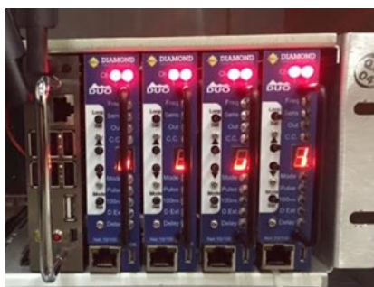
Figure 3.2 Inductive Loop Signature Cards for Vehicle Classification (Image from CLR Analytics Inc.).
