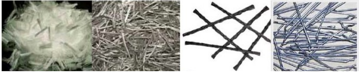
Figure 2-22. Fibers used in the Kevern et al. (2016) study: polypropylene fibrillated fiber (left), polypropylene macro fiber (left middle), carbon fiber (right middle) and steel fiber (right).
