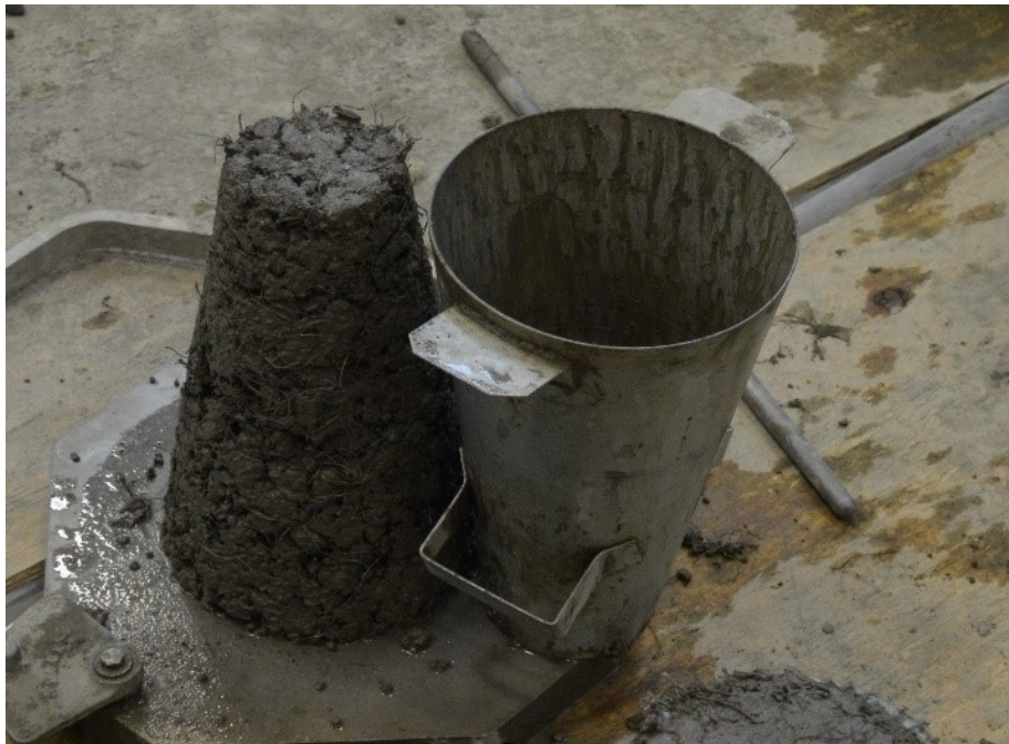
Figure 4-6. Slump test on FRC mixture.
