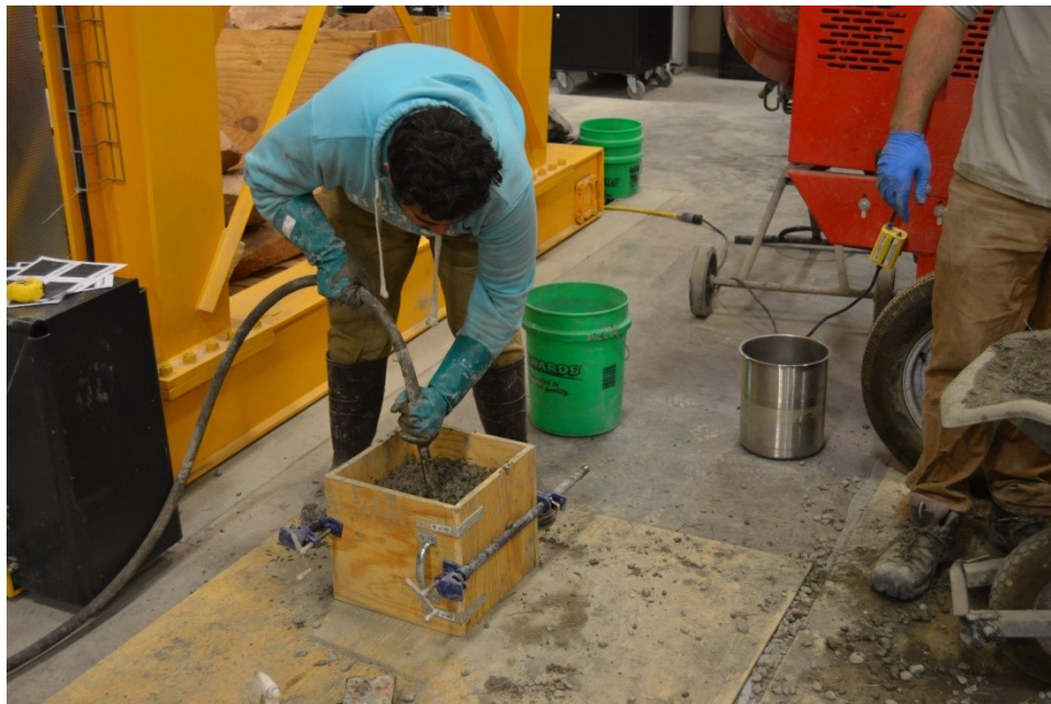
Figure 4-9. The Box test in progress.
