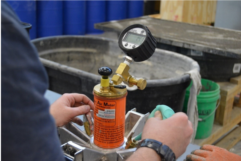
Figure 4-7. The air content by pressure method test in progress.
