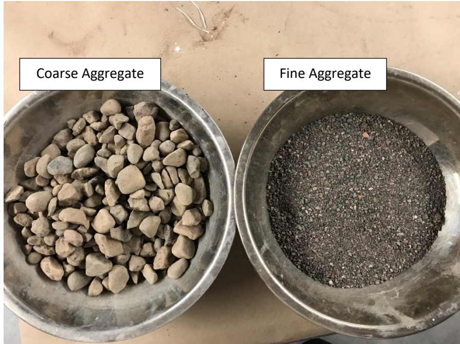
Figure 4-2. Coarse aggregate and fine aggregate used in this project.
