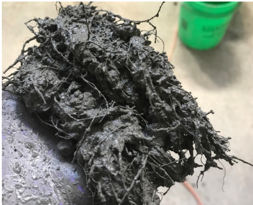
Figure 4-5. Fiber balling in a concrete mixture.
