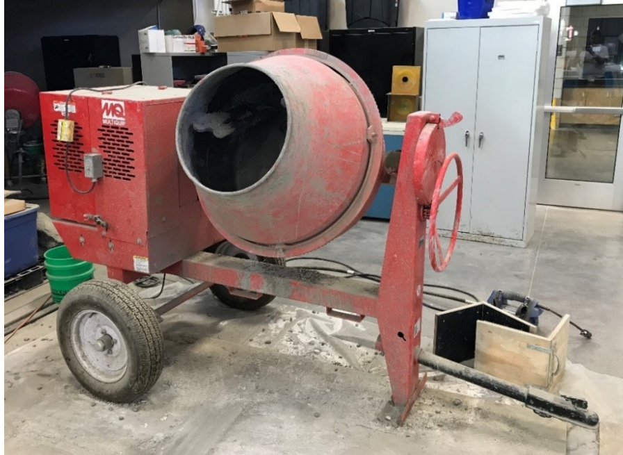
Figure 4-4. Concrete mixer used in this project.
