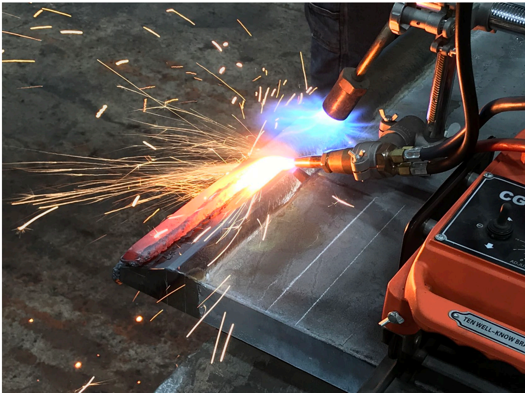
Figure 6 Cutting a 60° Transition – (Pre-Heat Applied in Advance of the Cut)
