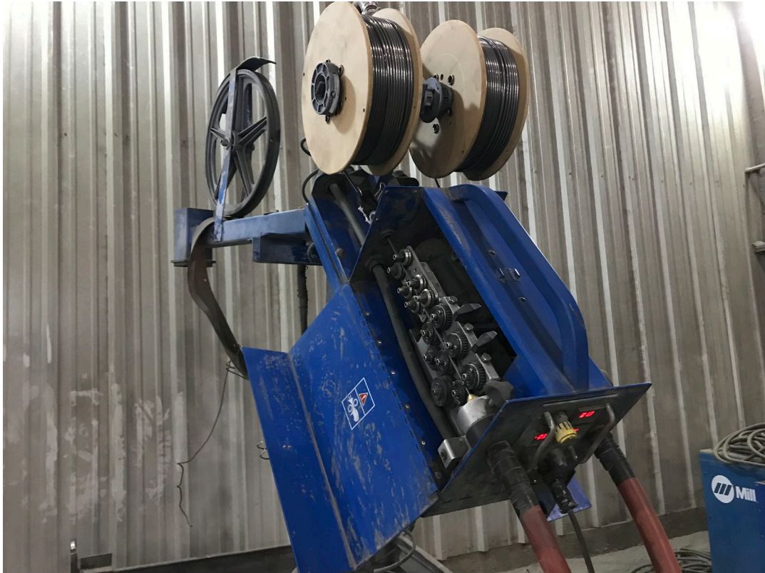
Figure 16 Thermion® Twin Wire Feed Unit
