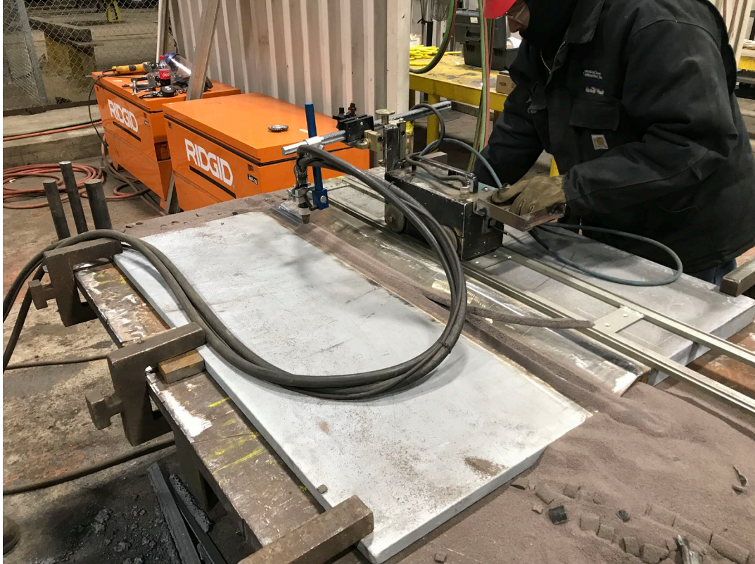
Figure 7 Sub-Arc Welding Using Lincoln Electric Flextec® 650X Welder with a 74 HT Flex Feed™ Coupled with the Bug-O Transport System
