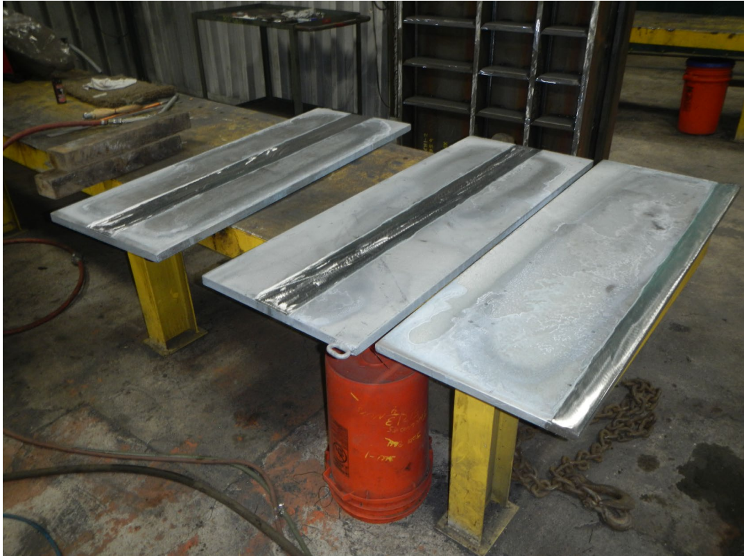
Figure 3 Steel After Removal of Galvastop®
