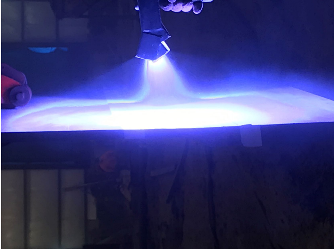
Figure 20 Smaller Spray Pattern May Reduce Overspray Cleanup
