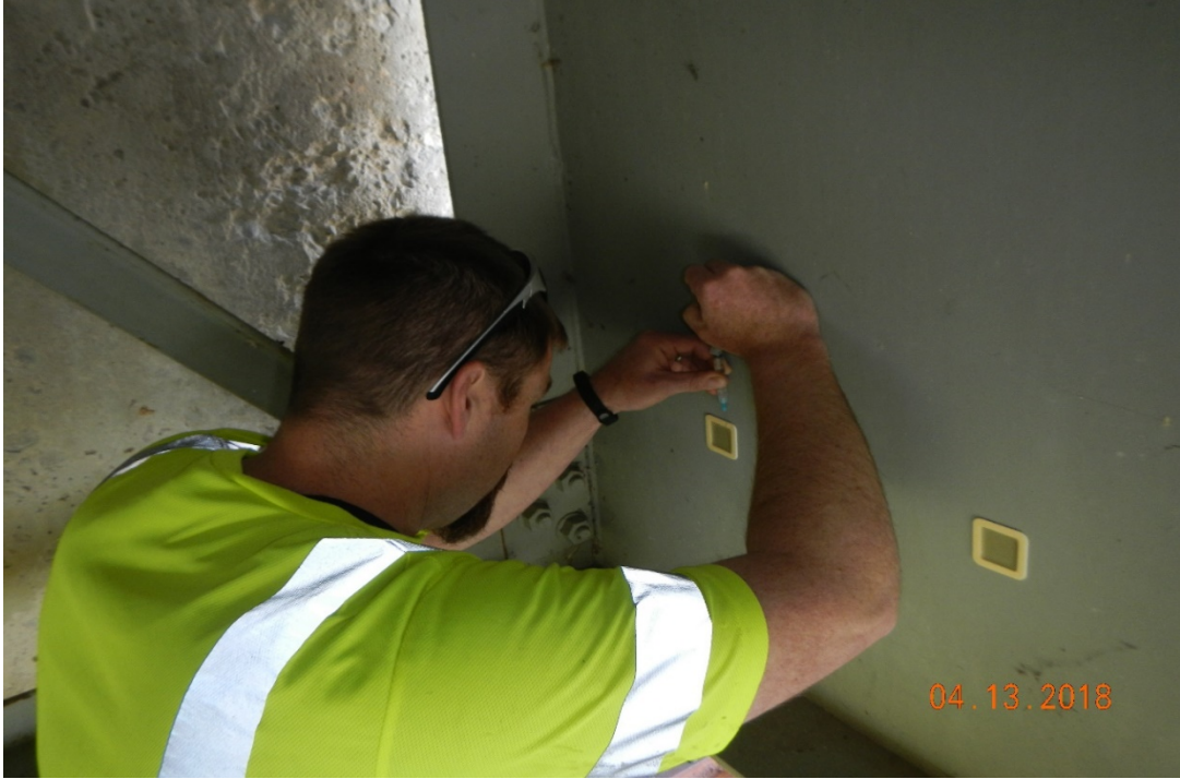
Figure 24 KTC Personnel Performing CI Testing
