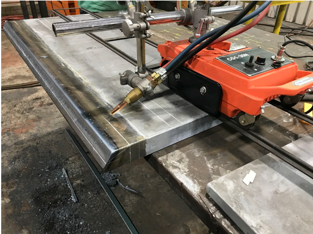
Figure 5 Setup for Cutting 60° Transition
