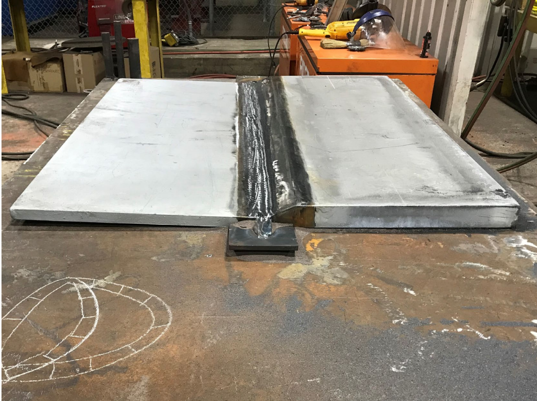
Figure 8 Distortion From Welding Process
