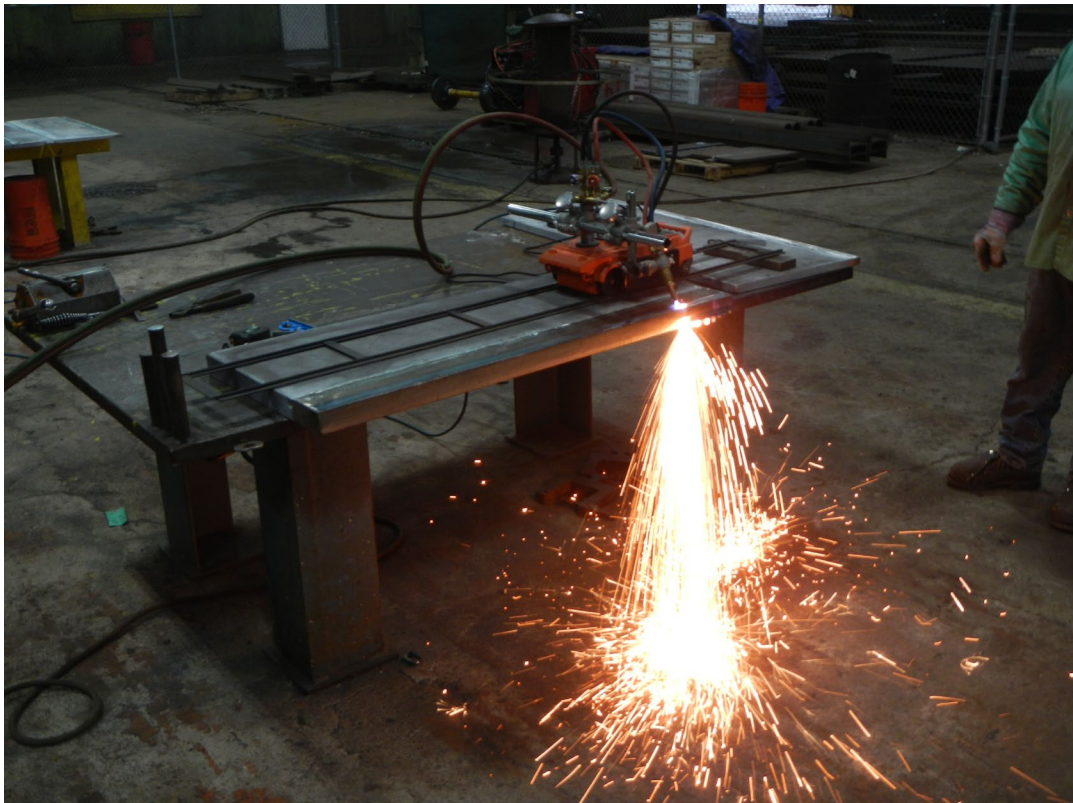
Figure 4 Steel Cutting Using Ten-Know Brand CG1-30N Track Cutting Equipment
