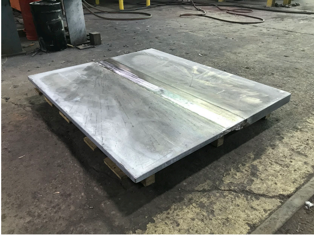
Figure 10 Moved to a Pallet For Transport After Welding Was Complete
