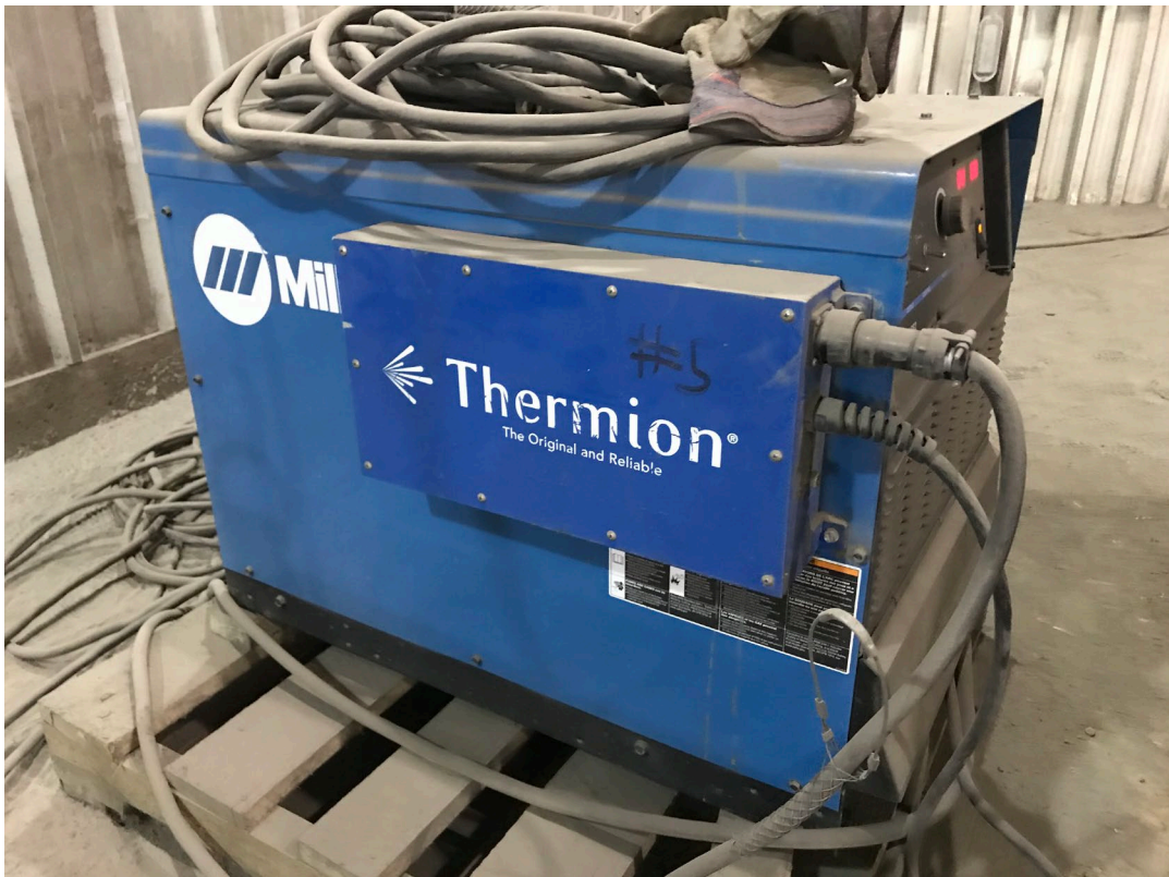
Figure 17 Miller Deltaweld® 652 Power Source for Thermion® Precision Arc System
