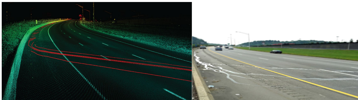
Figure 3.3 I-471 Flowpath Model (Left) and Field Observations (Right)
