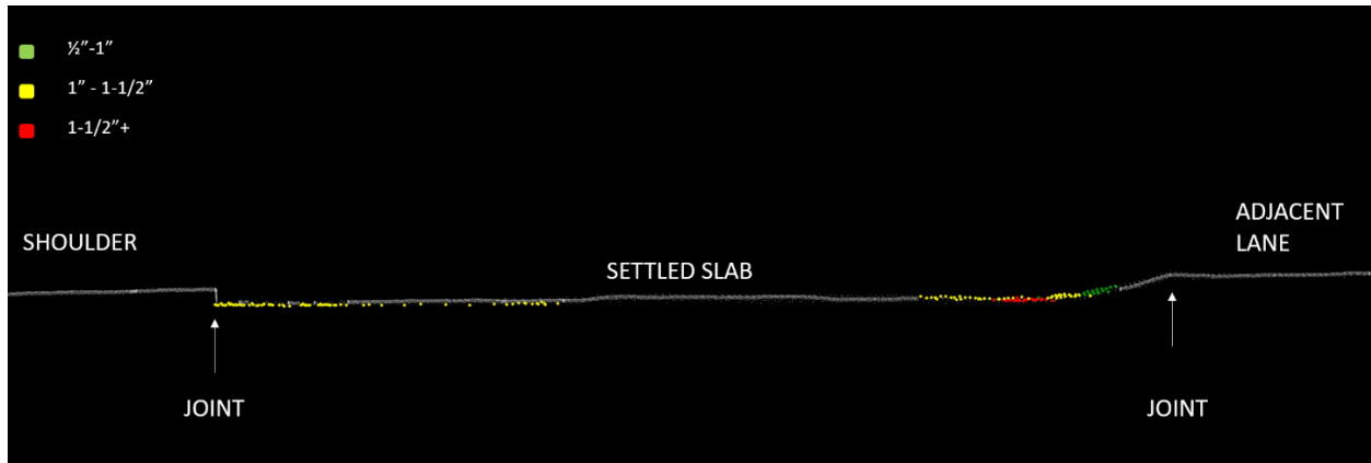
Figure 3.7 Settled Slab Cross Section
