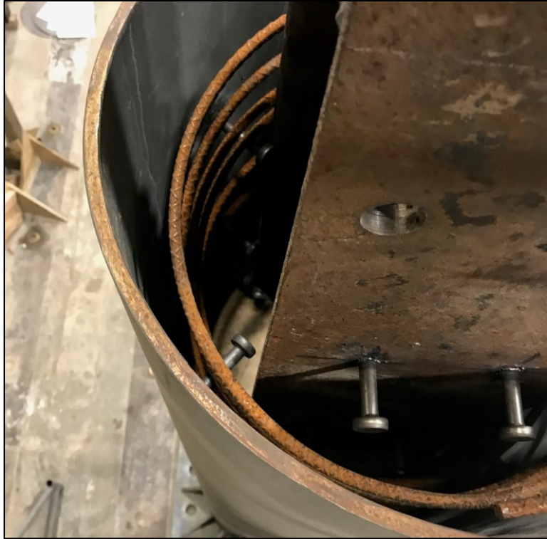
Figure 5-32 - HP10x57 and Confinement Placed in Sign Post
