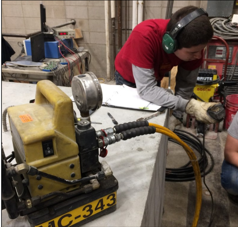
Figure 4-2 - Operation of Hydraulic Wrench
