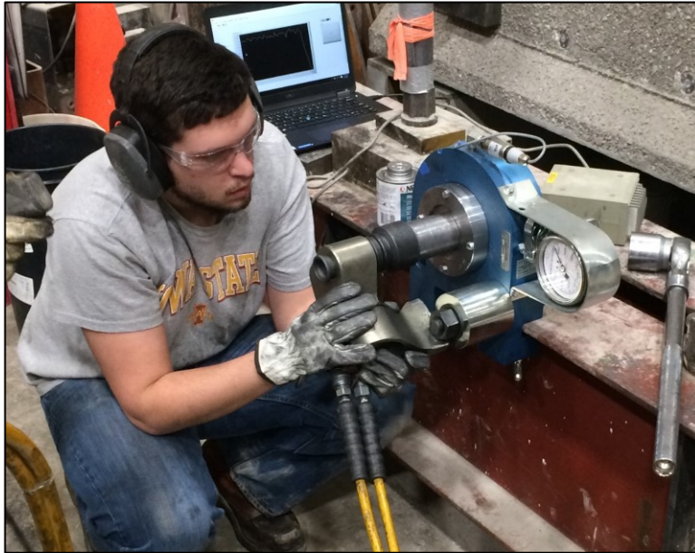
Figure 4-1 - Hydraulic Wrench Tightening
