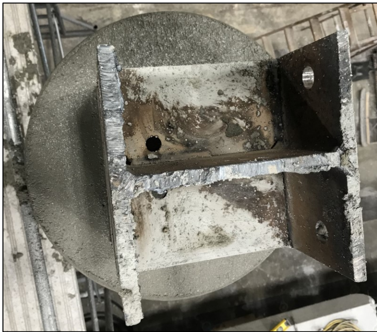
Figure 5-35 - Top View HP10x57 Curing in Concrete
