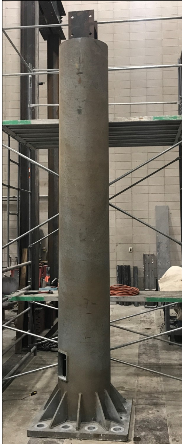
Figure 5-33 - H-Pile Placed Inside Sign Post
