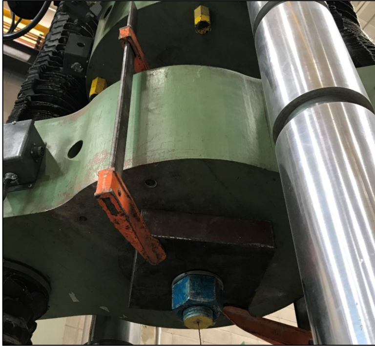
Figure 5-7 - Calibration of Anchor Bolts
