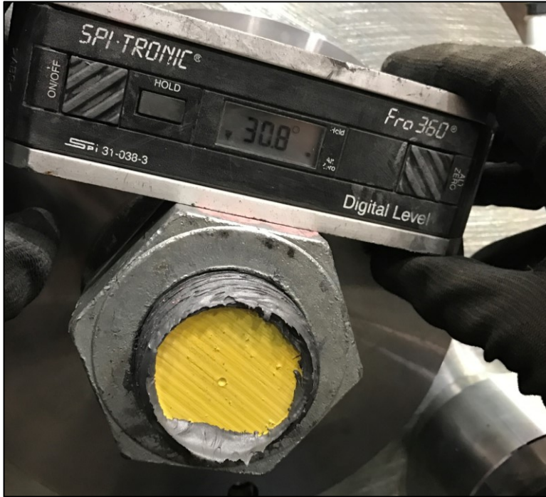
Figure 4-6 - Digital Level Measurement after Tightening
