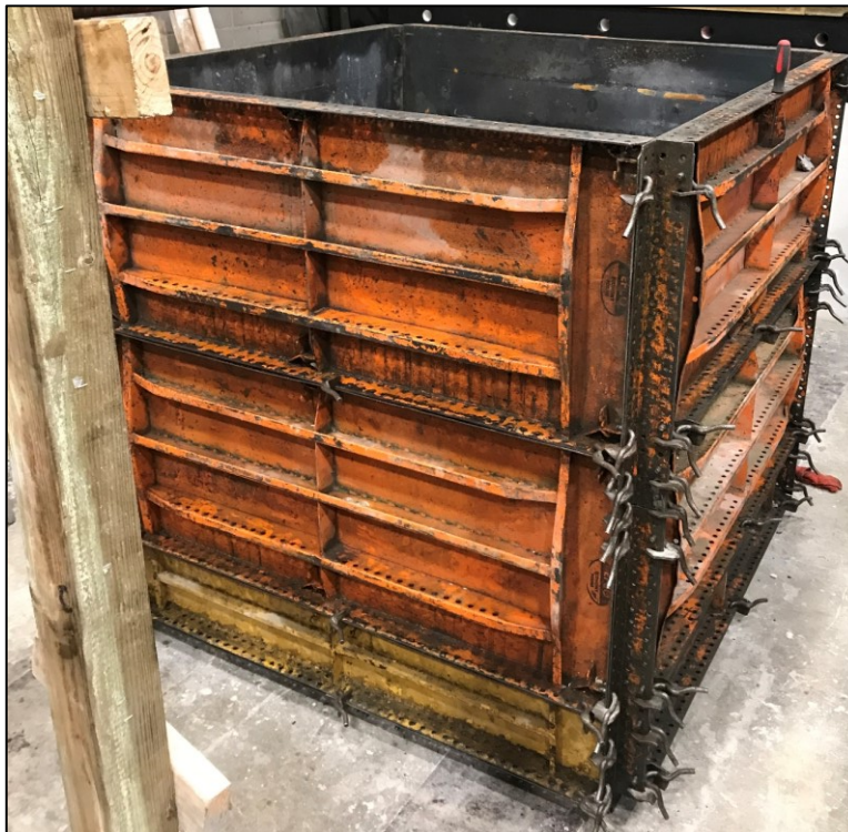
Figure 5-25 - Concrete Block Formwork
