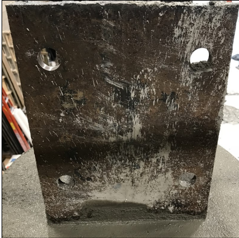
Figure 5-34 - HP10x57 Curing in Concrete
