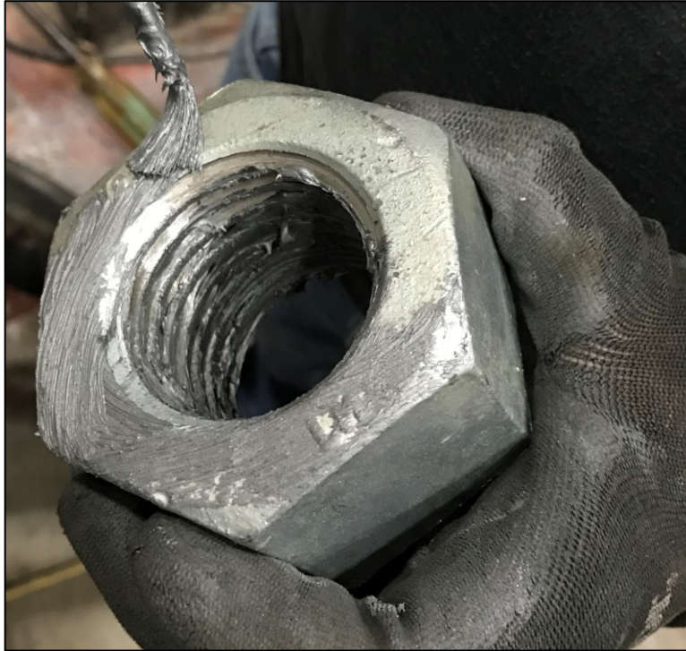
Figure 4-4 - Lubrication of Nut Bearing Surface
