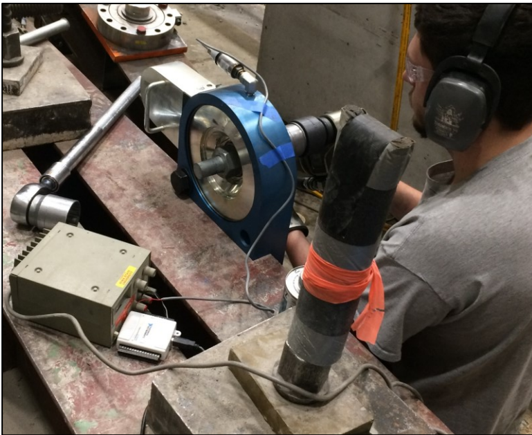
Figure 4-3 - Skidmore Wilhelm Instrumentation
