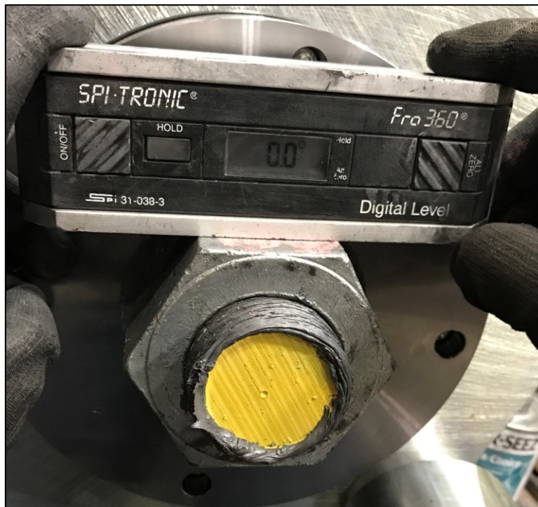
Figure 4-5 - Zeroing of Digital Level
