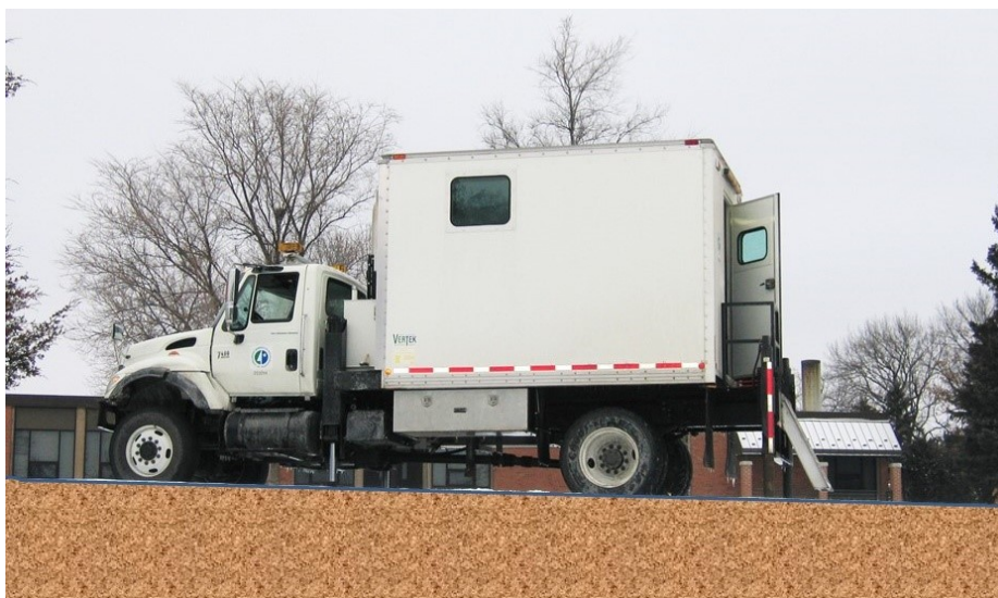
Figure A2. CPT truck-mounted rig used by MnDOT.
