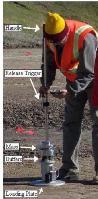
Figure 11 Light Weight Deflectometer as used in the field. (From Fig. 1.2 of Siekmeier et al. [2009])
