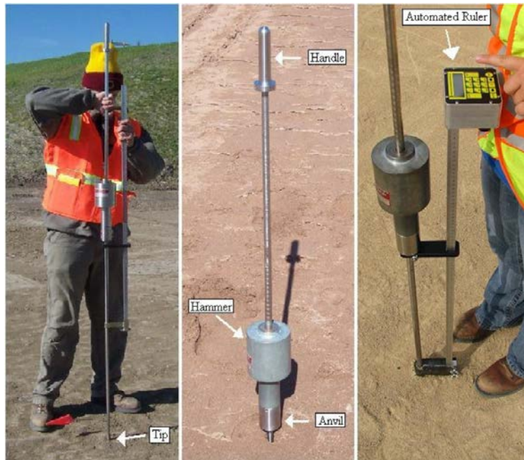
Figure 9 Dynamic Cone Penetrometer as used in the field. (From Fig. 1.1 of Siekmeier et al. [2009])
