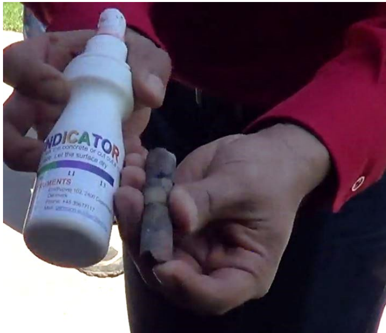
Figure 37 Use of indicator solution to measure depth of carbonation in small concrete core sample
