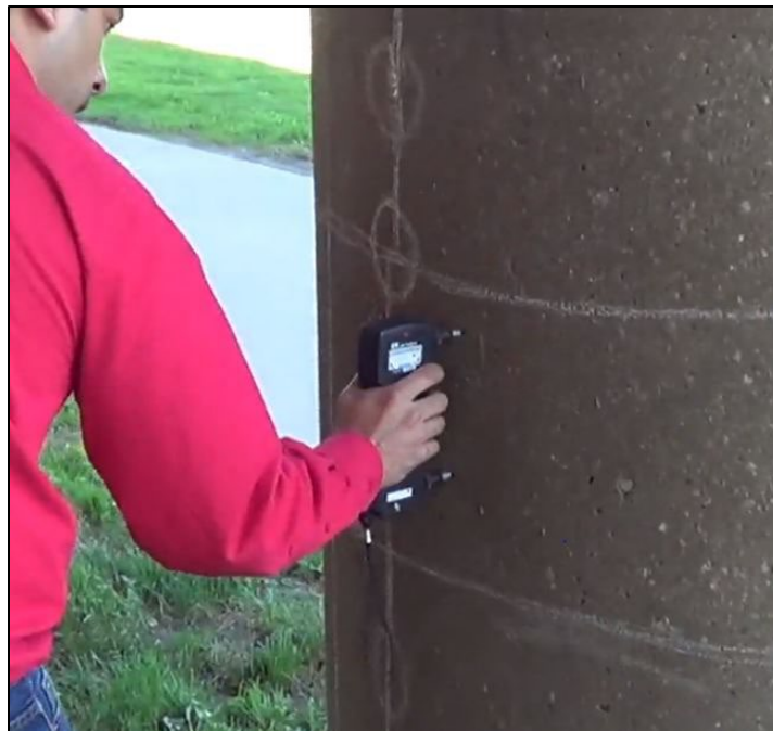
Figure 25 Measuring crack depth using the pulse velocity (time-of-flight) indirect method
