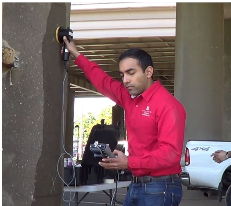
Figure 29 Galvastatic pulse tester used for corrosion current, half-cell corrosion potential and concrete resistivity. The operator is applying the probe to the surface of the concrete with his right hand and reading the instrument held in his left hand.
