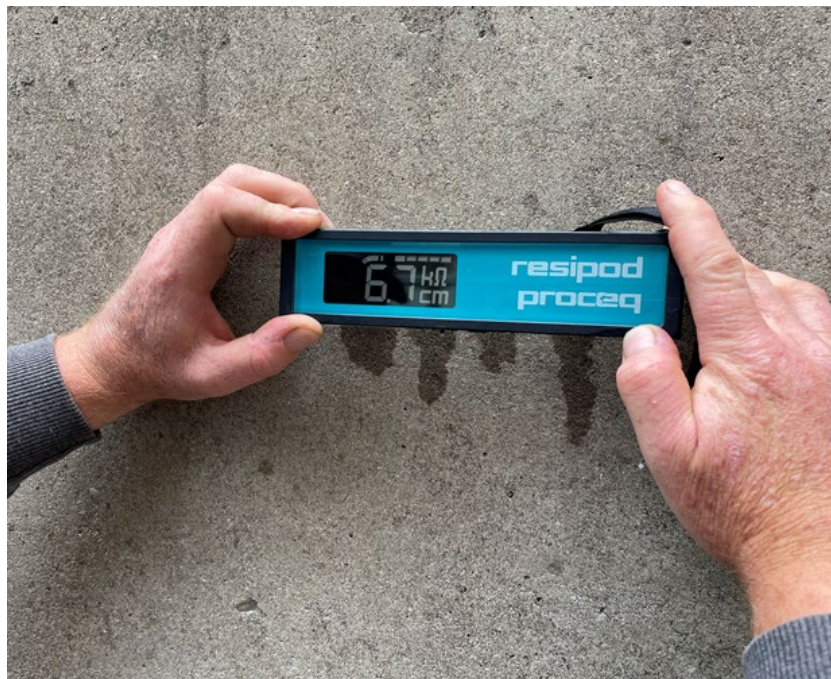
Figure 33 Measuring concrete resistivity using a Wenner four-point probe instrument
