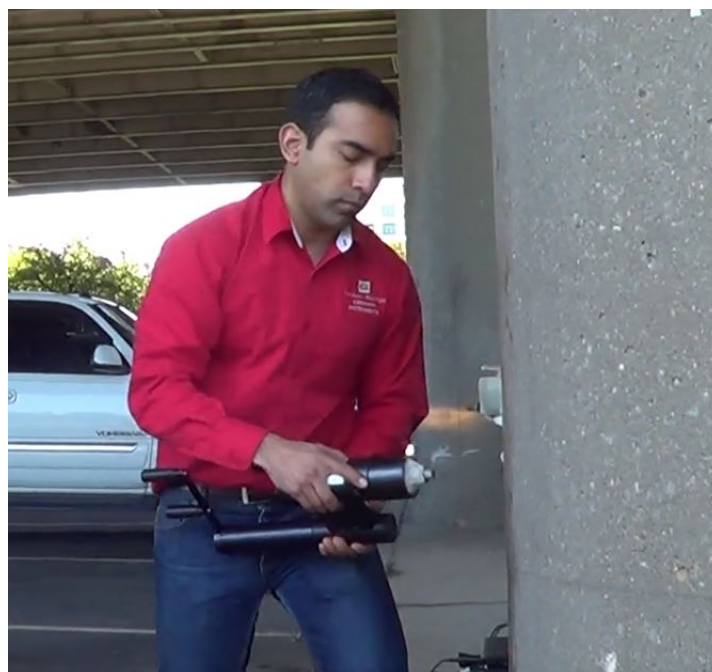
Figure 19 Measuring concrete strength using the lateral pullout test
