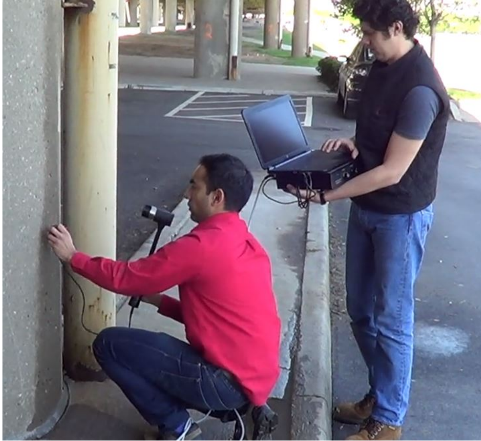
Figure 22 Testing of a concrete column using the impulse response method. The hammer operator is holding the transducer on the column with his left hand while hitting it with the instrumented hammer held in his right hand.
