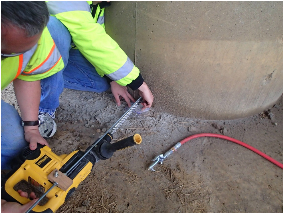
Figure 8 Extracting powder samples from column on I-65 to perform laboratory chloride tests (2013)
