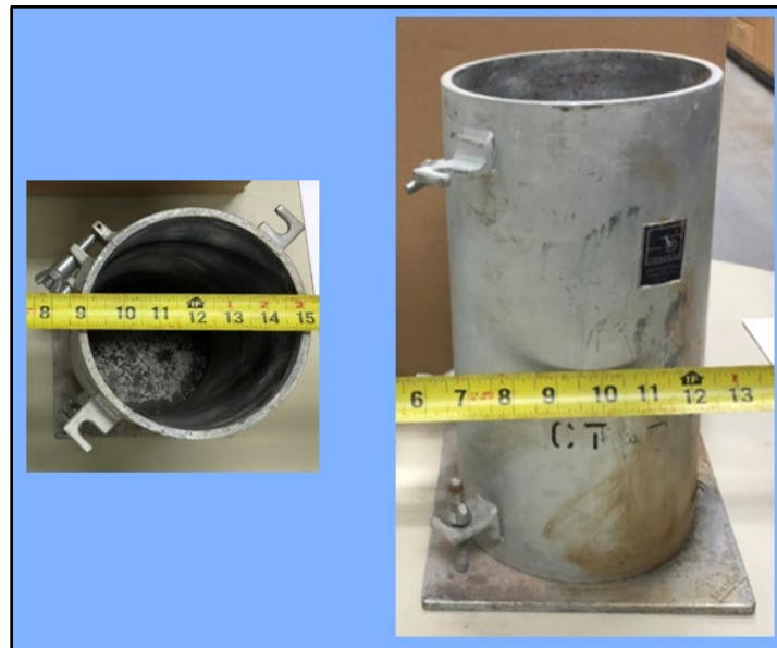
Figure 3.2 Cylindrical Steel Container
