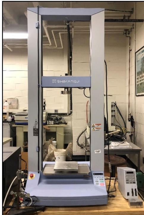
Figure 3.1 SHIMADZU AGS-X Tabletop Precision Universal Tester
