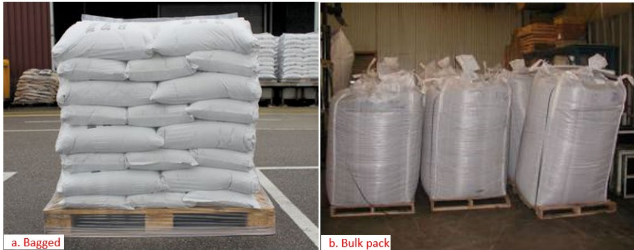
Figure 4.1 Delivery Methods for Packing Recycled Tire Derivatives
