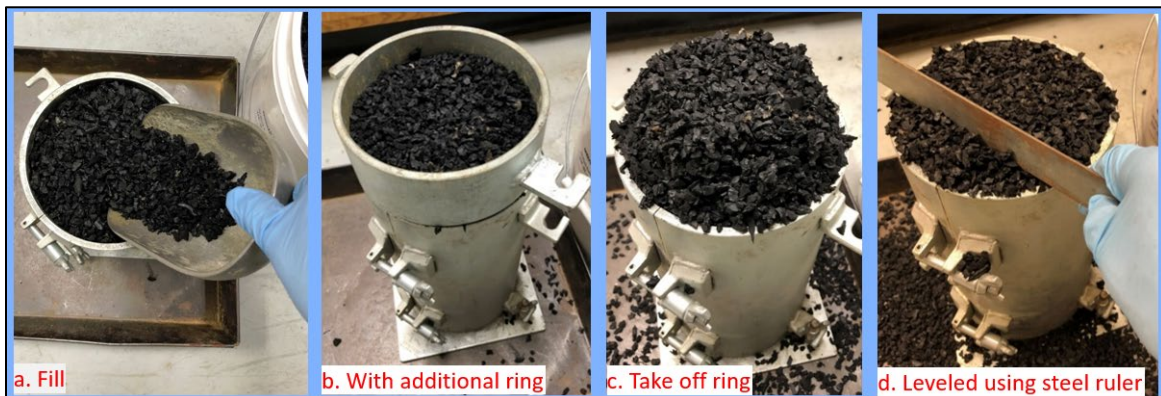
Figure 3.3 Method of Filling Cylindrical Steel Containers with Recycled Tire Granules
