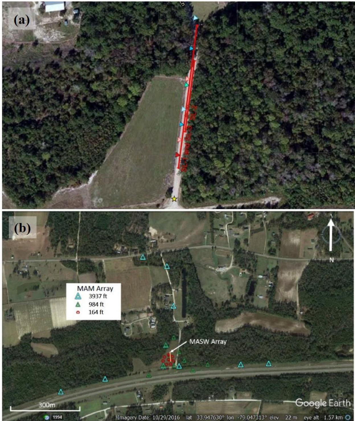
Figure 3.3 Surface Geophysical Testing Locations at Site A: (a) MASW and SASW Testing Arrays, (b) MASW and MAM Testing Arrays
