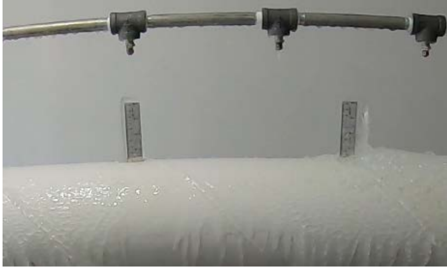
Figure 22 Rulers attached above sheath used to estimate ice lens thickness measurements
