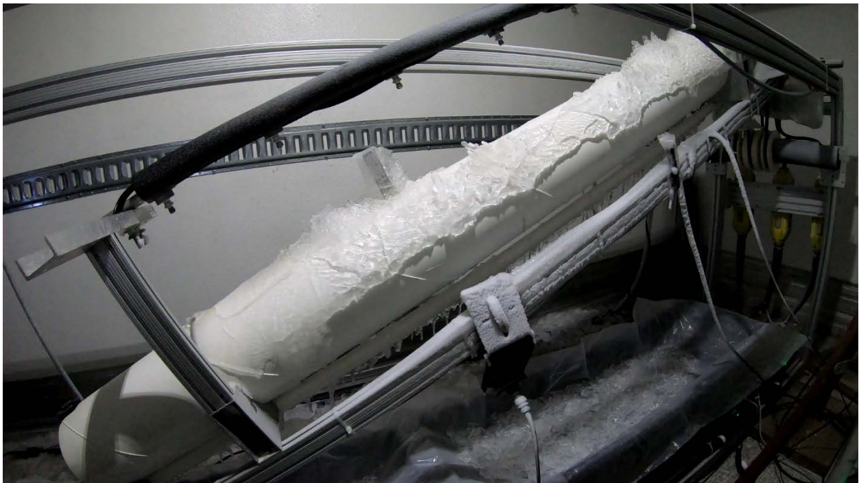
Figure 29 Example ice shed at 25° sheath angle, heavy ice accumulation - 4 cycles
