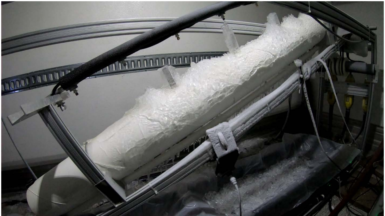
Figure 27 Example ice shed at 25° sheath angle, heavy ice accumulation - 2 cycles
