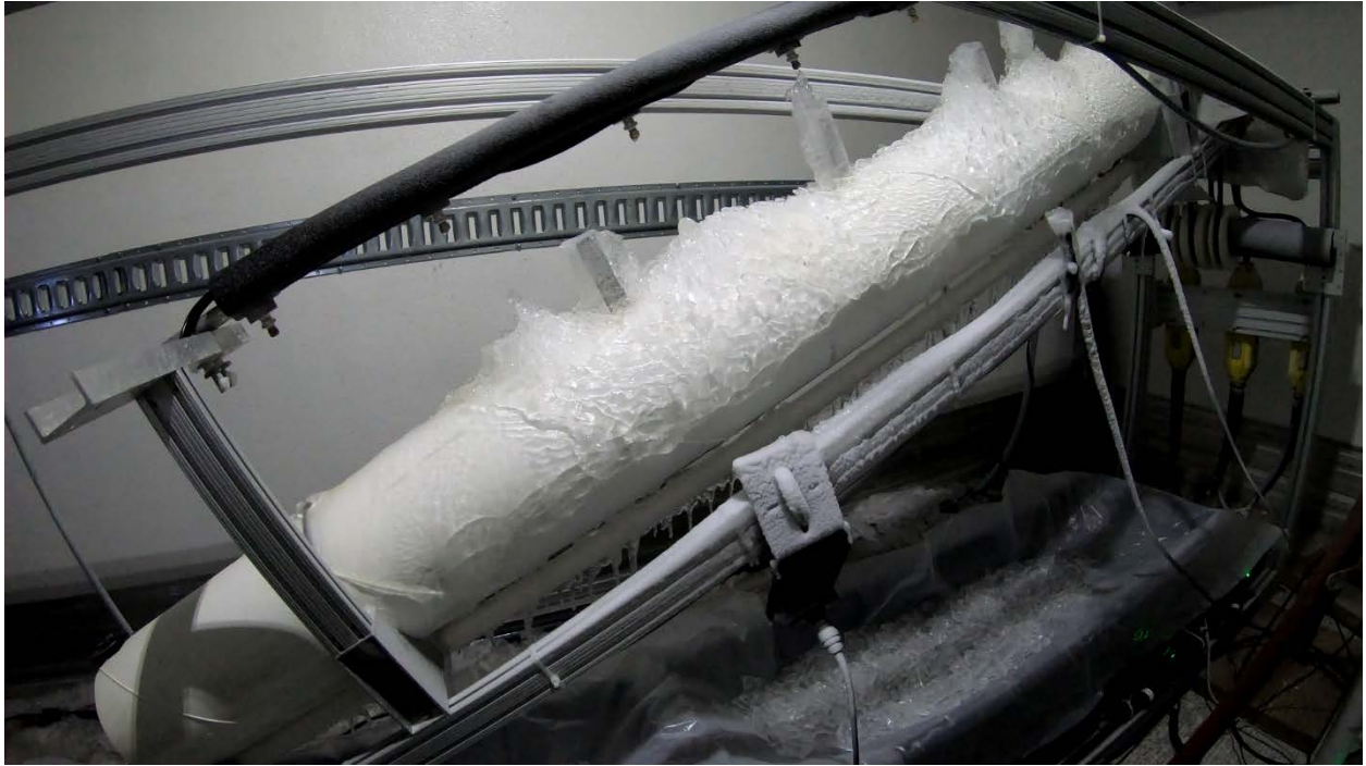
Figure 26 Example ice shed at 25° sheath angle, heavy ice accumulation - 1 cycle
