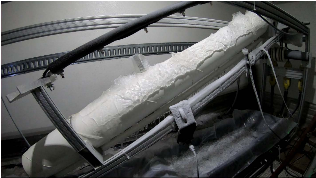
Figure 28 Example ice shed at 25° sheath angle, heavy ice accumulation - 3 cycles
