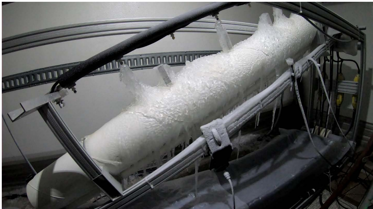
Figure 25 Example ice shed at 25° sheath angle, heavy ice accumulation - 0 cycles
