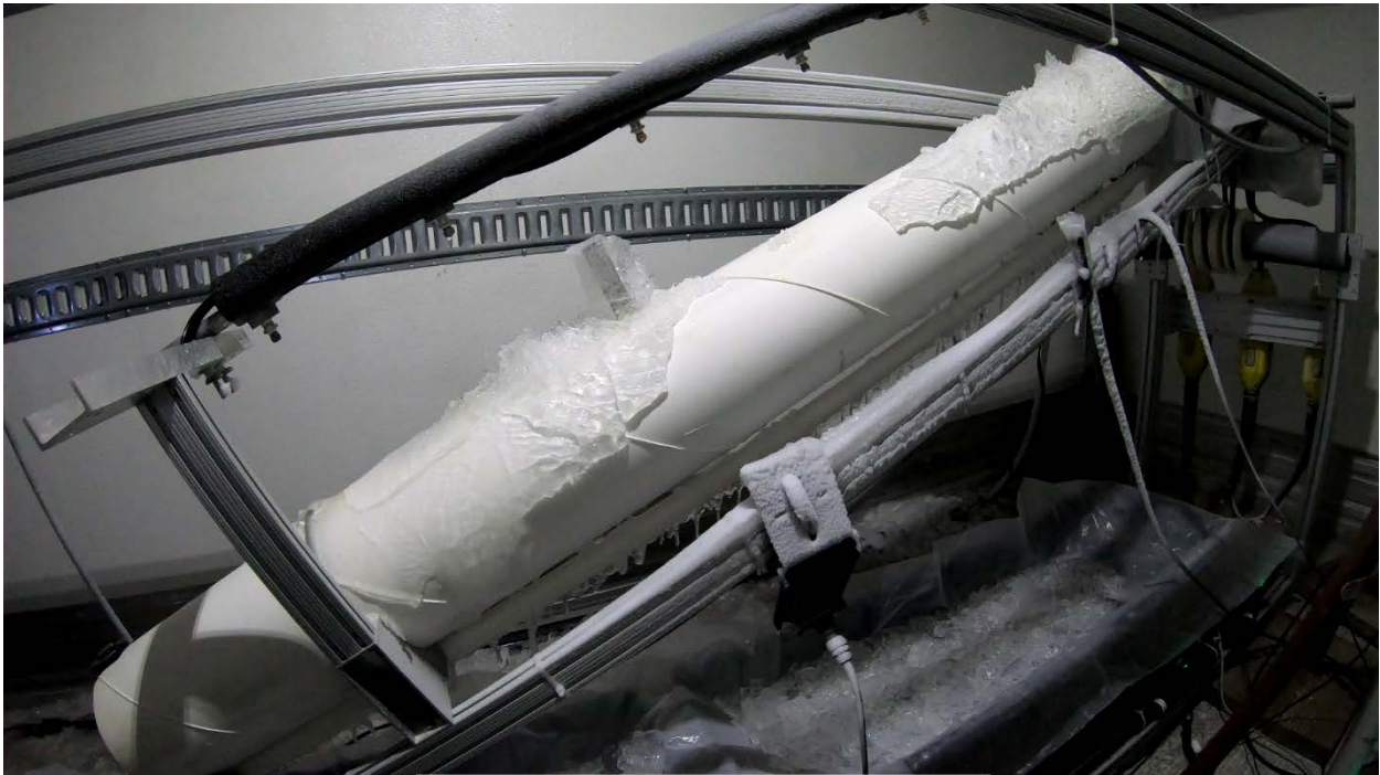
Figure 30 Example ice shed at 25° sheath angle, heavy ice accumulation - 5 cycles
