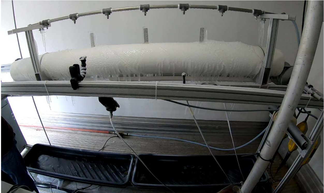
Figure 19 Example image of ice formed by the spray system in one the performance tests
