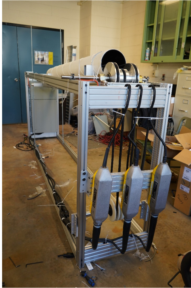
Figure 16 Frame fully assembled with cable management pulley system
