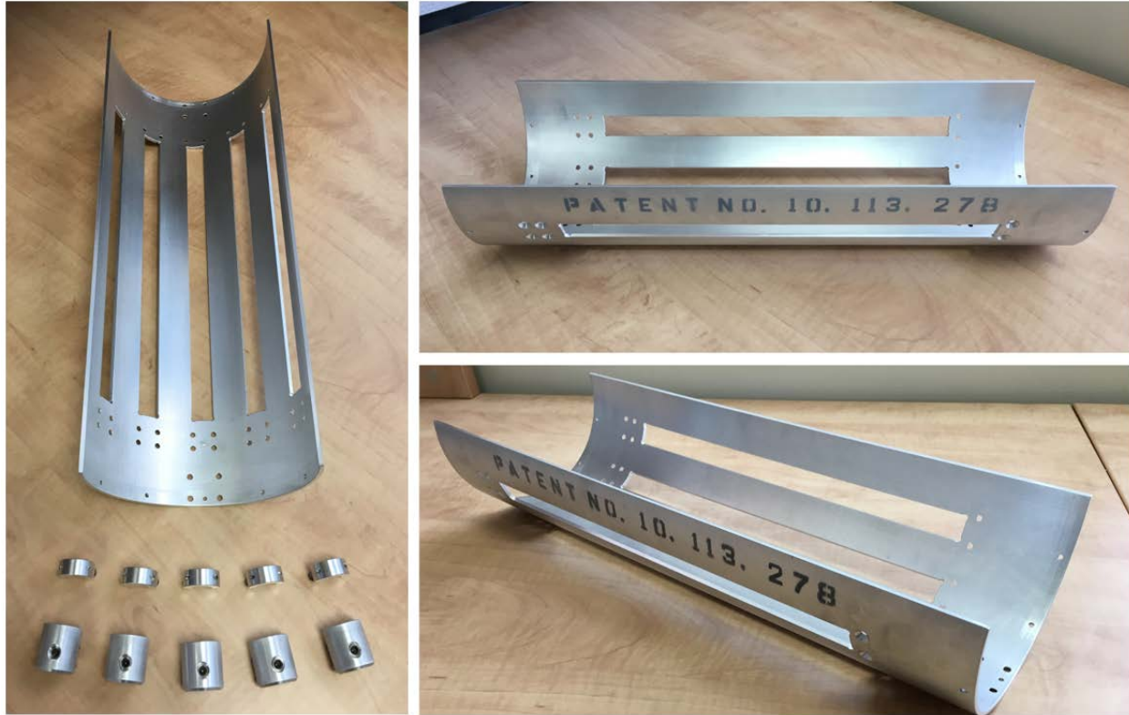
Figure 12 Machined aluminum SHAKEY sled with vibrator attachment pieces
