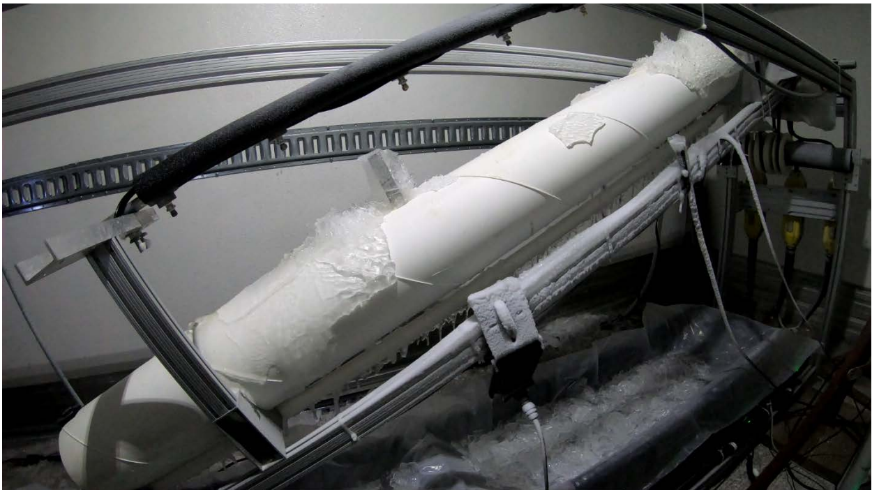
Figure 31 Example ice shed at 25° sheath angle, heavy ice accumulation - 6 cycles
