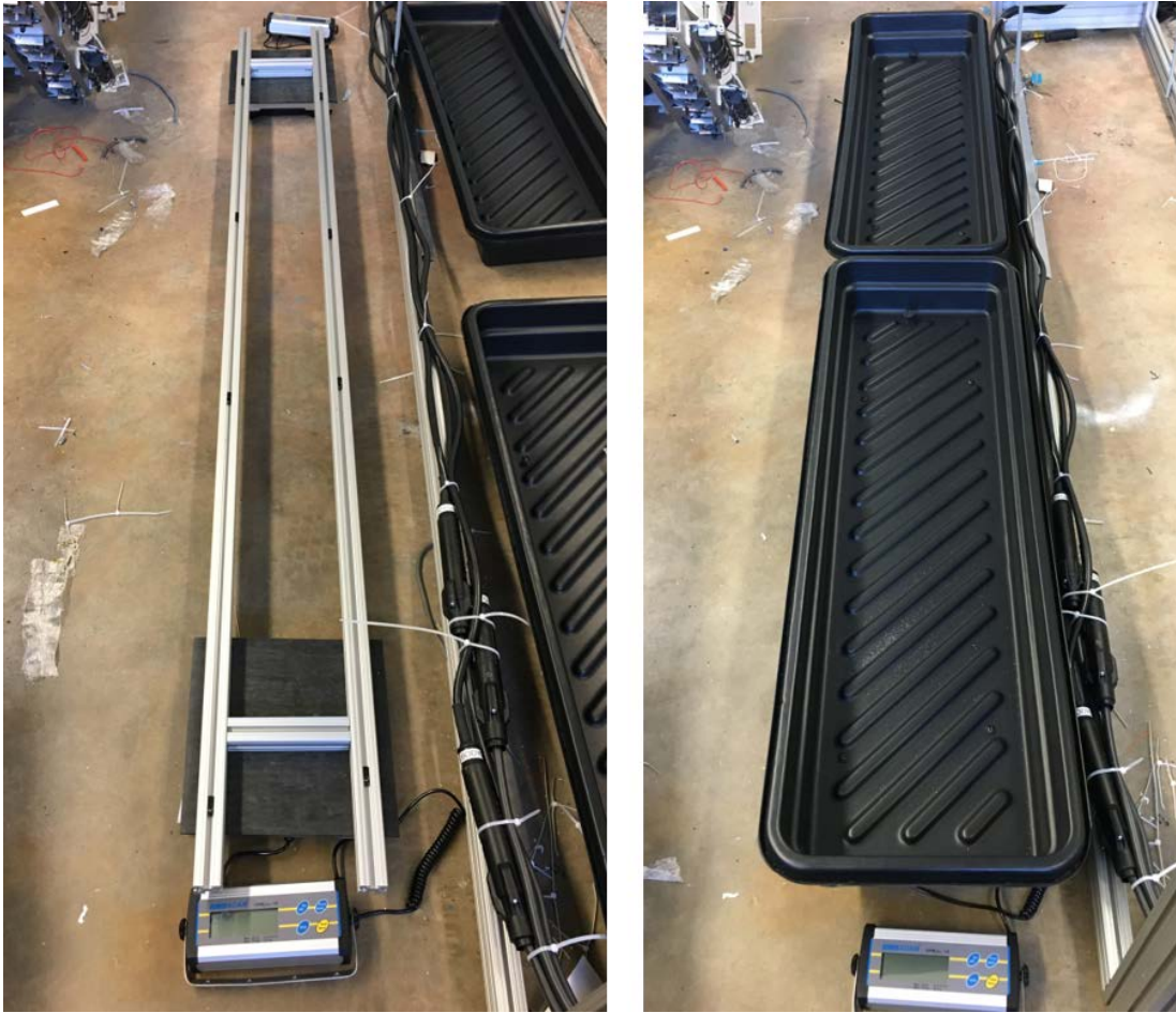
Figure 23 Ice shed catch basin frame and bench scales (left). Basin sitting on top of scales (right)
