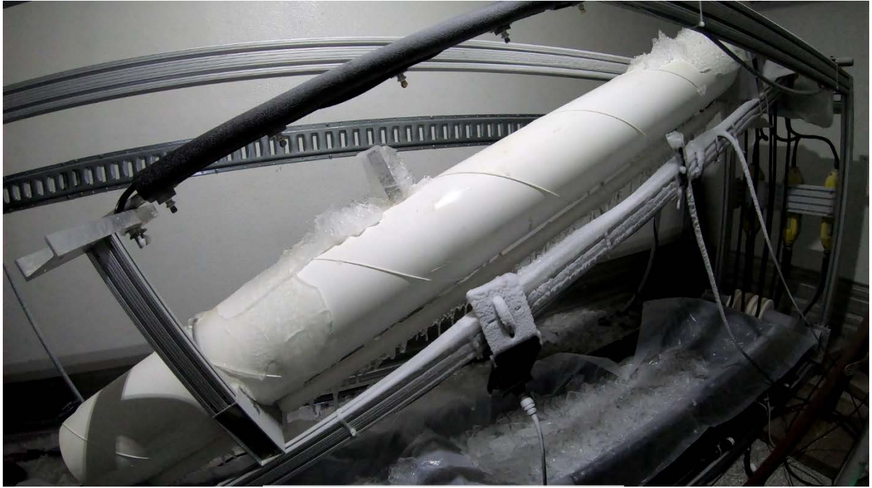
Figure 32 Example ice shed at 25° sheath angle, heavy ice accumulation - 7 cycles
