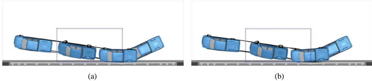
Figure 4.23: Vehicle trajectories of 2007 Chevy Silverado impacting the Oregon Rail. (a) With expansion joint as reference; and (b) with the post as reference.
