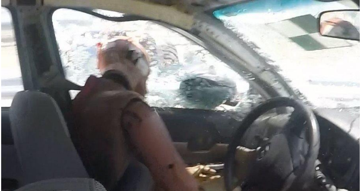
Figure 94. Maximum Occupant Head Protrusion, Test No. NCBR-1
