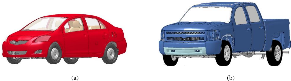
Figure 1.2: Finite element models of two MASH-compliant test vehicles. (a) 2010 Toyota Yaris; and (b) 2007 Chevy Silverado quad cab.
