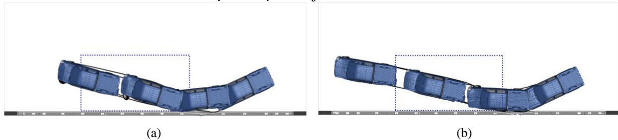
Figure 4.57: Vehicle trajectories of 2014 Chevy Silverado impacting 3BMR-2 under TL-3 conditions. (a) With expansion joint as reference; and (b) with the post as reference.
