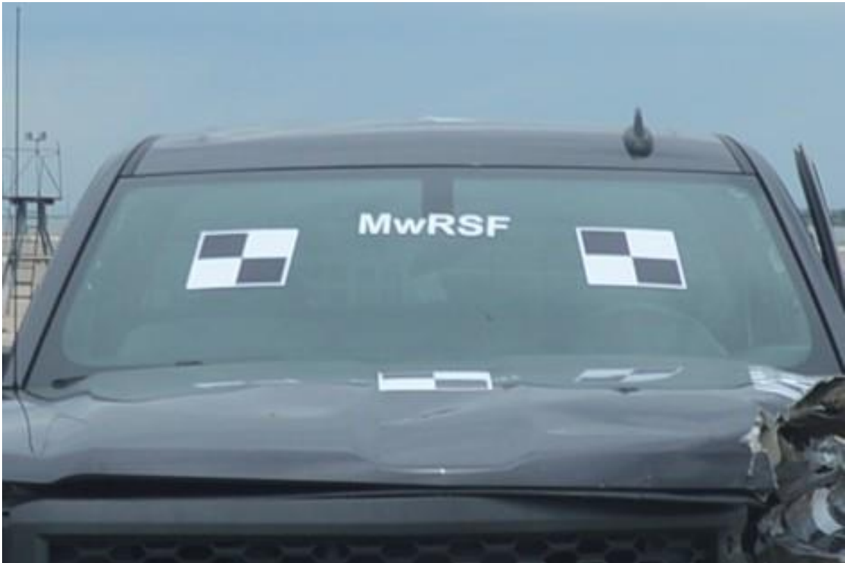
Figure 85. Windshield Damage (Pre- and Post-Test), Test No. NCBR-2
