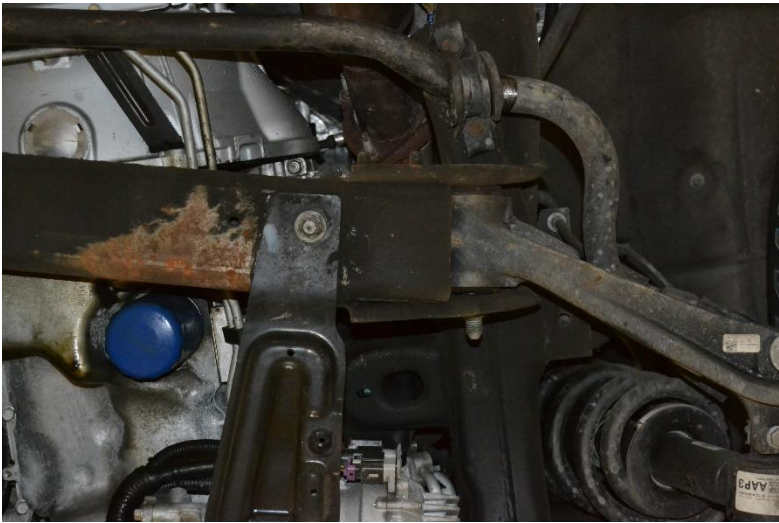
Figure 84. Undercarriage Damage, Test No. NCBR-2
