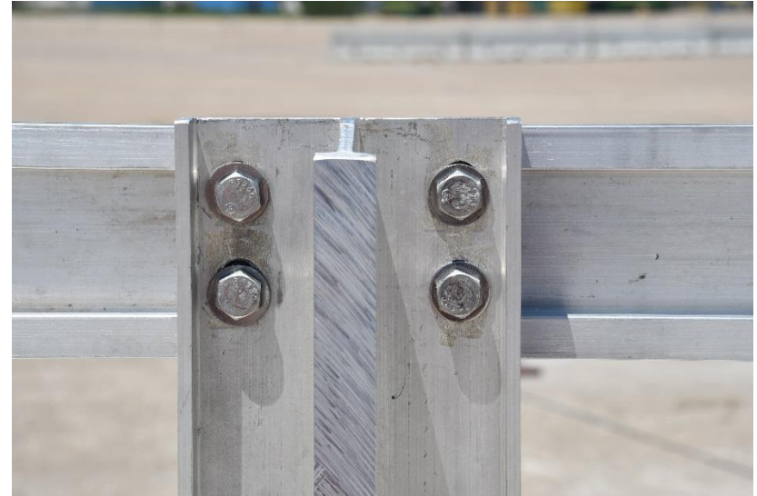
Figure 32. Post-to-Parapet and Post-to-Rail Attachment Details, Test Nos. NCBR-1 and NCBR-2
