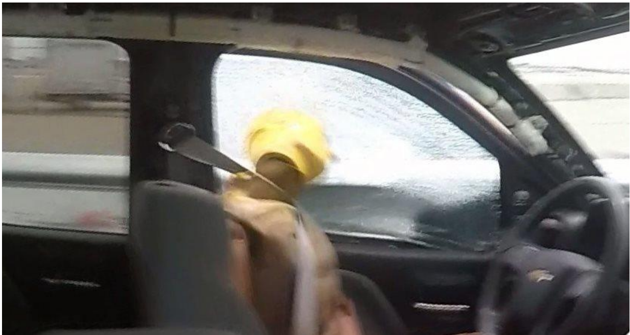
Figure 95. Maximum Occupant Head Protrusion, Test No. NCBR-2
