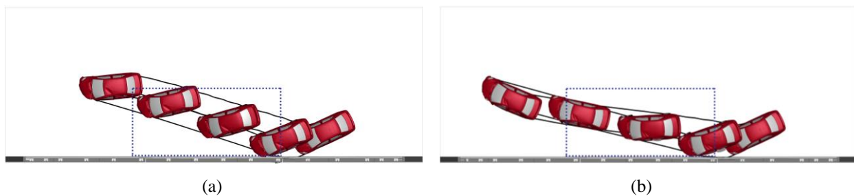
Figure 4.51: Vehicle trajectories of 2010 Toyota Yaris impacting 3BMR-2 under TL-3 conditions. (a) With expansion joint as reference; and (b) with the post as reference.
