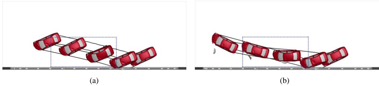
Figure 4.42: Vehicle trajectories of 2010 Toyota Yaris impacting 3BMR-1 under TL-3 conditions. (a) With expansion joint as reference; and (b) with the post as reference.
