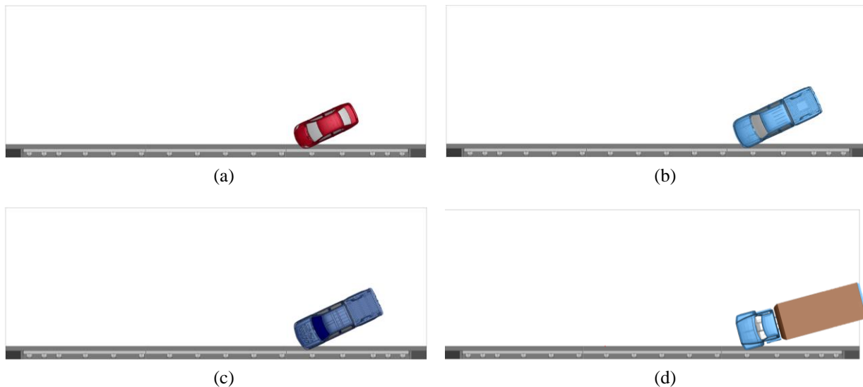
Figure 3.22: Full simulation models for the Oregon Rail using expansion joints as the reference points. (a) 2010 Toyota Yaris; (b) 2007 Chevy Silverado; (c) 2014 Chevy Silverado; and (d) 1996 Ford F800.
