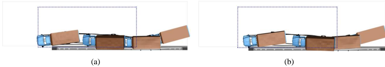
Figure 4.29: Vehicle trajectories of 1996 Ford F800 impacting the Oregon Rail. (a) With expansion joint as reference; and (b) with the post as reference.
