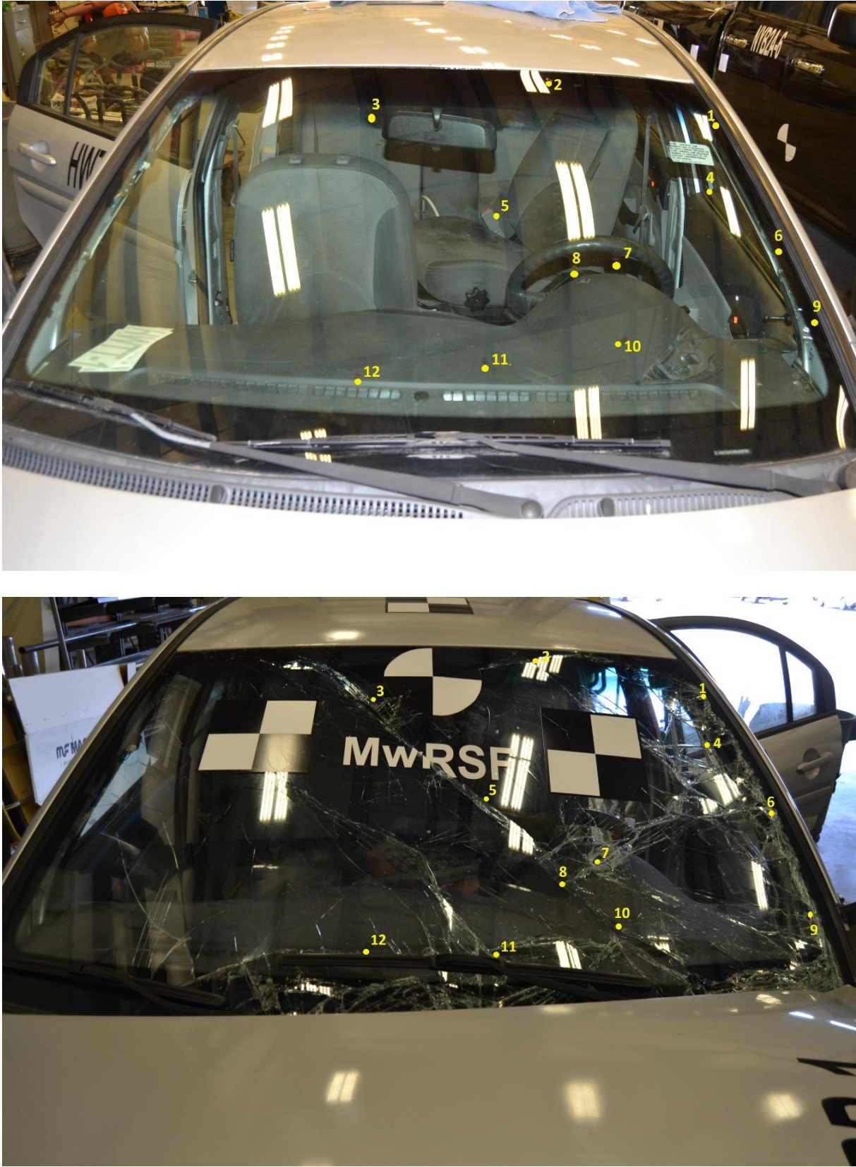
Figure 63. Windshield Damage (Pre- and Post-Test), Test No. NCBR-1
