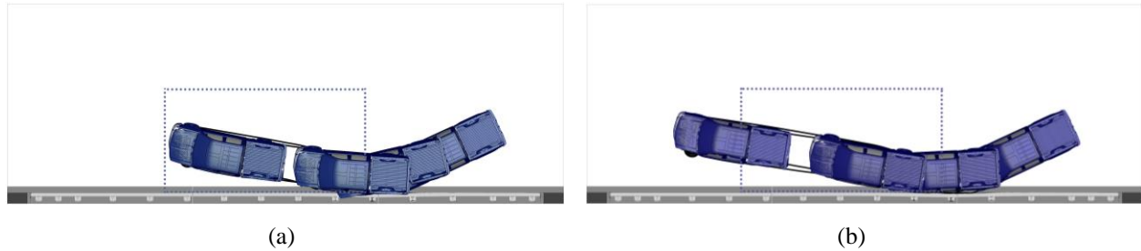
Figure 4.26: Vehicle trajectories of 2014 Chevy Silverado impacting the Oregon Rail. (a) With expansion joint as reference; and (b) with the post as reference.
