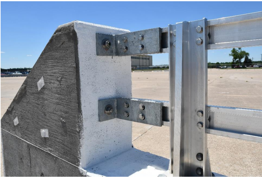
Figure 33. Rail End Anchorage Details, Test Nos. NCBR-1 and NCBR-2
