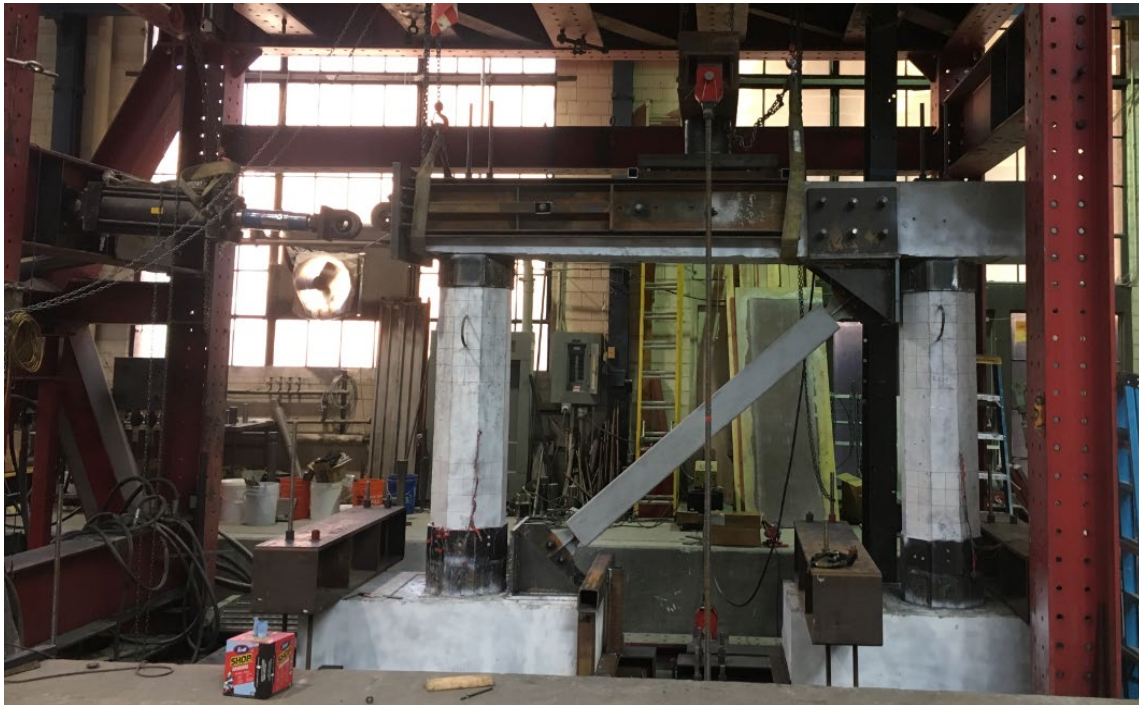
Figure 3.8 Experimental setup of PT-BRB Bent test
