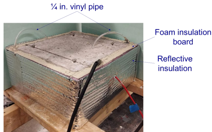
Figure 7-10. Insulated treated slab before exposure to 120° F at 25% RH
