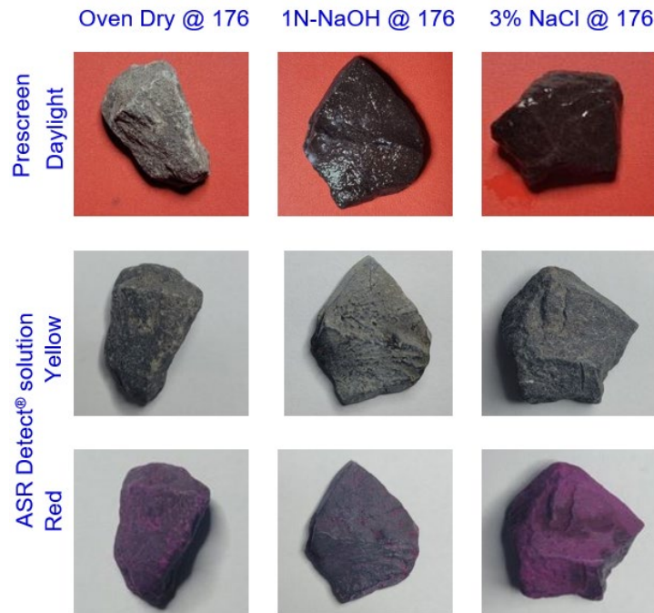
Figure 5-7. Observation of coarse aggregate (Spratt) stored under various exposure conditions and treated with ASR Detect®
