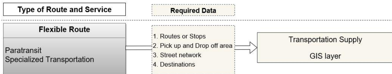
Figure 3-4. Conceptual Framework for Flexible Route Service GIS Layer
