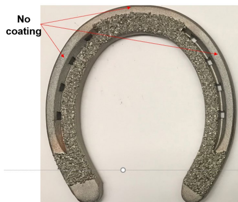
Figure 1. The Selected tungsten carbide coating design for horseshoes
