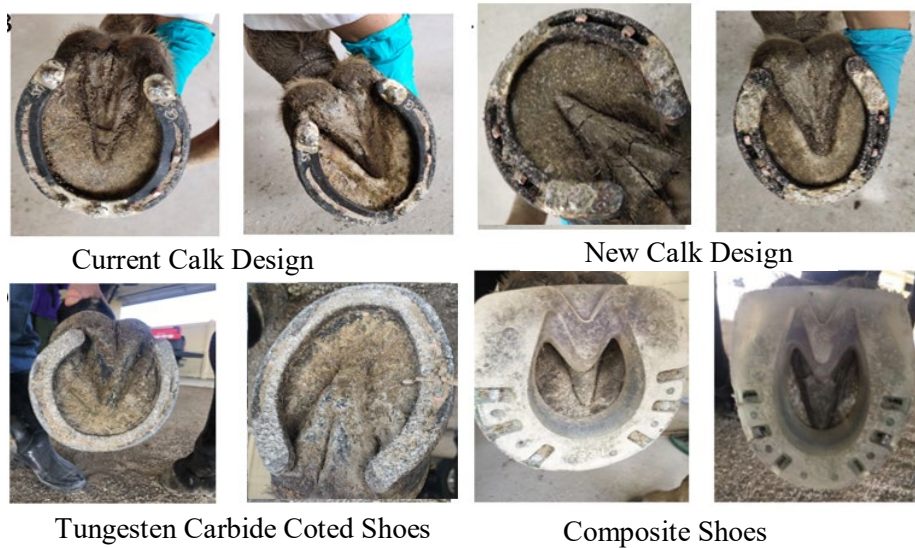
Figure 3. Pictures of different horseshoes tested in on fore (left) and hind (right) hoof
