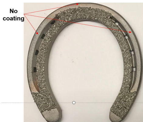
Figure B.3 The selected tungsten carbide coating design for horseshoes
