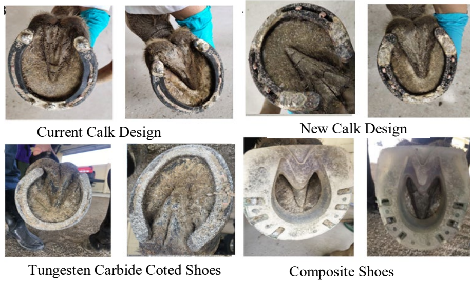
Figure B.7 Pictures of different horseshoes tested in on fore (left) and hind (right) hoof
