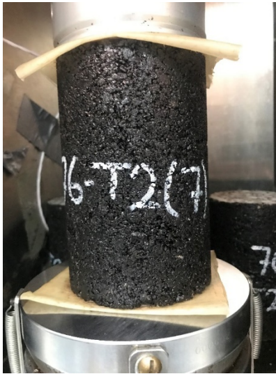
Figure A.1. Flow number test configuration
