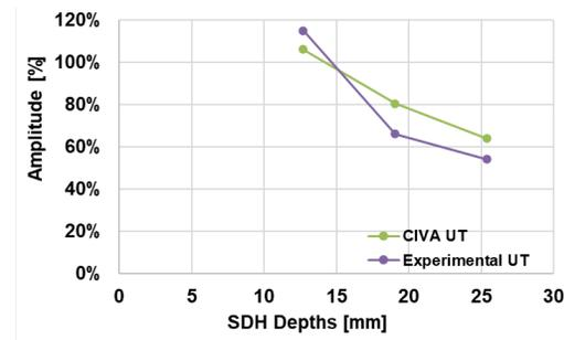
Figure 6. Maximum amplitude comparisons on SDHs in rail using 70° SW
