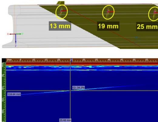
Figure 7. B-scan result for SDHs in rail: (top) CIVA-UT, (bottom) experimental UT
