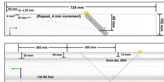
Figure 2. Drawings of samples with SDHs for model validation: (top) steel block, (bottom) 136RE rail
