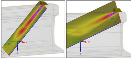
Figure 4. Contact ultrasonic SW beam field response in 136RE rail: (left) 45°, (right) 70°
