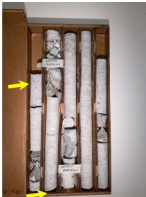
Figure 120. Photo. Cores obtained from coring test drilled shaft #2 showing the start and end of a defect between depths of 13.5 and 14.0 ft (see yellow arrows).
