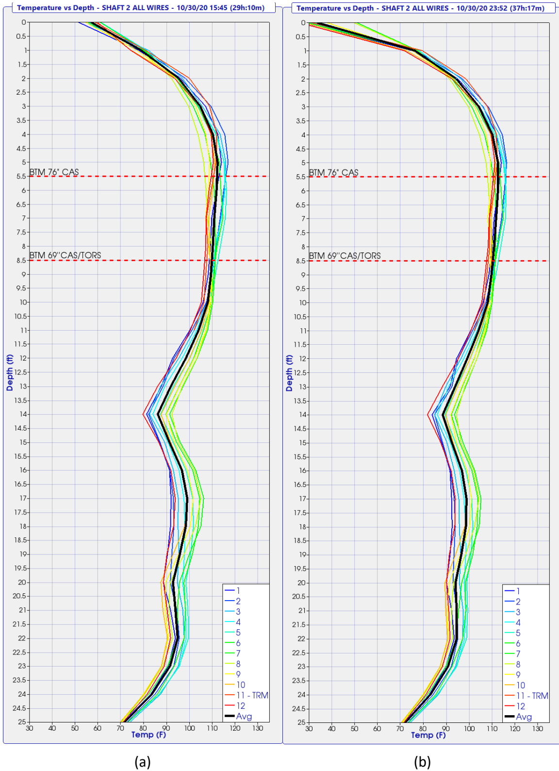
Figure 98. Graph. Temperature versus depth profile for all the 12 wires in test drilled shaft #2: (a) at 29h 10m, and (b) at 37h 17m (peak) after concrete placement.
