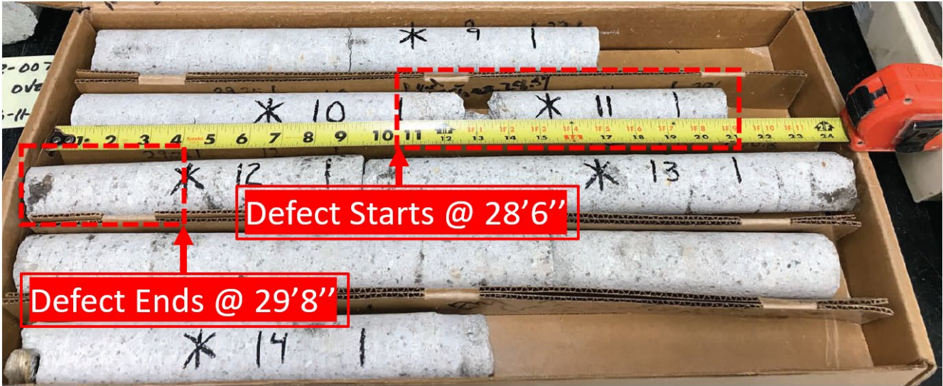
Figure 155. Photo. Photograph showing the start of defect at 28 ft 6 in. depth and end of defect at 29 ft 8 in. depth from core #1 of test drilled shaft #3.
