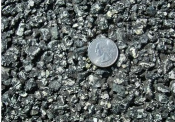
Figure 9. Surface Texture of PFC.
