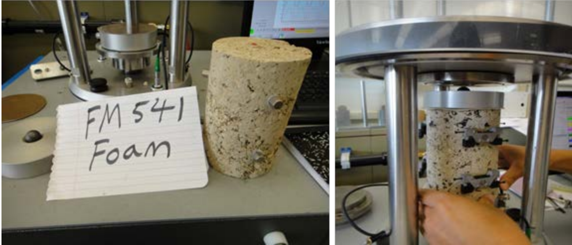
Figure 20. Dynamic Modulus Testing of Asphalt Stabilized Material.
