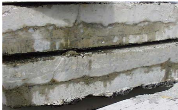
Figure 132. Formation of Deep Delamination.
