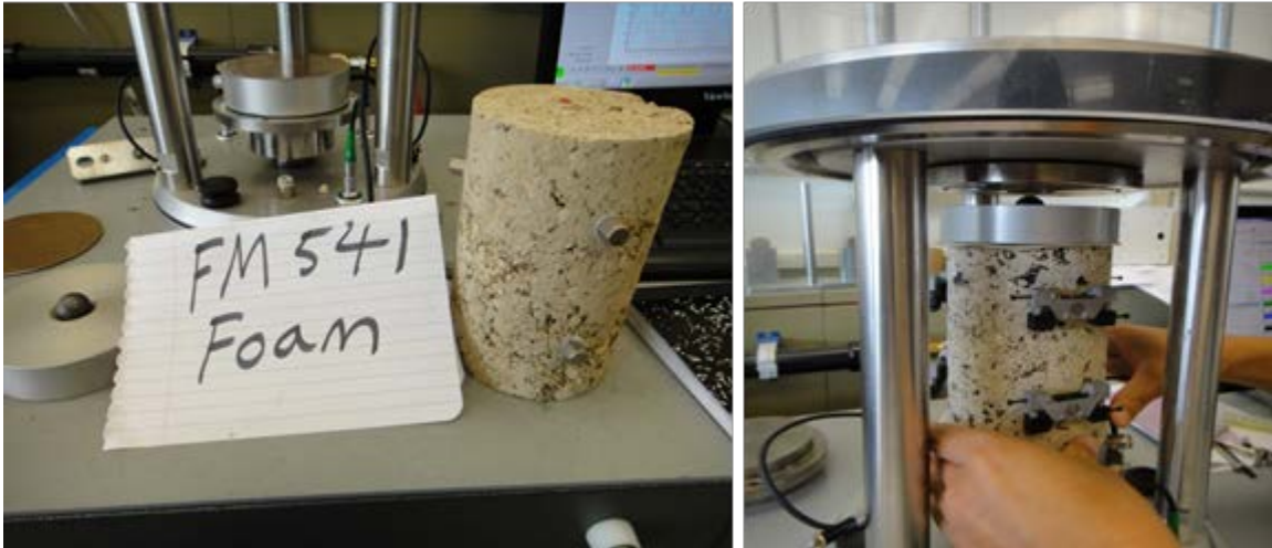
Figure 27. Dynamic Modulus Testing of Stabilized Materials (FDR).
