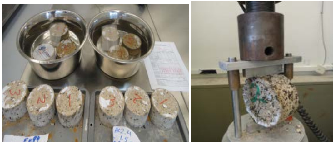
Figure 21. Samples Taken during the Moisture Conditioning and the IDT Test.
