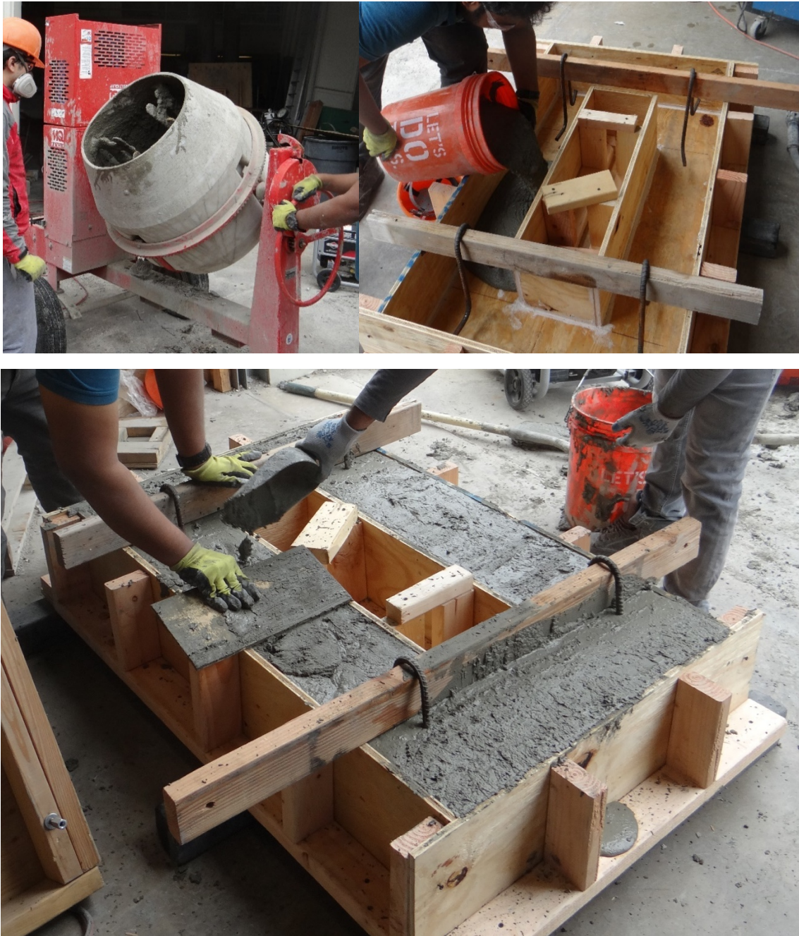
Figure 28. In-lab concrete mixing is shown in top photo and casting for the outer hollow slab is shown in the bottom photo.
