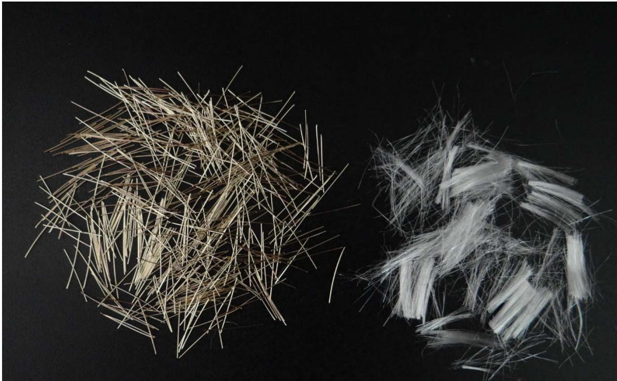
Figure 12. Micro steel fiber (left) and ultra-high molecular weight polyethylene fiber (right).
