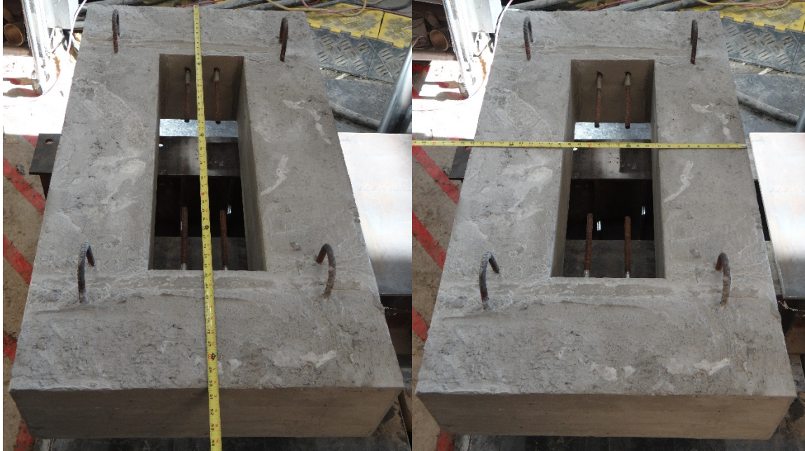
Figure 31. Outer hollow slab showing embedded rebar location.
