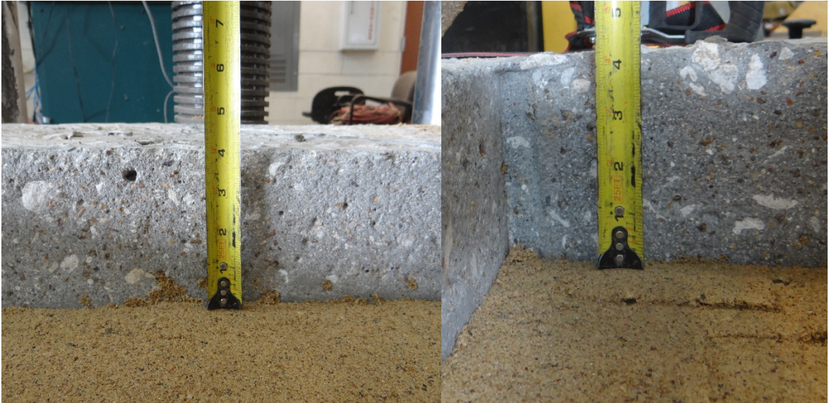
Figure 37. The 4-inch casting surface level obtained after placement and compaction of sand in the hollow portion.
