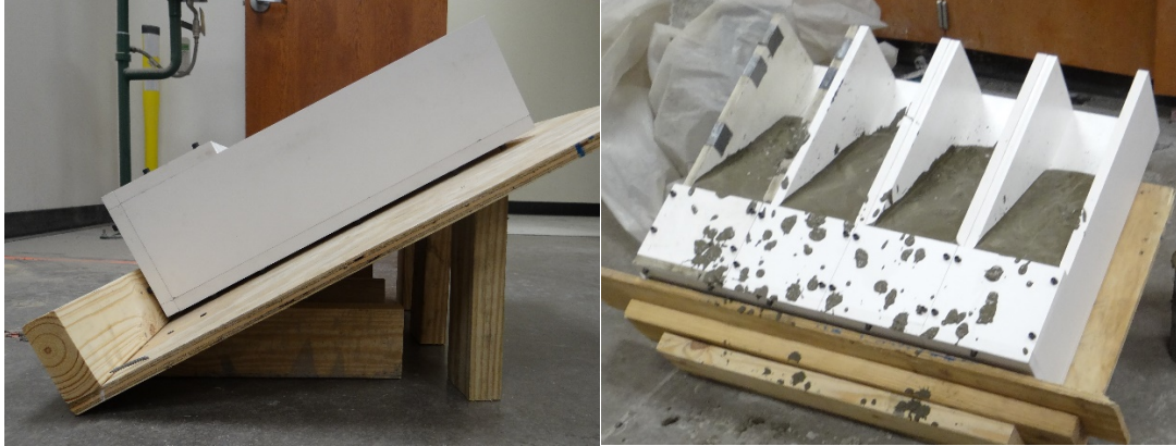
Figure 14. Mold placement and casting for bottom half of slant shear specimen.
