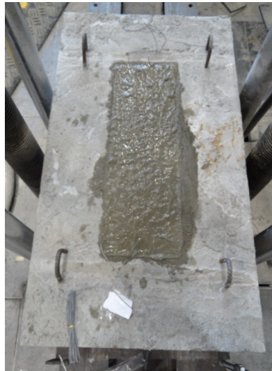
Figure 34. Cast in place PC punch test specimen.
