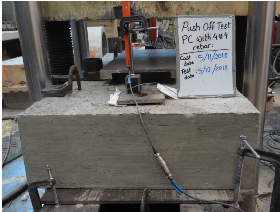
Figure 58. Punch test setup for PC specimen with dowel bars.
