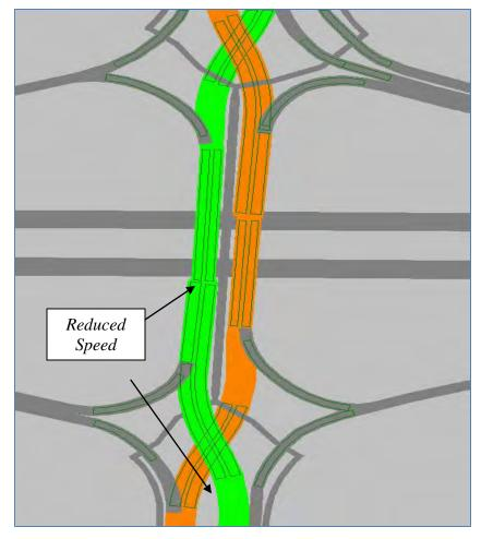
travel speeds for the diamond interchange models were higher than those measured in the field. It should be noted, however, the field travel time results reflect only 7 to 8 runs. The VISSIM results reflect several hundred to as many as a thousand vehicles traveling through the corridor and therefore include vehicles that may have been stopped at a red light. Travel time runs along arterials (especially short sections such as this study area) are highly sensitive to signal timing and phasing.
