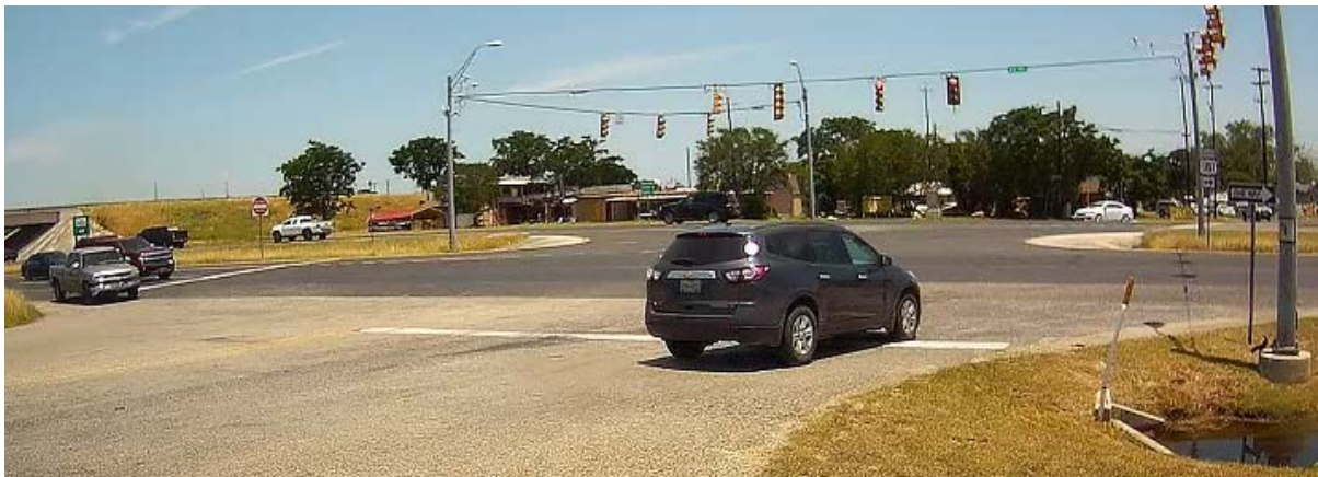
Figure 27. Right turn traffic (left side) using the shoulder as a turn bay.
