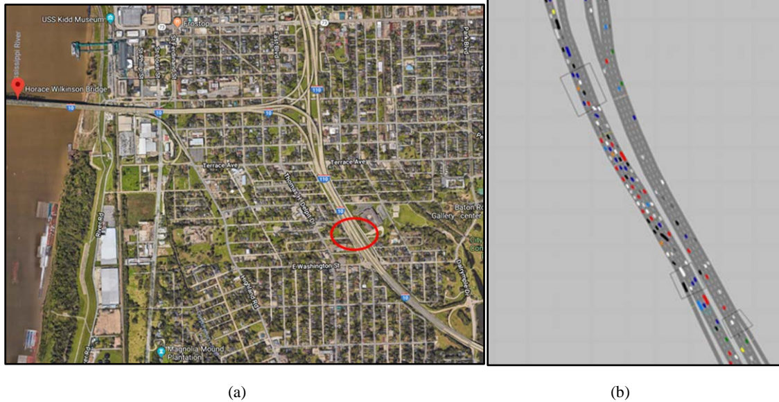
Figure 18. (a) Routing of I-10 EB traffic from Washington Street Exit to Dalrymple Drive Exit and (b) Congestion created by lane changes at Washington Street.
