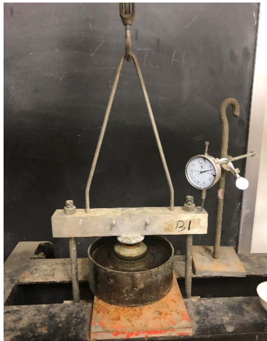
Figure 4. The 1-D swell test being conducted in consolidometer.
