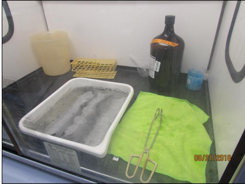
Figure 3-11: Hydrochloric Acid Bath in Ventilated Fume Hood
