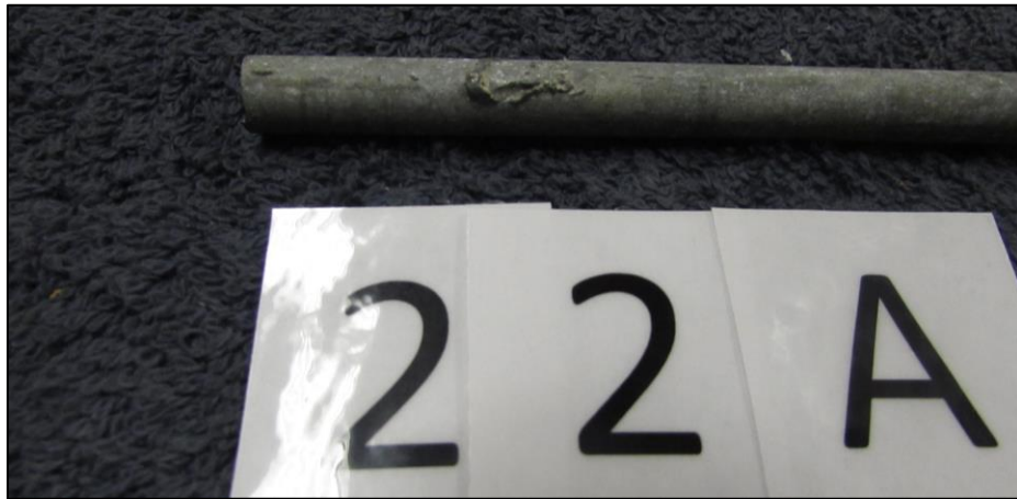
Figure 3-10: Zinc Coating Surface Abnormality
