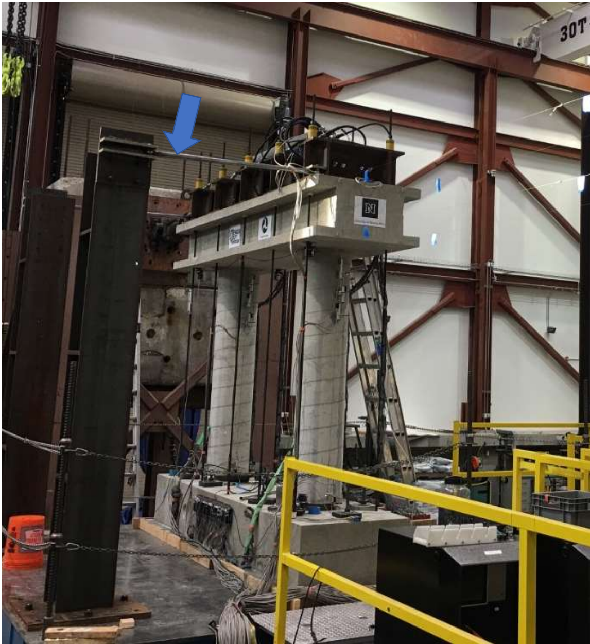
Figure 4.13 Connection of a steel column to load transfer beam using a compression rod
