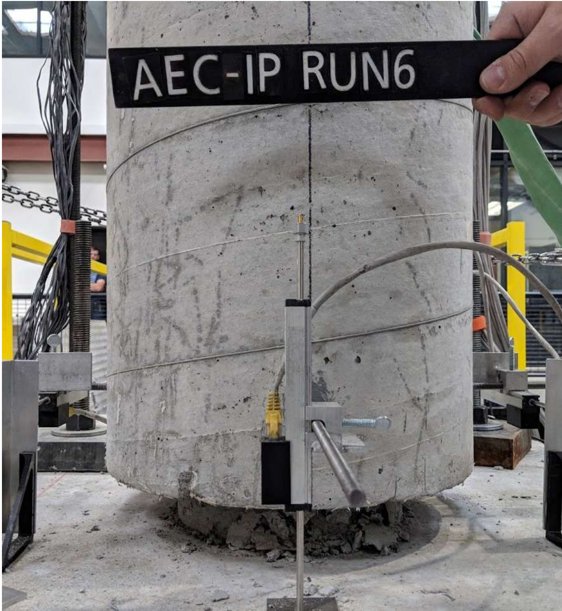
Figure 5.35 Run 6 – Progression of spalling in hinge (CIP – S face)
