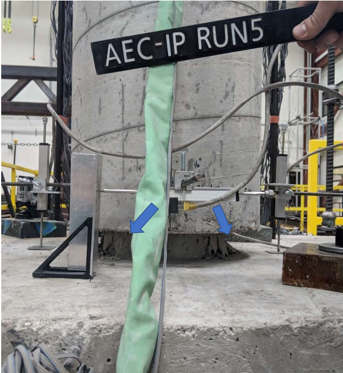
Figure 5.29 Run 5 – Major spalling of hinge (CIP – E face)
