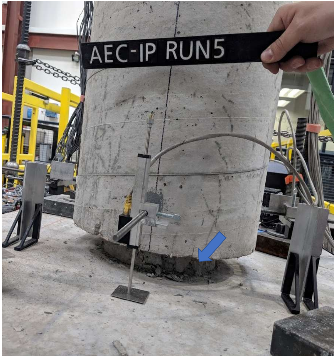
Figure 5.30 Run 5 – Major spalling of hinge concrete (CIP – S face)
