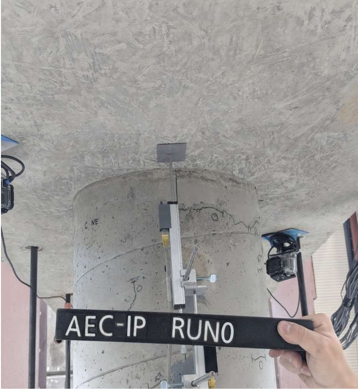
Figure 5.23 Run 0 – Cracks marked before testing (CIP – N face)
