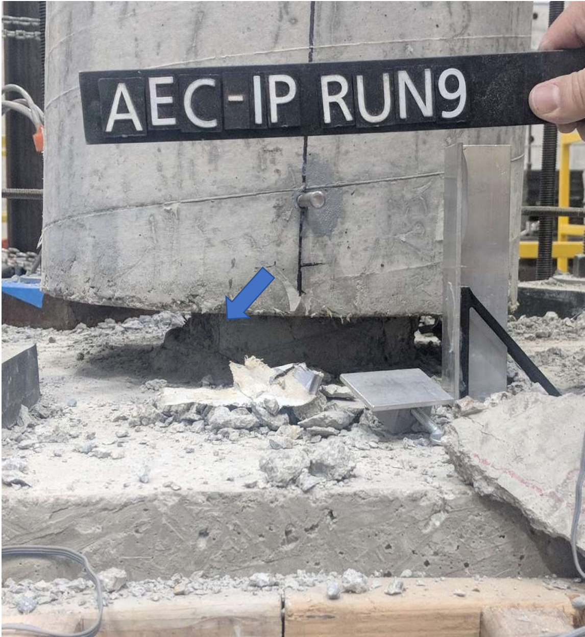
Figure 5.43 Run 9 – Progression of spalling into two-way hinge core (CIP – E face)
