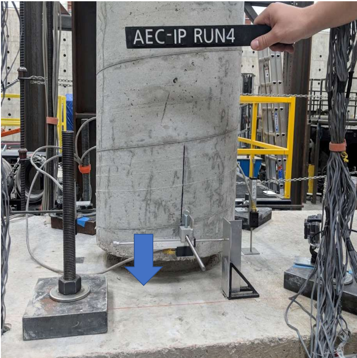
Figure 5.3 Run 4 - Initiation of two-way hinge spalling (ABC - W face)
