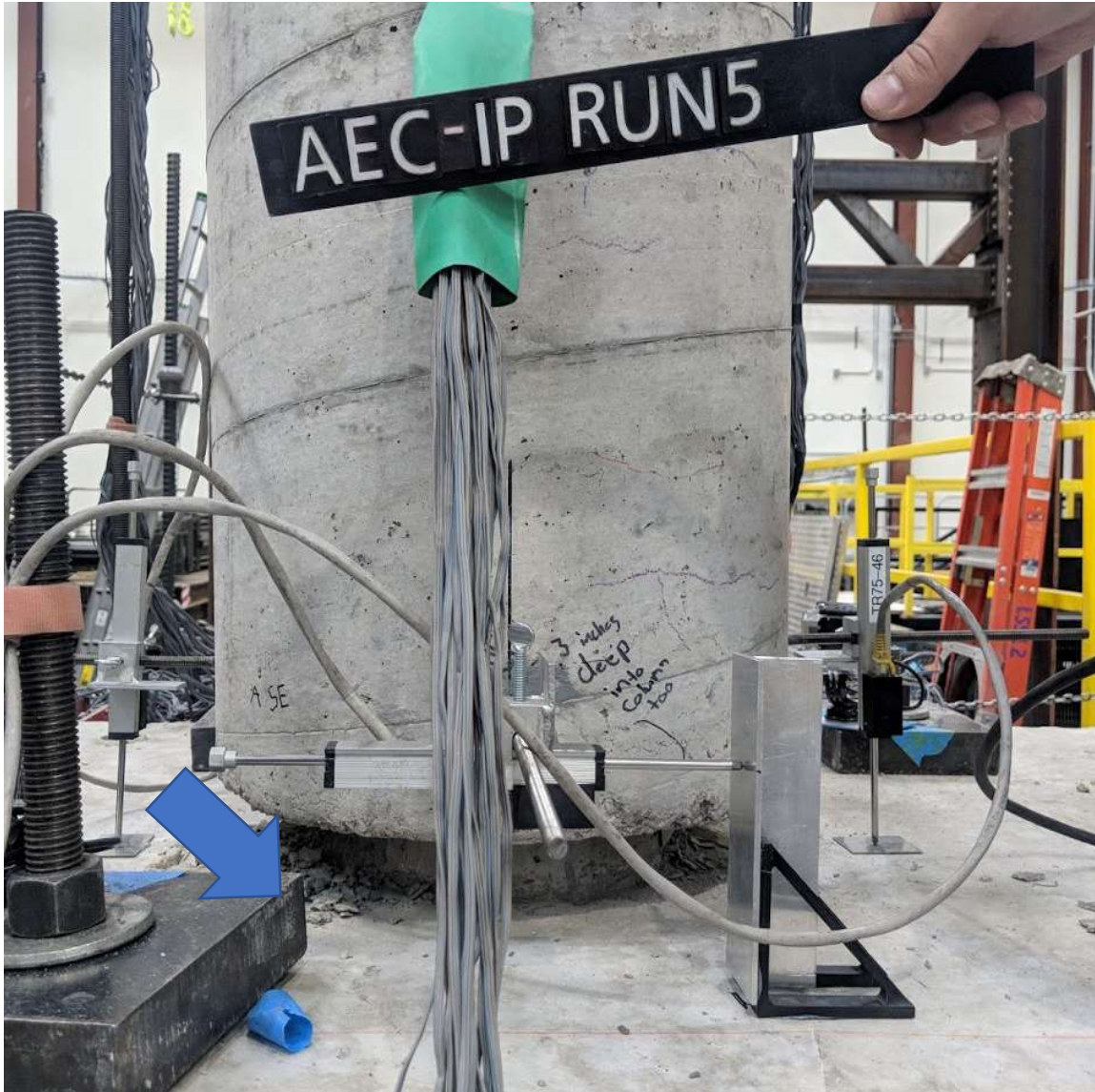
Figure 5.4 Run 5 – Progression of two-way hinge spalling (ABC - E face)
