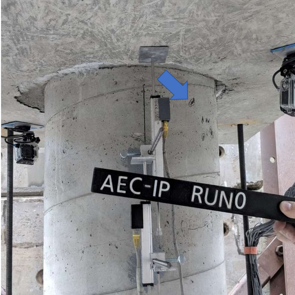
Figure 5.2 Run 0 - Voids on column before start of testing (ABC - N face)
