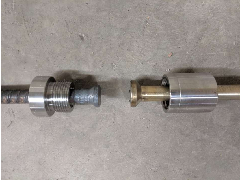
Figure 2.9 HRC connection between rebar and CAM bar
