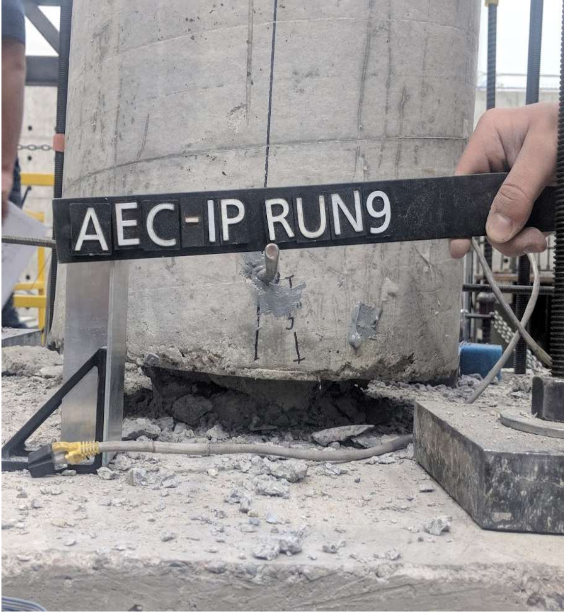
Figure 5.19 Run 9 – Severe spalling of two-way hinge (ABC – W face)
