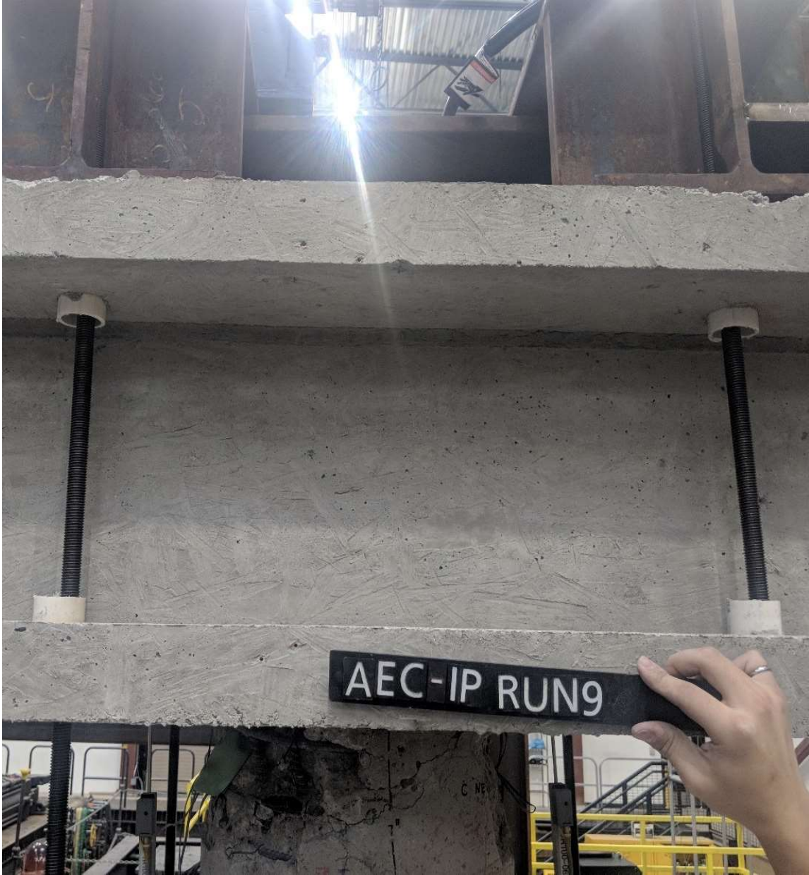
Figure 5.47 Run 9 – Absence of cracks on north column-cap joint (CIP – E face)
