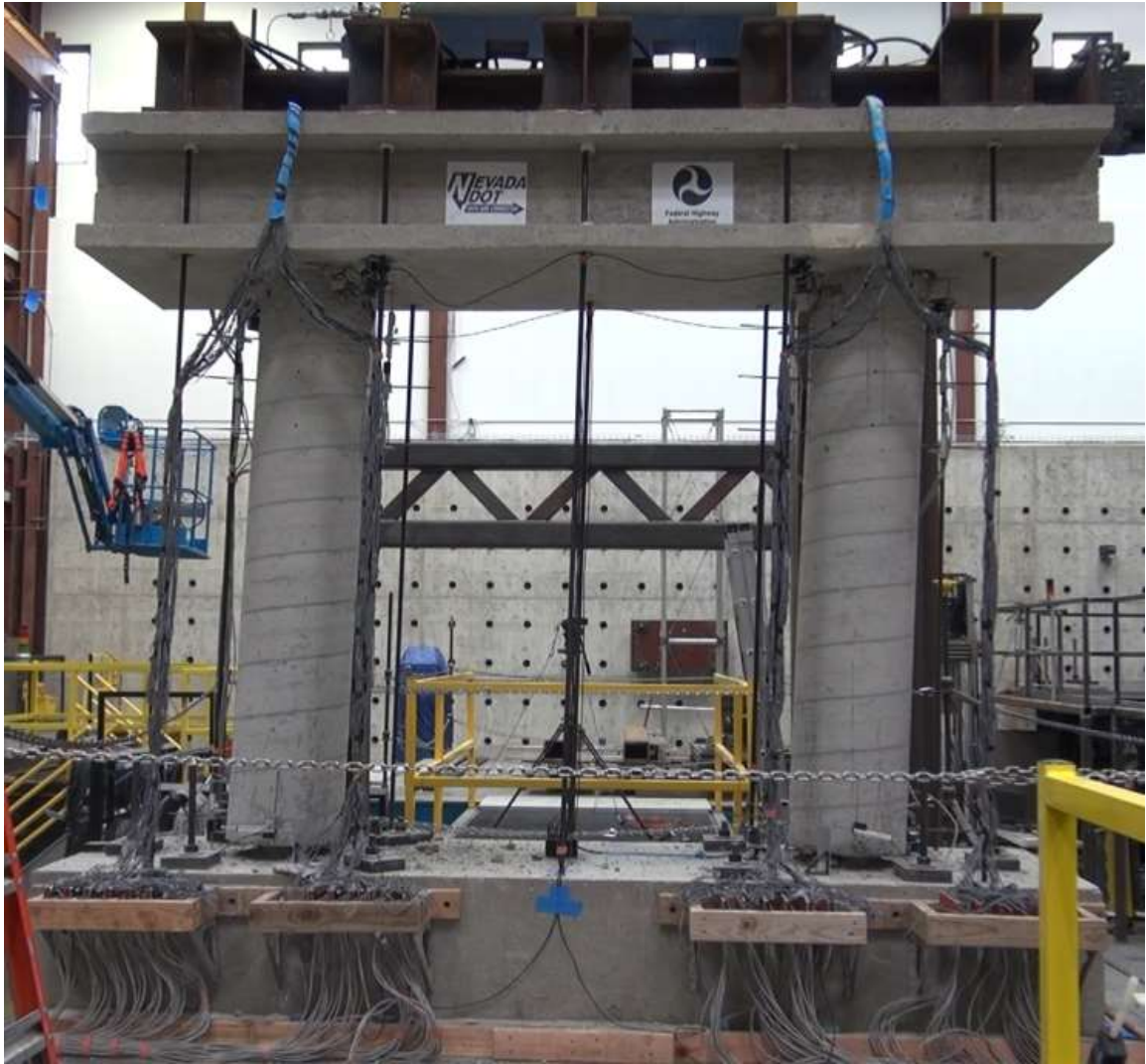
Figure 5.20 Run 9 – Overview of specimen after final ground motion (ABC – W face)
