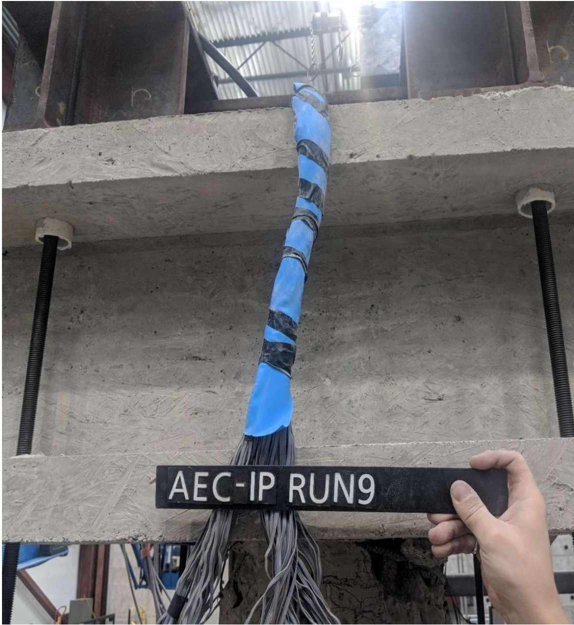
Figure 5.48 Run 9 – Absence of cracks on north column-cap joint (CIP – W face)
