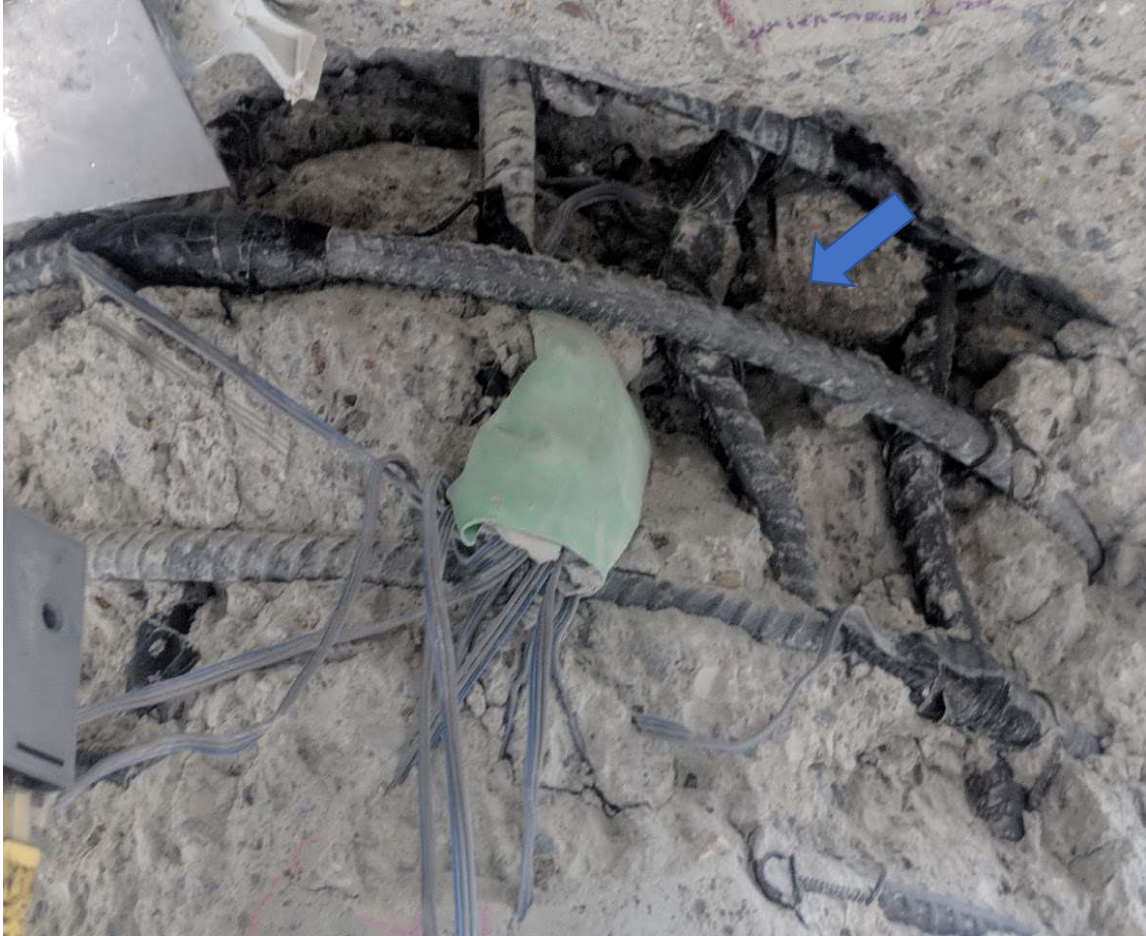
Figure 5.46 Run 9 – Close up of damage on southern face and deformed bars (CIP – S face)
