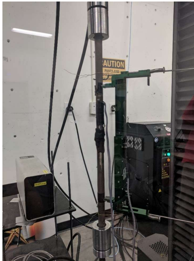
Figure 4.4 CAM bar test setup
