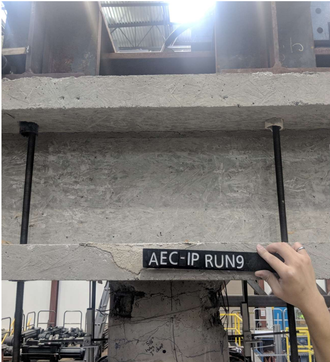
Figure 5.21 Run 9 – Absence of cracks on south column-cap joint (ABC – E face)
