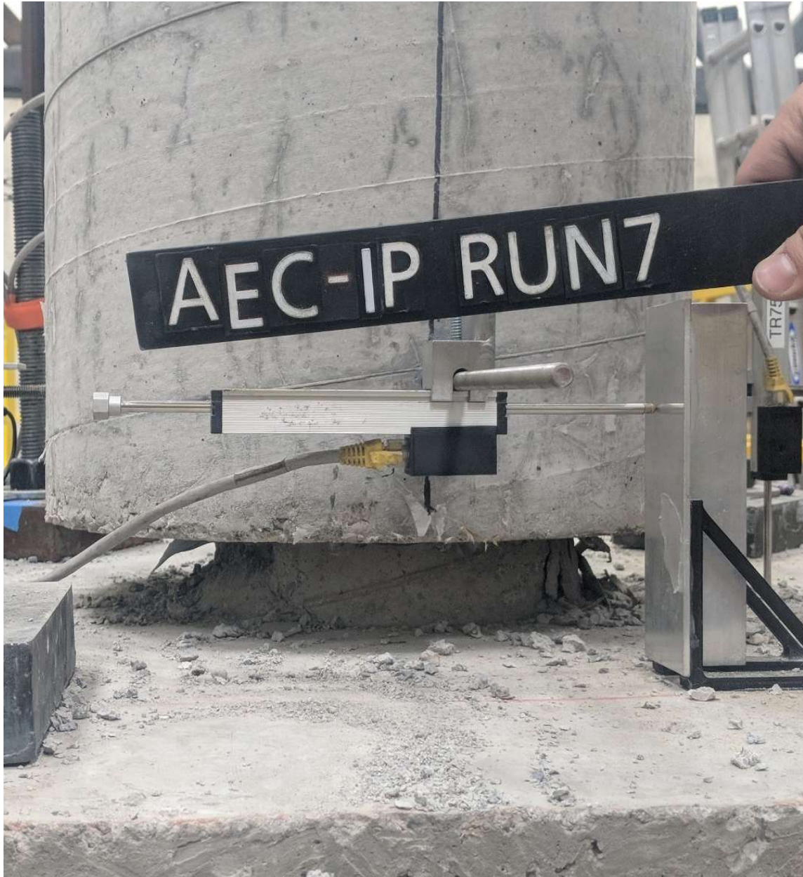
Figure 5.38 Run 7 – Debris removed from hinge (CIP – W face)
