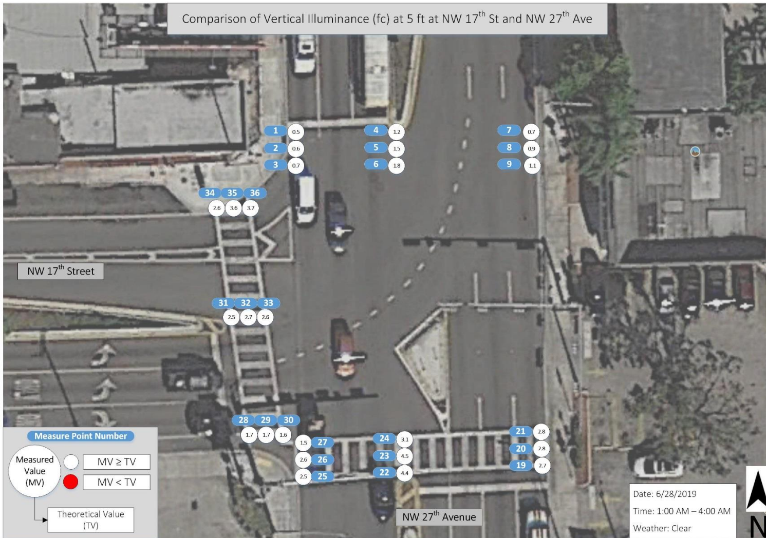
Figure 50. Comparison of Vertical Illuminance at NW 17 th St and NW 27 th Ave
