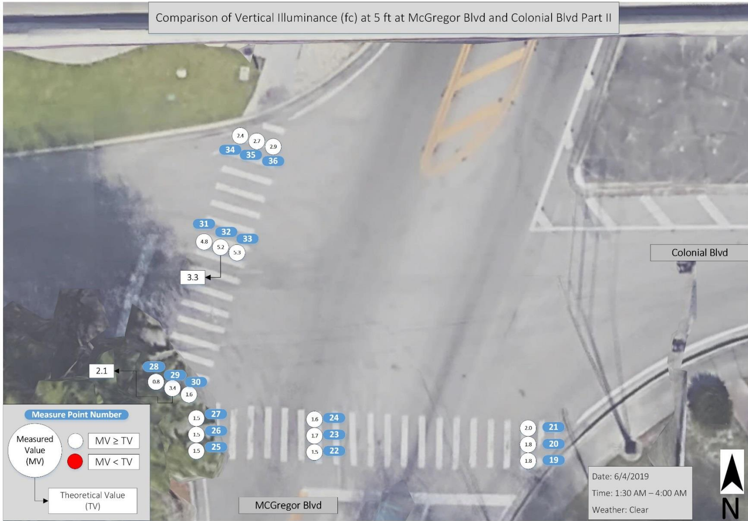
Figure 18. Comparison of Vertical Illuminance at McGregor Blvd and Colonial Blvd (South Side)
