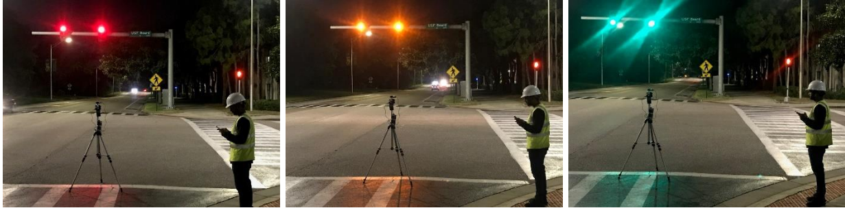
Figure 6. Test of Signal Light Influence on Crosswalk
