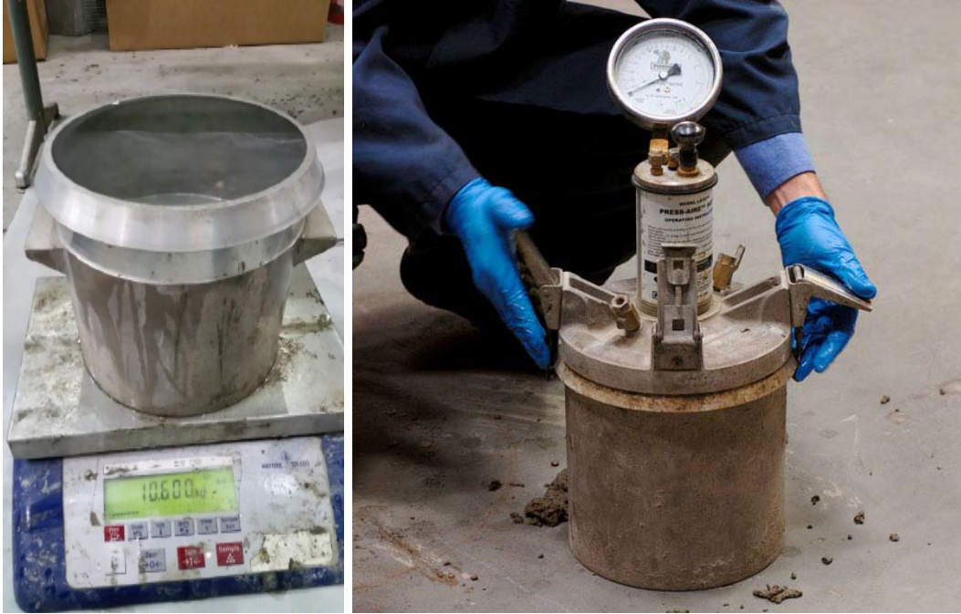
(a) Gravimetric Air Content From (Shalan 2016) (b) Pressure Air Content From (Shalan, 2016)
