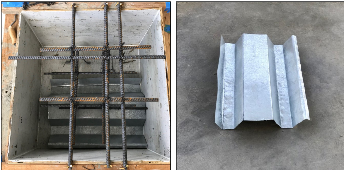
Figure 48. Photo. Bridge Deck Sample Image Before Casting and SIP Form
