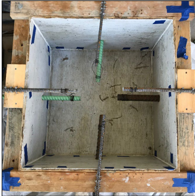
Figure 46. Photo. Dowel Bar Sample Image Before Casting
