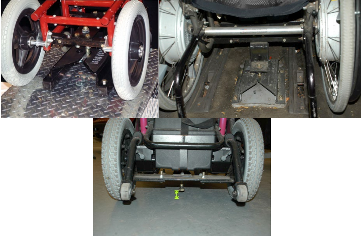
Figure 1. Examples of wheelchairs engaged with docking systems mounted to vehicle floors (upper left and right) and example of mating hardware with low ground clearance (lower center)
