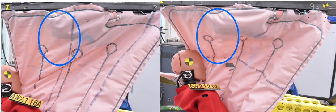
Figure D-3. Comparison of head contact location between AW2116 change test comparison (left) and AW2120 (right)
