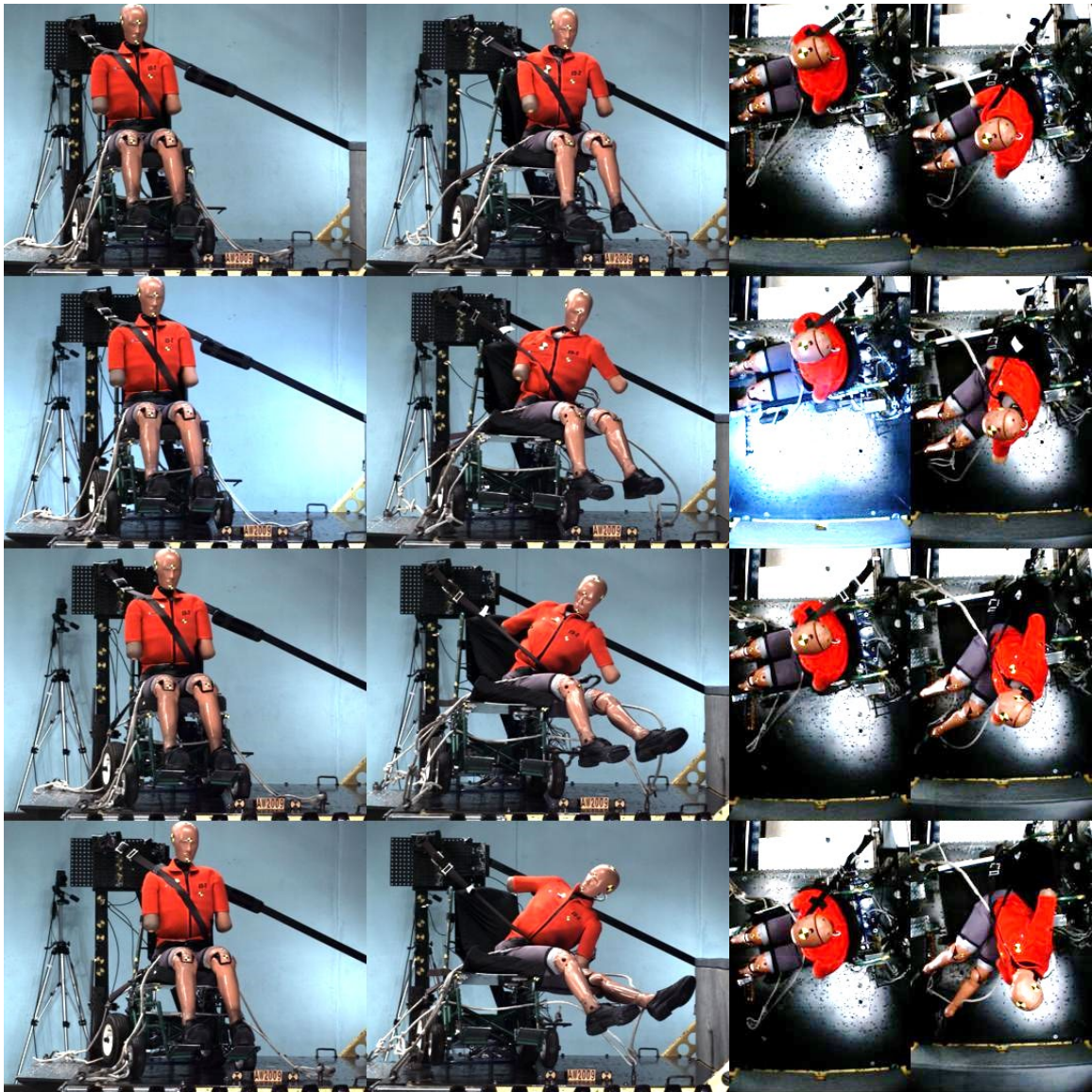
Figure C-13. Right side and oblique camera views every 20 ms for test AW2009, baseline with UDIG
