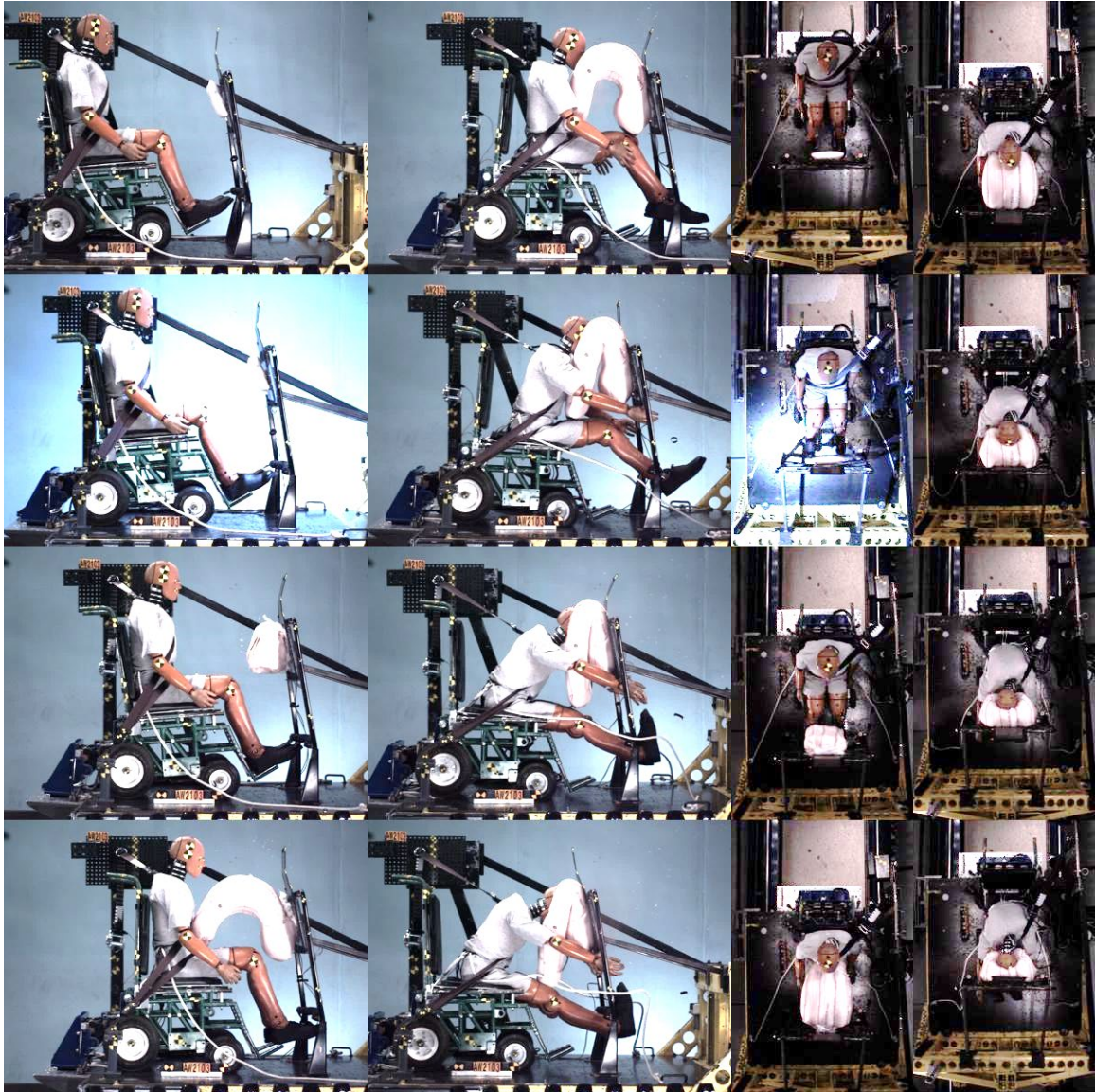
Figure C-3. Right side and overhead camera views every 20 ms for test AW2103
