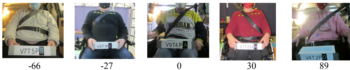
Figure 104. Examples of range of shoulder belt fit scores (mm)
