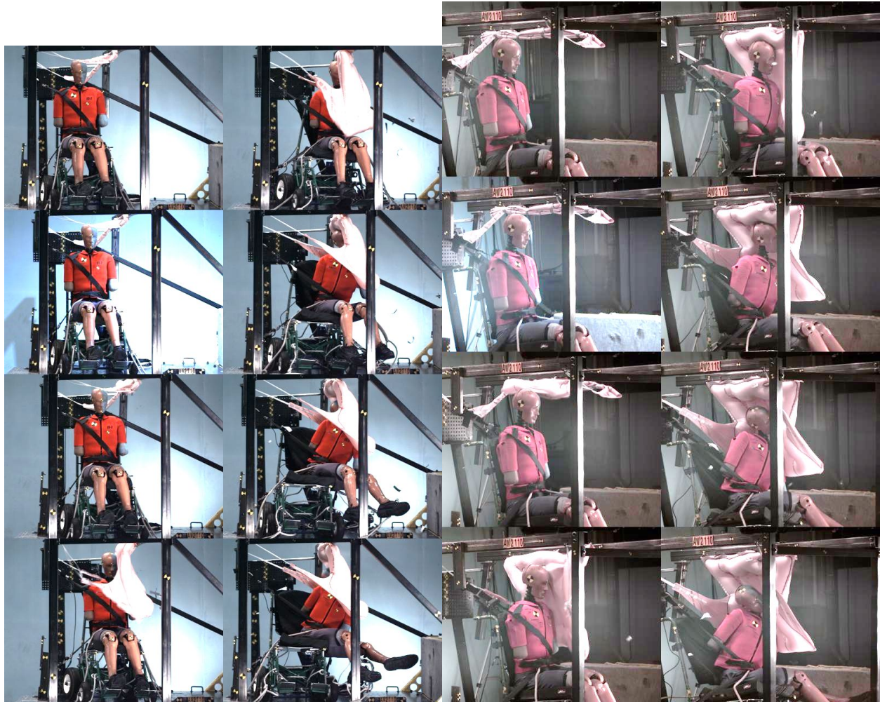
Figure C-16. Right side and oblique camera views every 20 ms for test AW2110
