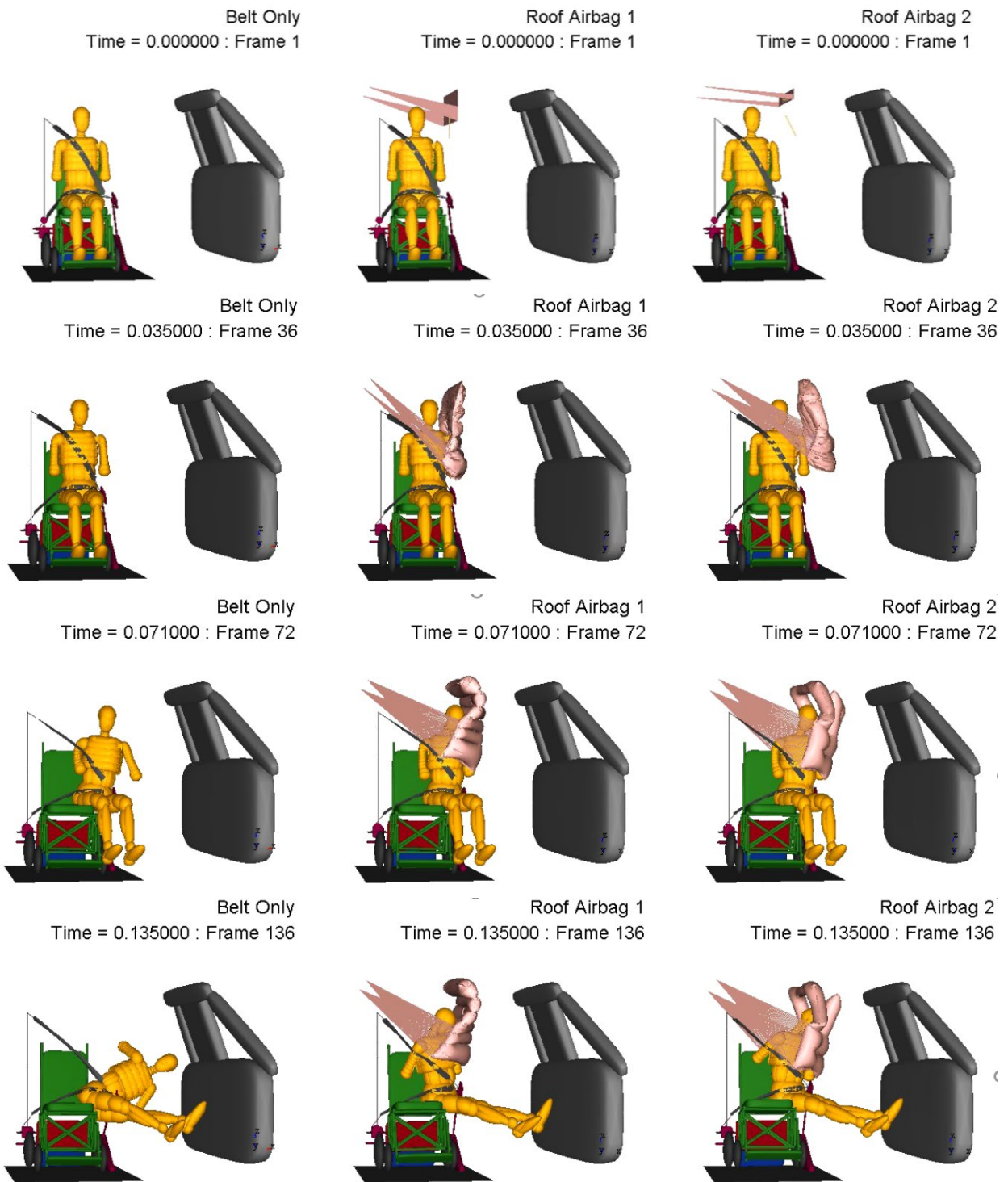
Figure 56. Comparison of kinematics in far-side impact for belt only (left), CATCH 1 design (middle), and CATCH 2 design (right)
