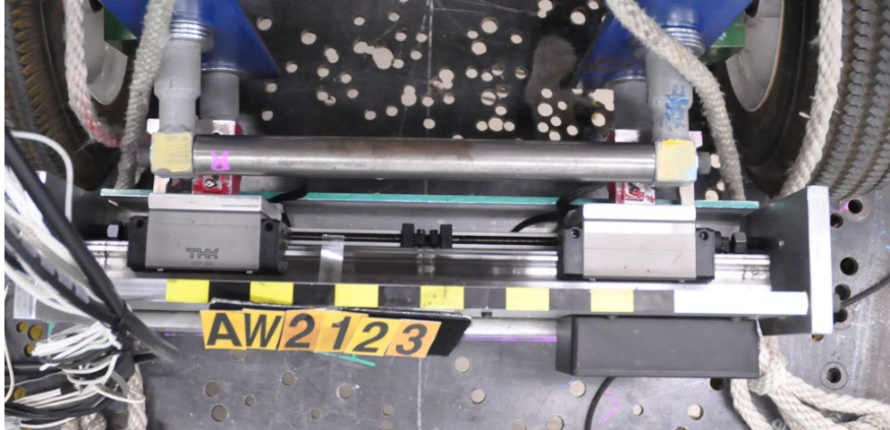
Figure D-11. Top view of UDIG anchors with new hook components
