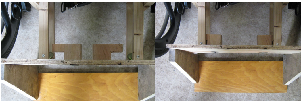
Figure 78. Mockup of UDIG anchorages before (left) and after (right) engaging UDIG attachments on manual wheelchair
