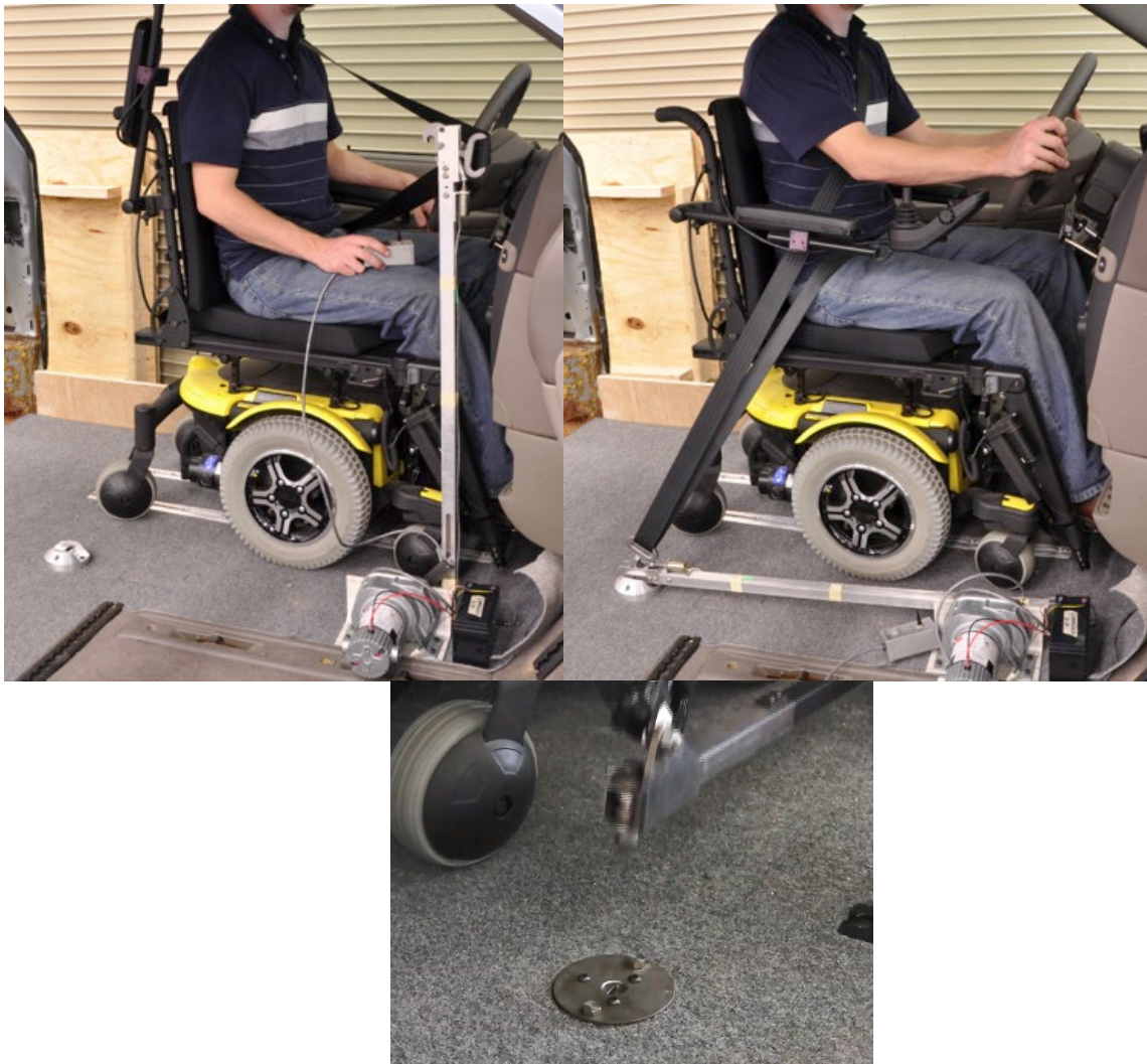
Figure 24. Prototype UMTRI belt-donning system before (left) and after (right) deployment; recessed floor pocket (bottom)
