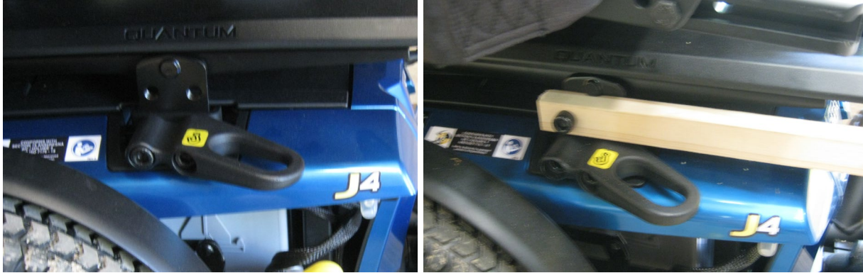
Figure 71. Connecting UDIG attachments near tiedown securement point on power wheelchair
