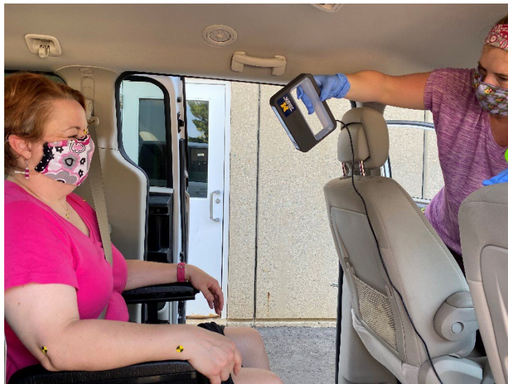
Figure 101. Measuring volunteer belt fit with remote scanner instead of FARO arm
