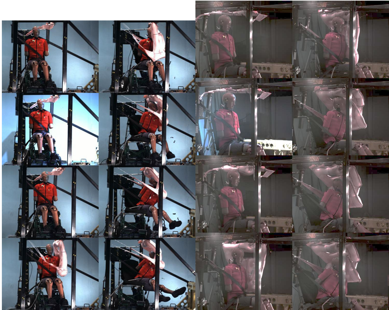
Figure C-18. Right side and oblique camera views every 20 ms for test AW2117
