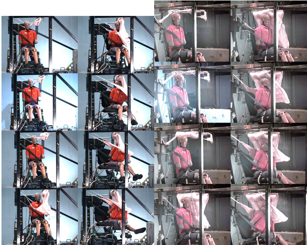
Figure C-15. Right side and oblique camera views every 20 ms for test AW2108
