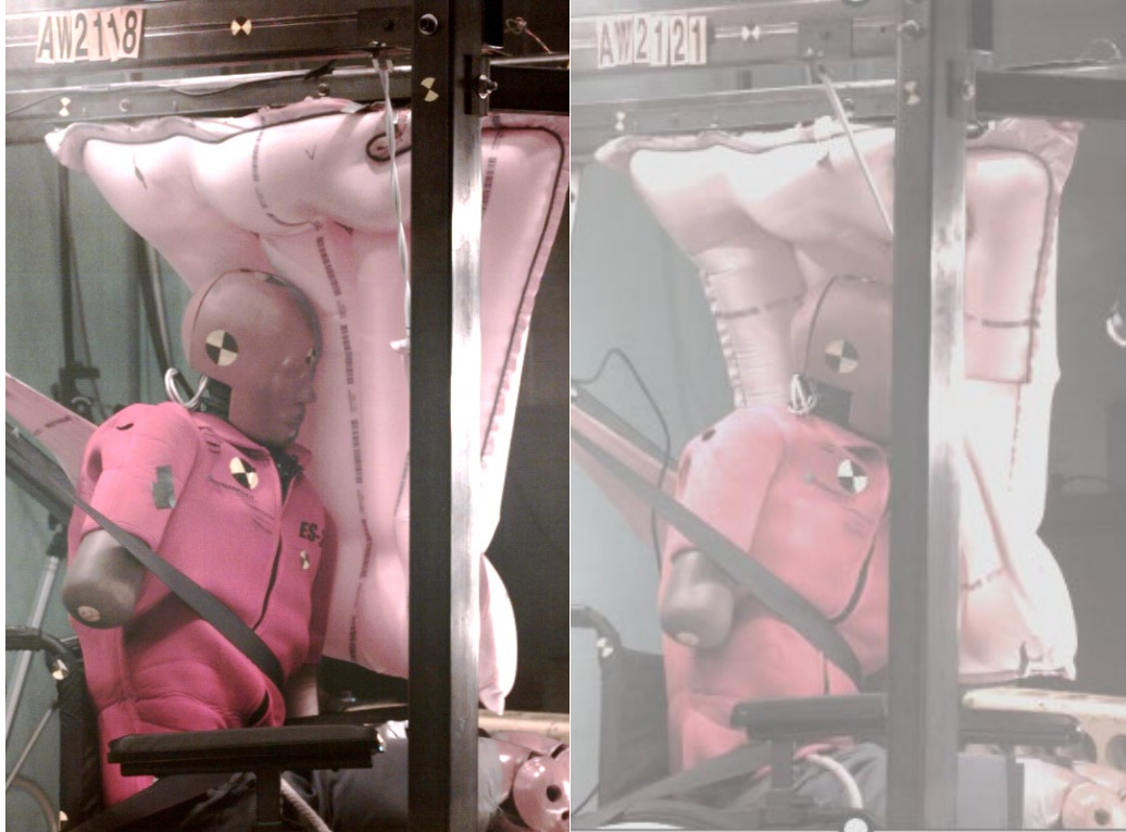
Figure D-5. Comparison of head contact points in manual chair in original and shifted locations
