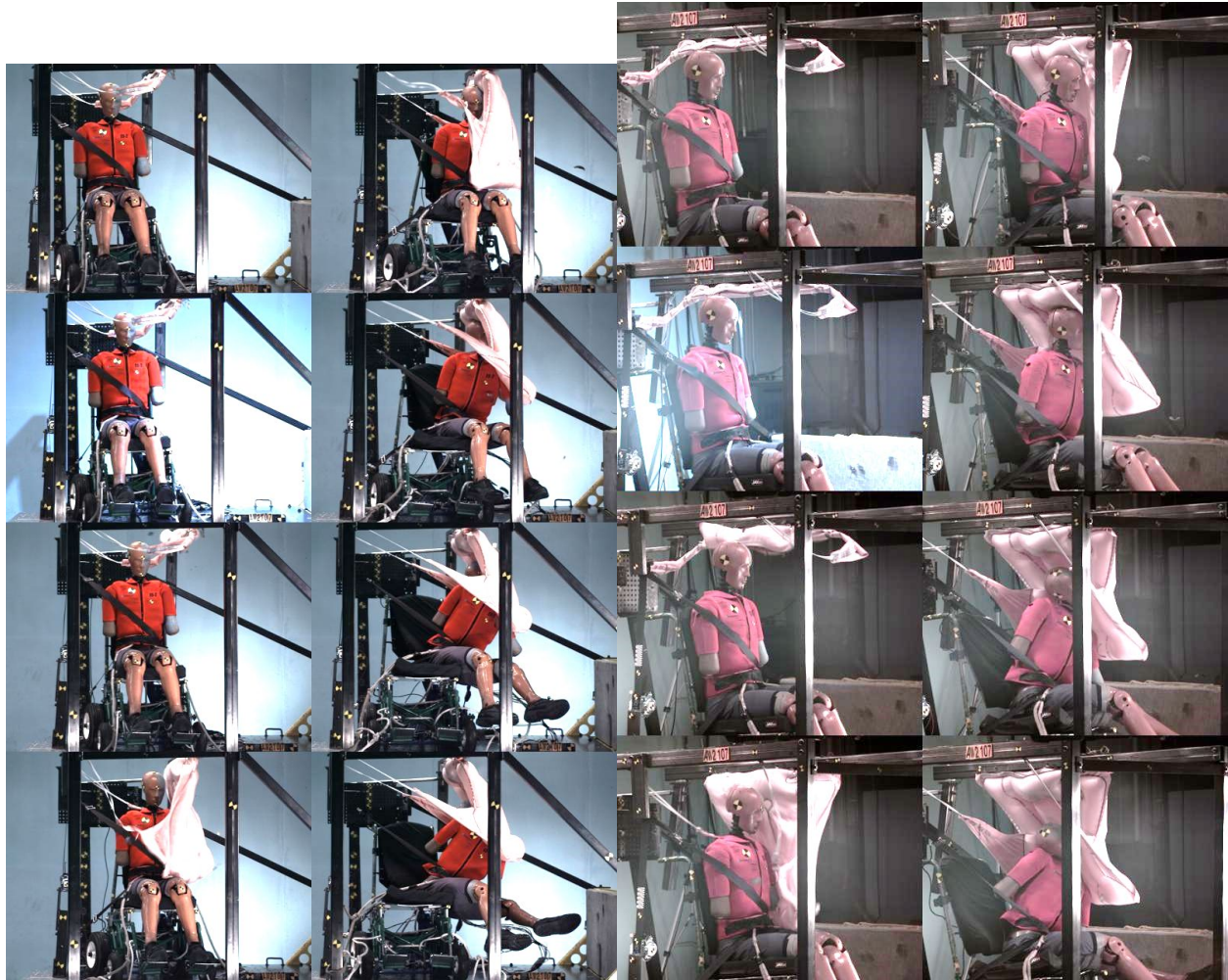
Figure C-14. Right side and oblique camera views every 20 ms for test AW2107
