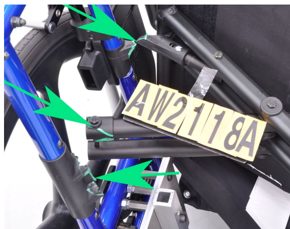
Figure 133. Damage to manual wheelchair during test AW2118
