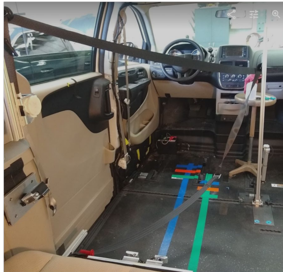
Figure 90. Duct tape used to mark centerlines and space 48", 54", and 60" forward of the UDIG anchorages
