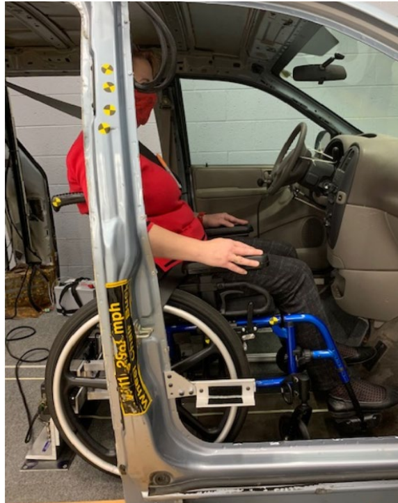
Figure 93. For current vehicle configurations, a right-front position that allows the required 48" long space for a wheelchair places the UDIG well behind the B-pillar
