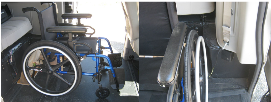
Figure 88. Manual wheelchair and UDIG anchorages in Braun vehicle; lateral location limited by wheel well
