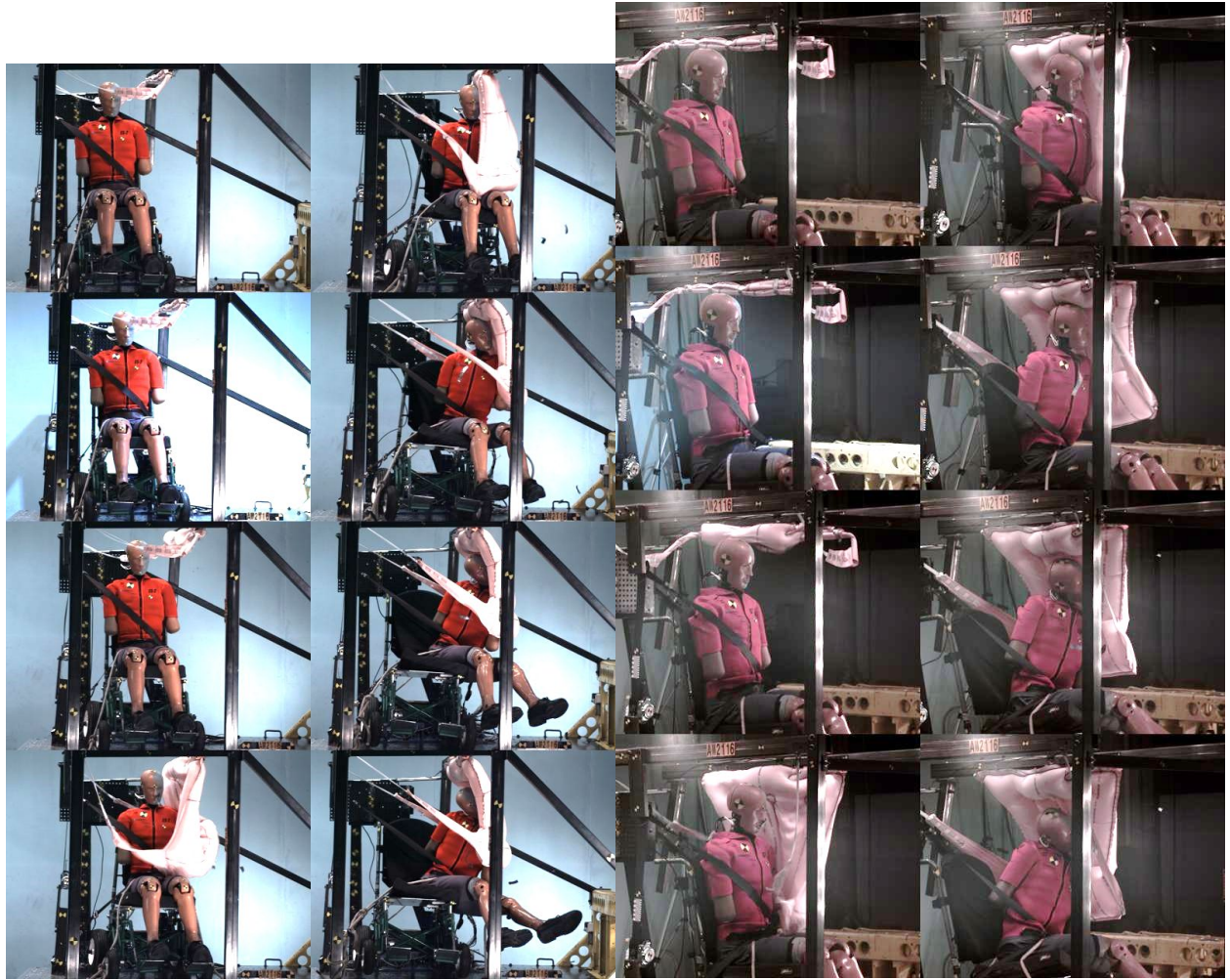
Figure C-17. Right side and oblique camera views every 20 ms for test AW2116
