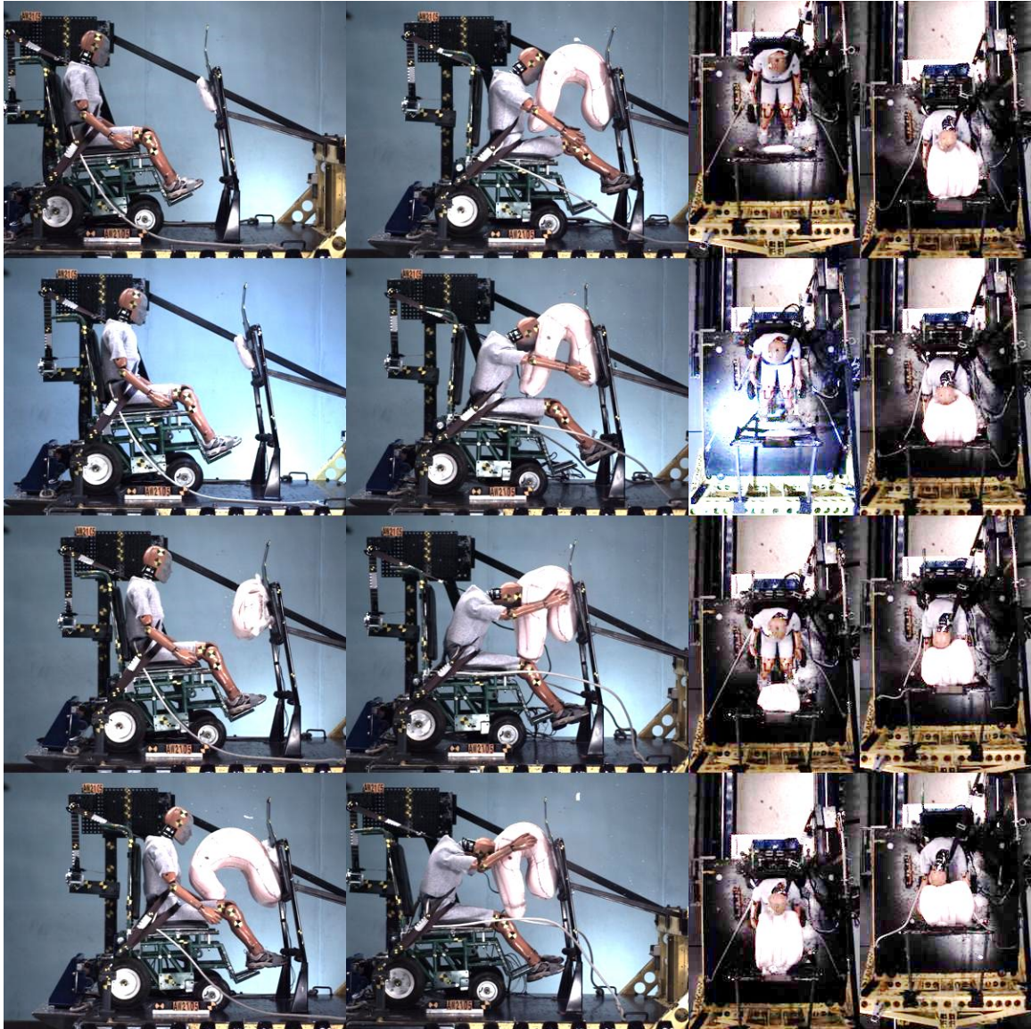
Figure C-5. Right side and overhead camera views every 20 ms for test AW2105
