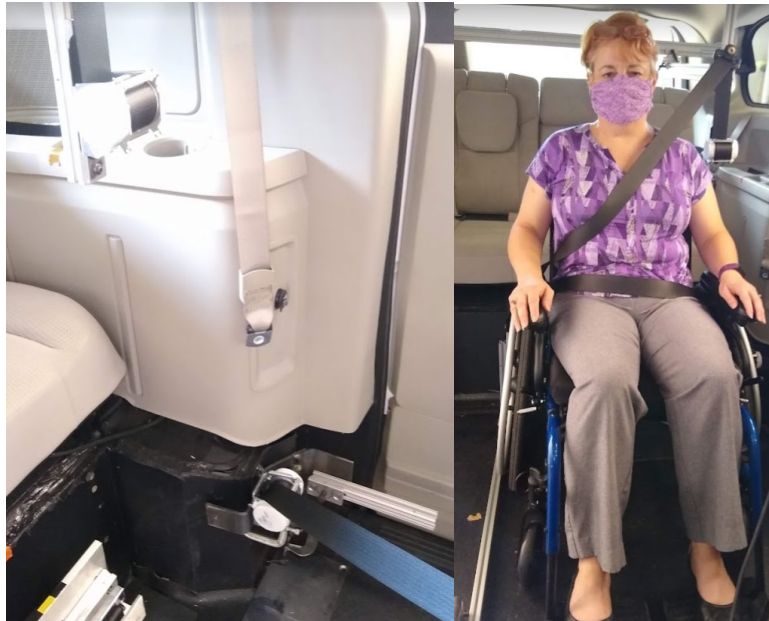
Figure E-1. Seat belt with dual retractors installed (left) and providing snug belt tension on pilot volunteer (right)
