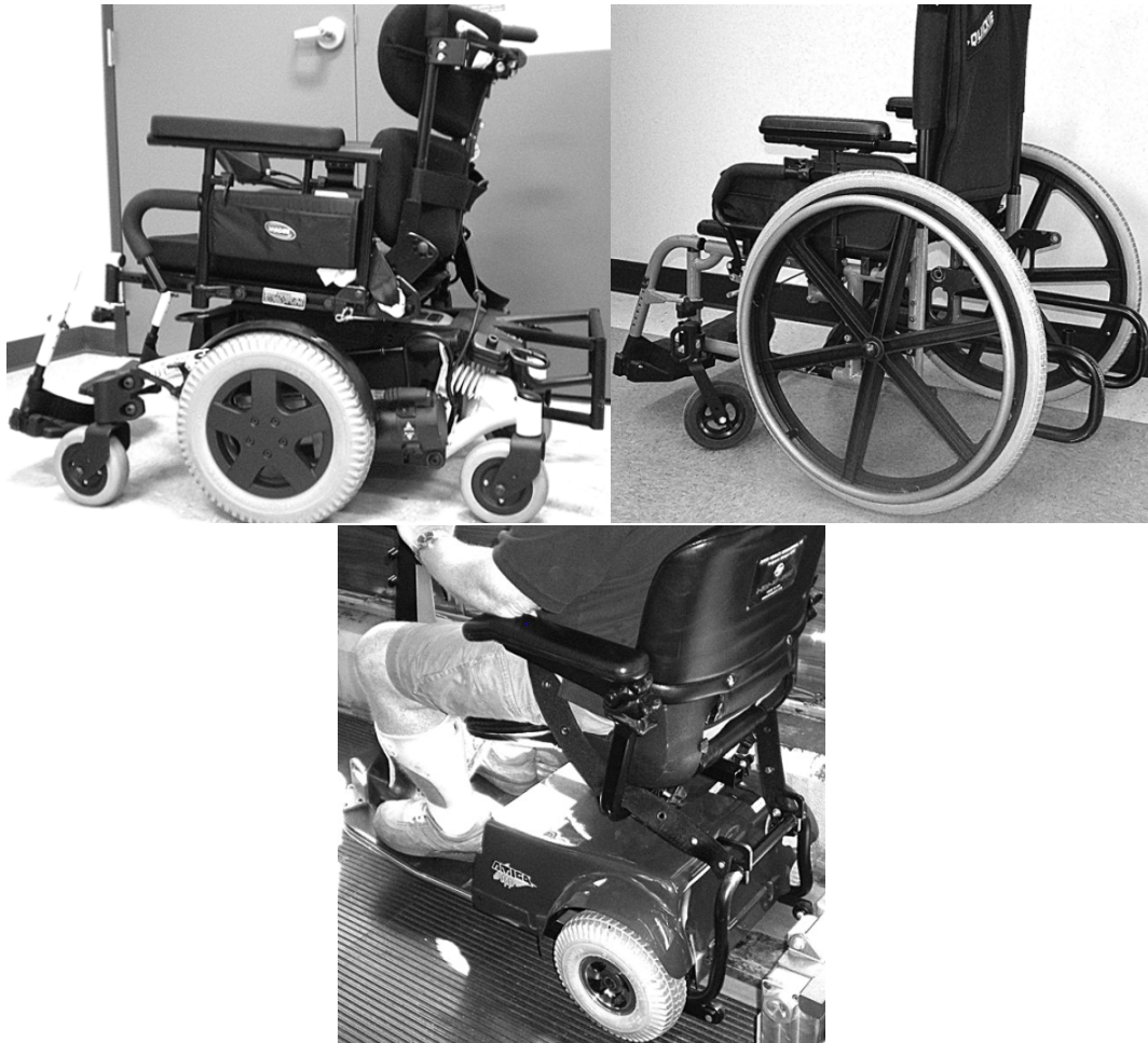
Figure 6. A power wheelchair (upper left), manual wheelchair (upper right), and scooter (lower center) equipped with UDIG-compatible hardware
