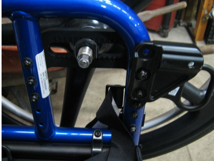
Figure 67. Location on manual wheelchair (pictured upside down) to attach UDIG-compliant attachments
