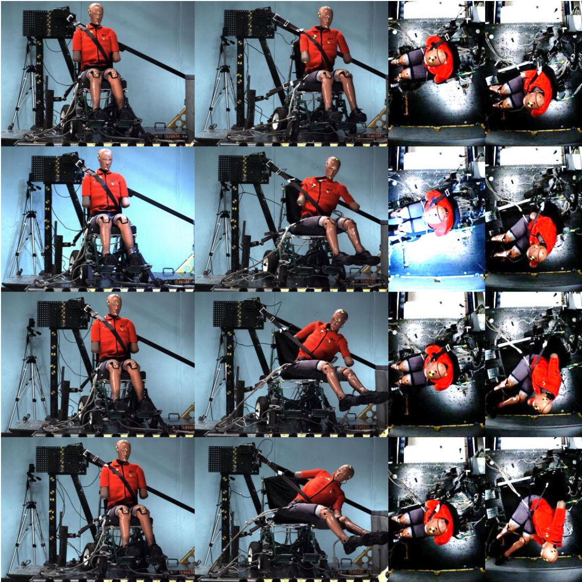
Figure C-12. Right side and oblique camera views every 20 ms for test AW2011, baseline with 4-point strap tiedown
